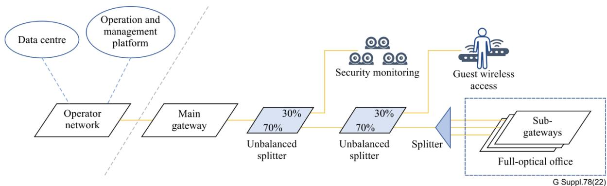
**Figure 7-12 – Applying an unbalanced optical splitter in a workshop scenario**
