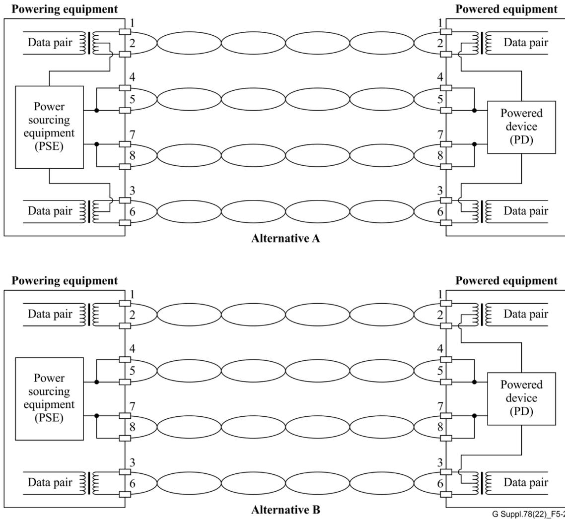
**Figure 5-2 – 10BASE-T/100BASE-TX 2-pair endpoint PSE location overview [IEEE 802.3bt]**
