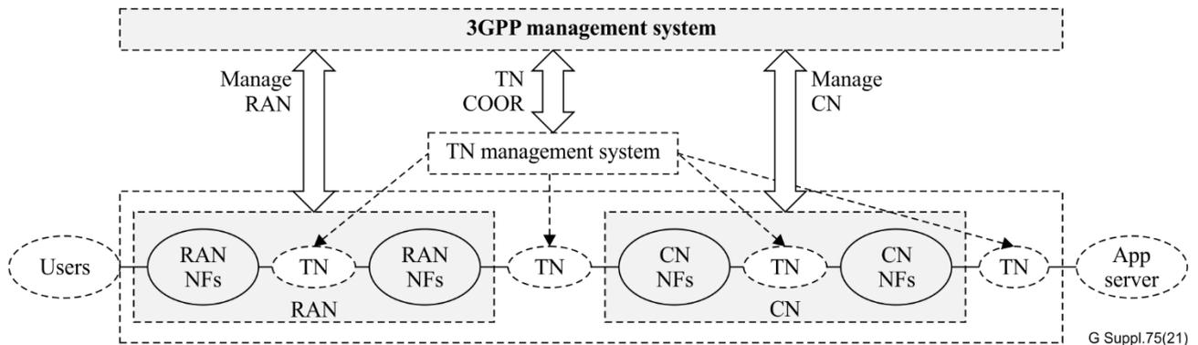
**Figure 20 – Example of coordination between 3GPP and TN management systems [b-3GPP TS 28.530]**
