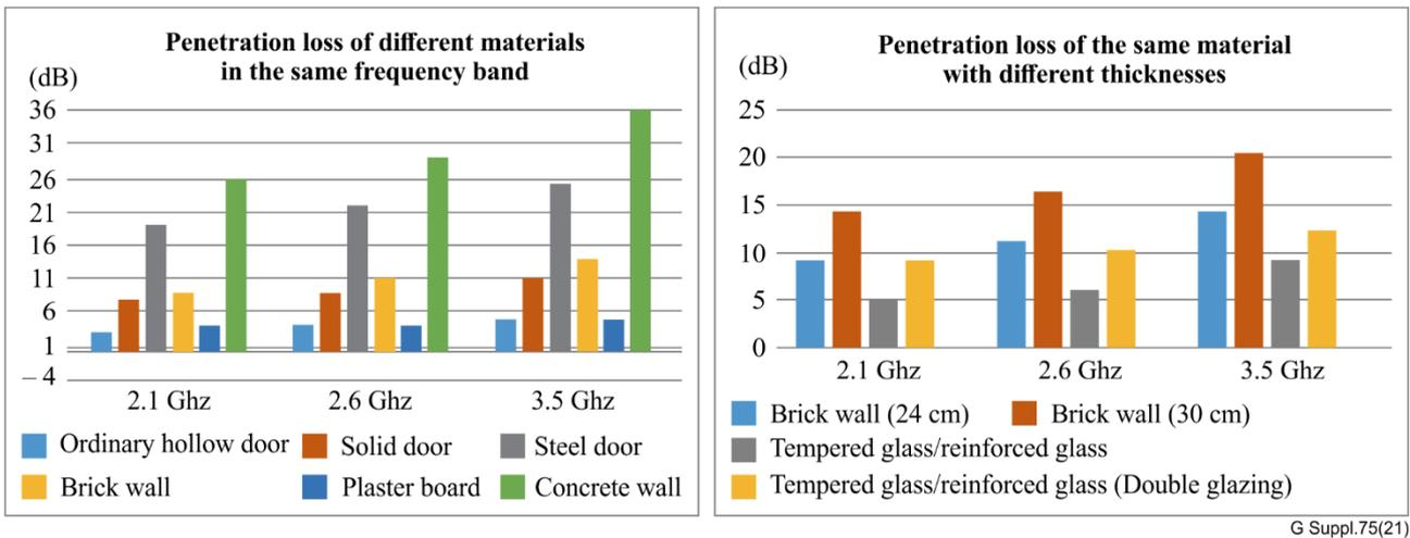
**Figure 9 – The penetration loss of wireless signals corresponding to different materials/thicknesses**
