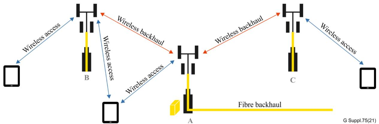
**Figure 31 – Schematic diagram of IAB**
