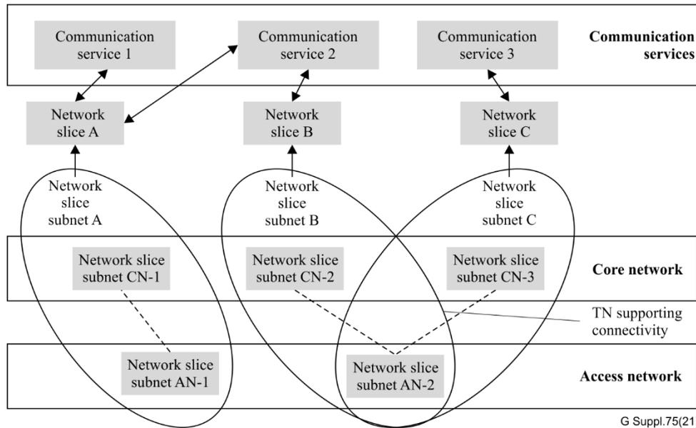
**Figure 18 – A variety of communication services provided by multiple network slices[b-3GPP TS 28.530]**
