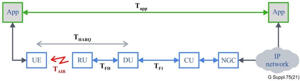
**Figure 12 – Requirements for latency (delay)**
