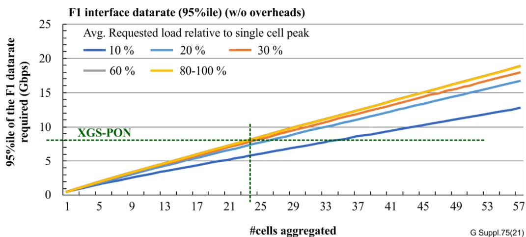
**Figure 25 – F1 midhaul area traffic capacity with 10G TDM-PON**
