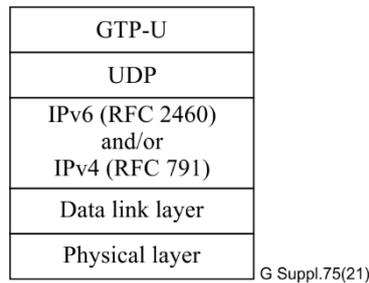
**Figure 22 – Transport network layer over F1**
