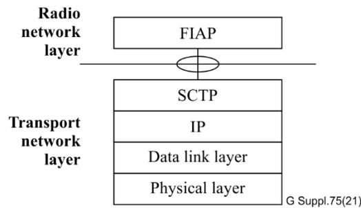
**Figure 23 – F1-C signalling bearer**
