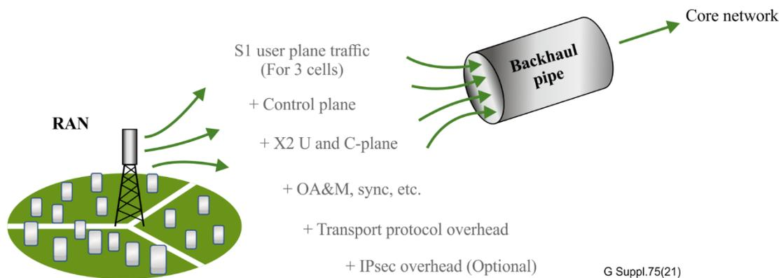
**Figure 10 – Components of backhaul traffic [b-NGMN LTE BH]**
