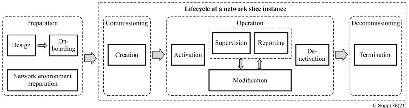
**Figure 19 – Management aspects of network slicing [b-3GPP TS 28.530]**
