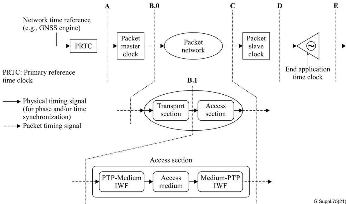
**Figure 28 – Models for budgeting in a chain of xPON devices per Appendix IX in [b-ITU-T G.8271.1]**
