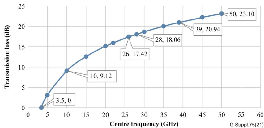
**Figure 36 – Transmission loss of different centre frequencies (compared with 3.5GHz) [b-CU mmW WP]**
