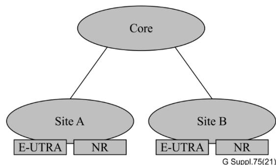
**Figure 33 – Co-sited deployment with E-UTRA (Figure 5.3-1 of [b-3GPP TR 38.801])**
