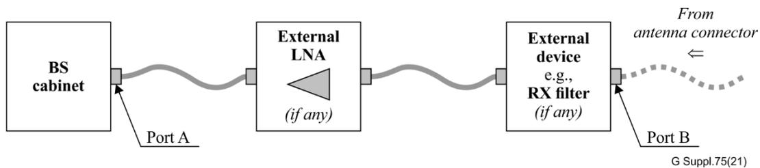
**Figure 5 – BS type 1-C receiver interface [b-3GPP TS 38.104]**
