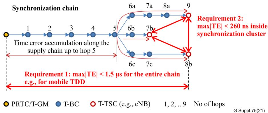
**Figure 16 – Illustration of relative time error**
