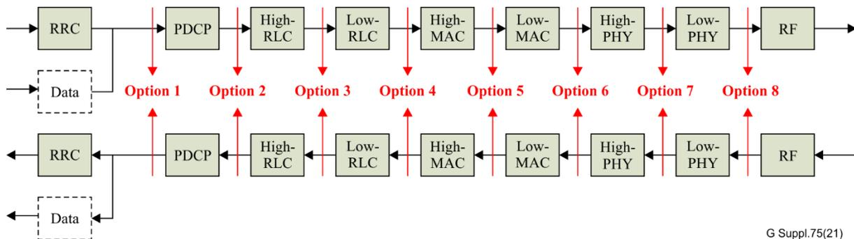
**Figure 1 – Function split between central and distributed unit [b-3GPP TR 38.801]**
