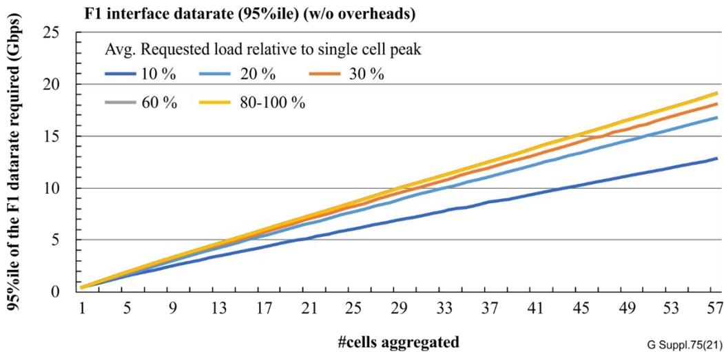
**Figure 11 – F1 midhaul area traffic capacity simulation based on 5G NR (3GPP 3D-UMa)**
