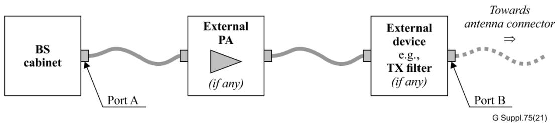
**Figure 4 – BS type 1-C transmitter interface [b-3GPP TS 38.104]**
