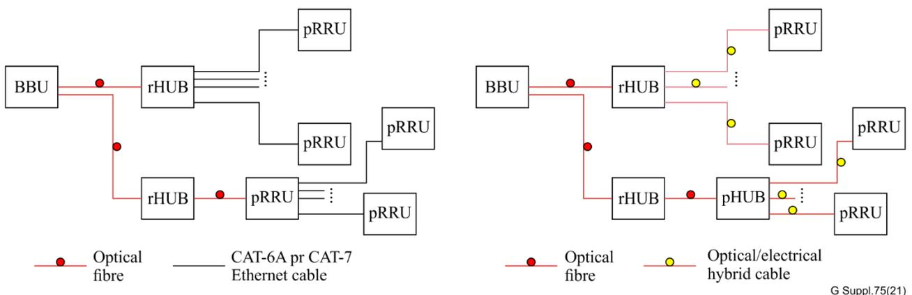
**Figure 30 – BBU (DU) + rHUB + pRRU Architecture**
