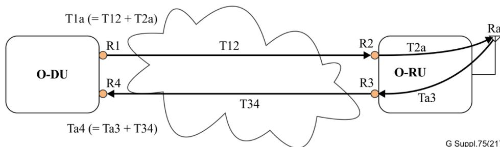
**Figure 13 – Definition of reference points for delay management (i.e., Figure B-1 in [b-O-RAN CUS])**
