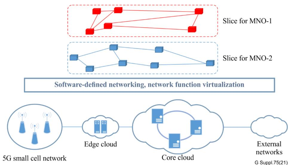
**Figure 29 – Example conceptualization of network slicing for small cell sharing (i.e., Figure 23 in [b-SCF500])**
