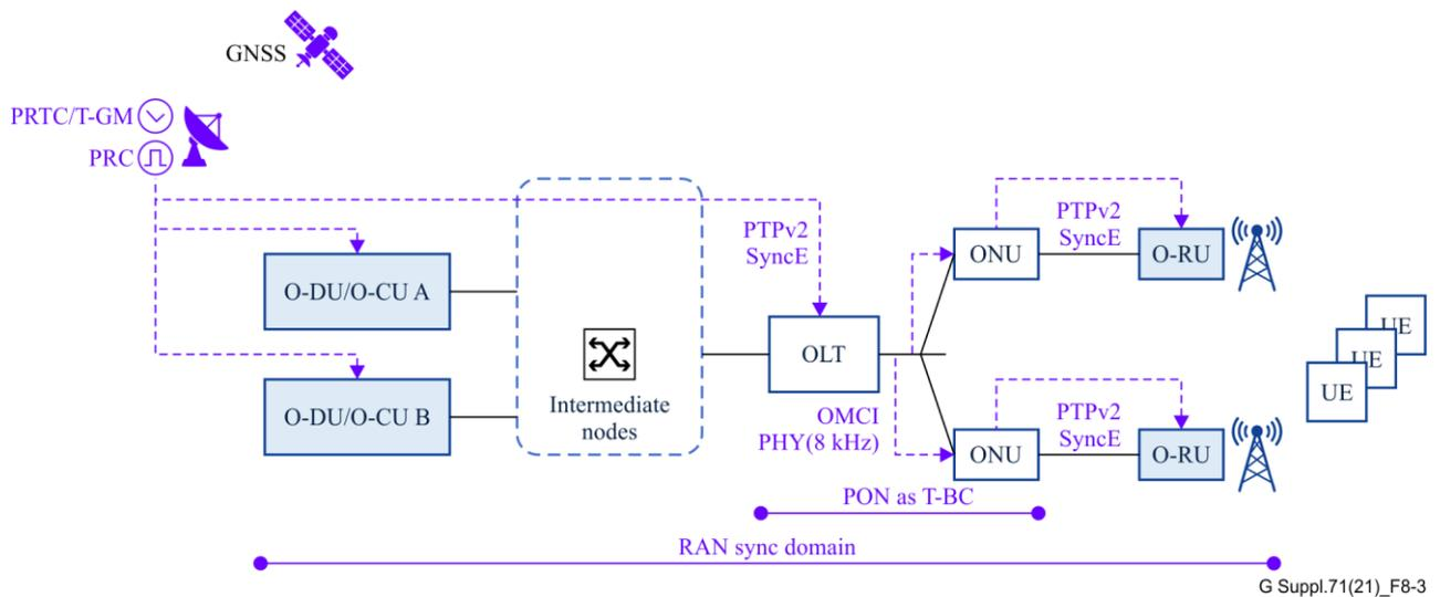
**Figure 8-3 – Access to common time of day by synchronizing transport domain to the RAN domain**
