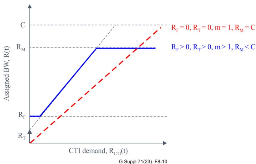
**Figure 8-10 – Effect of Co DBA traffic descriptor parameters**
