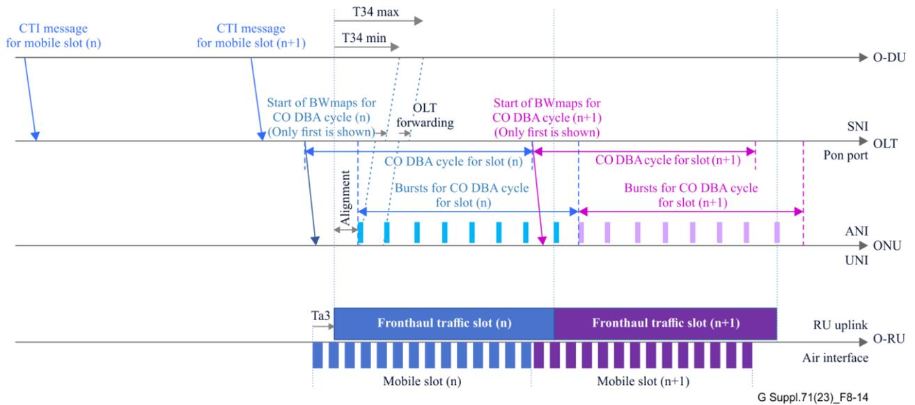
**Figure 8-14 – Alignment of CO DBA cycles with mobile slot boundaries at O-RU uplink**
