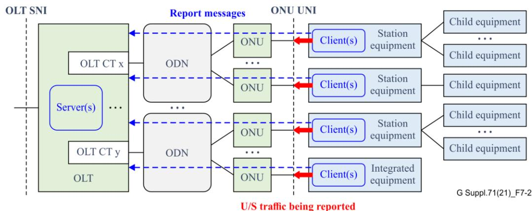
**Figure 7-2 – CO DBA by exchanging information with external entity subtended by ONU**
