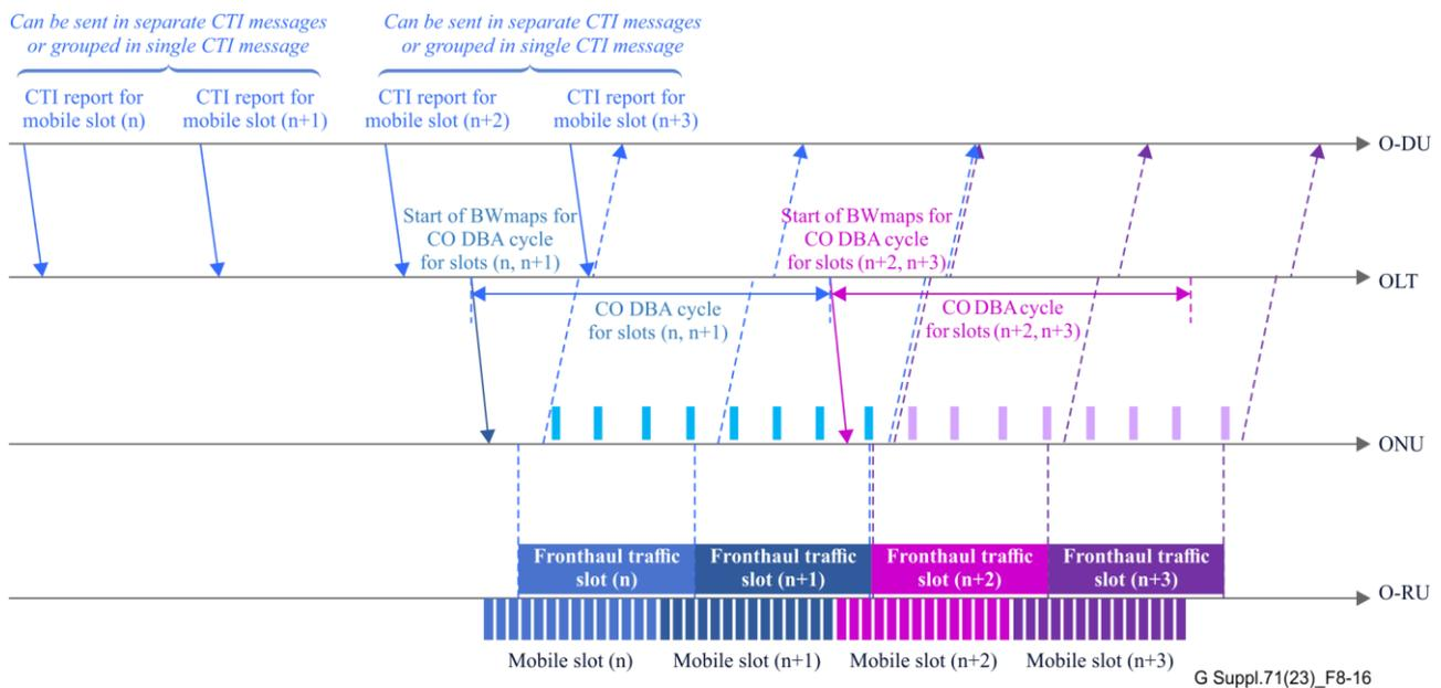
**Figure 8-16 – Multiple reported time intervals per CO DBA cycle**
