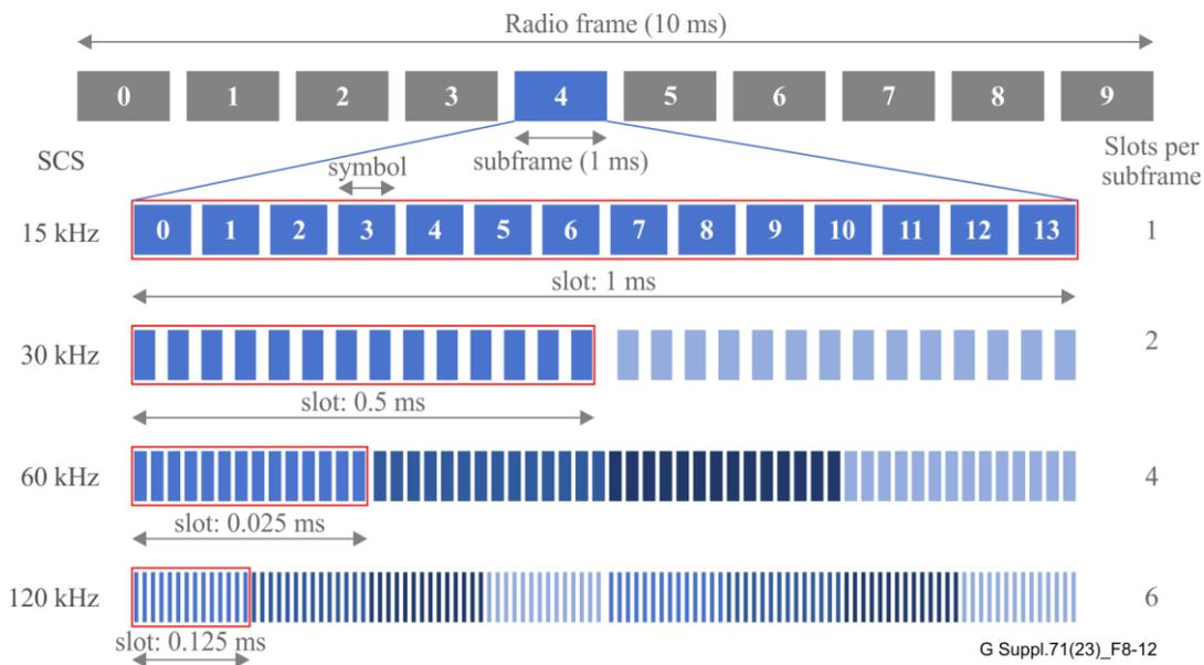
**Figure 8-12 – Time structures in RAN (sub-6 GHz) [b-NGMN Alliance]**
