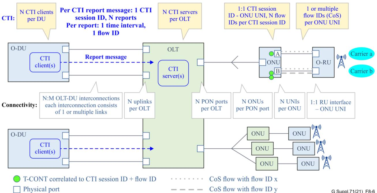
**Figure 8-6 – Interconnections, CTI clients and CTI servers, identifiers (every instance of "N" and "M" represents an independent number larger or equal to one)**
