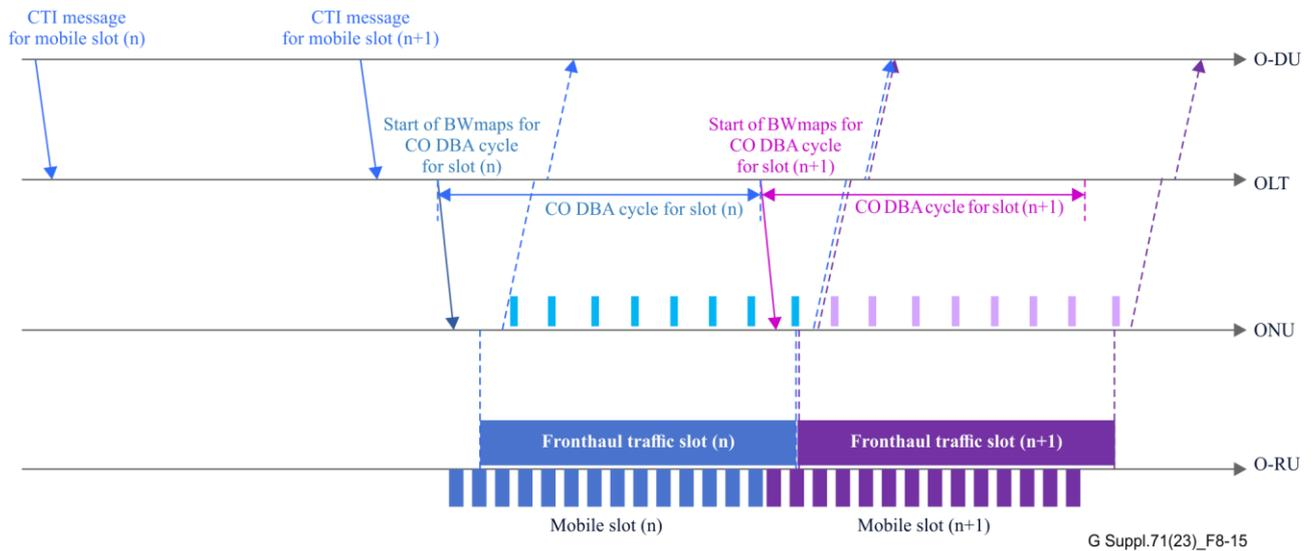
**Figure 8-15 – 1 CO DBA cycle per reported time interval**
