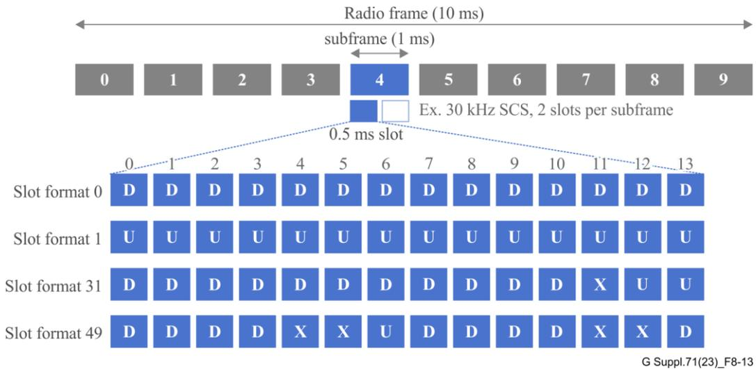
**Figure 8-13 – Dynamic slot configurations in 5G TDD: D – downstream symbol; U – upstream symbol; X – Flexible symbol: U, D or guard period**
