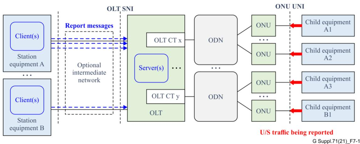
**Figure 7-1 – CO DBA by exchanging information with external entity north of OLT**
