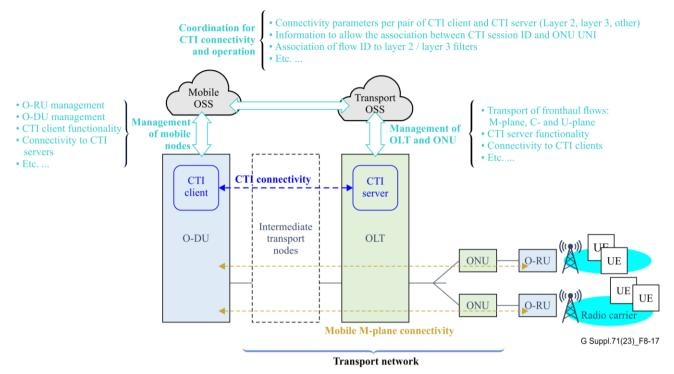
NOTE - M-plane connectivity between O-DU and O-RU is also depicted but is fully separate from CTI and does not replace the CTI connectivity between O-DU and OLT
