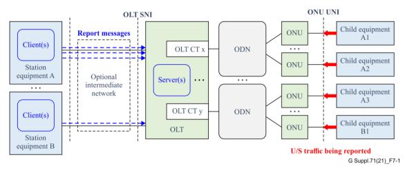
Figure 7-1 – CO DBA by exchanging information with external entity north of OLT
