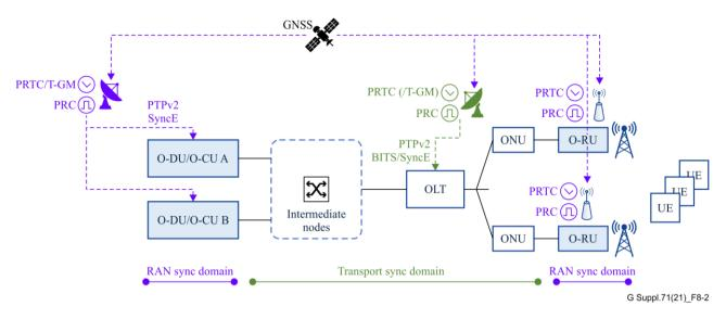
Figure 8-2 – Access to common time of day by separate GNSS inputs (no explicit synchronization between RAN and transport domains)
