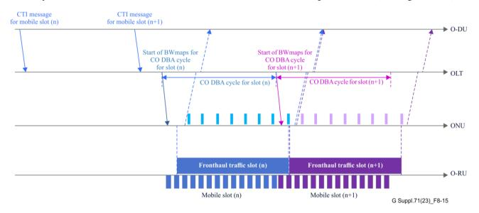
Figure 8-15 – 1 CO DBA cycle per reported time interval
