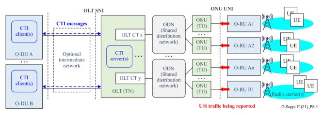
Figure 8-1 – Transport of mobile fronthaul with CTI
