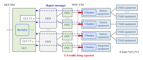
Figure 7-2 – CO DBA by exchanging information with external entity subtended by ONU
