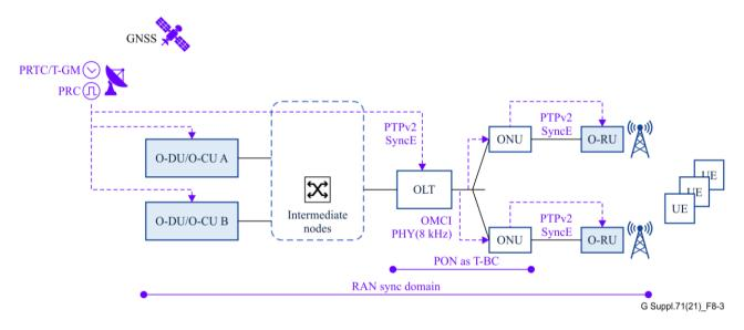
Figure 8-3 – Access to common time of day by synchronizing transport domain to the RAN domain
