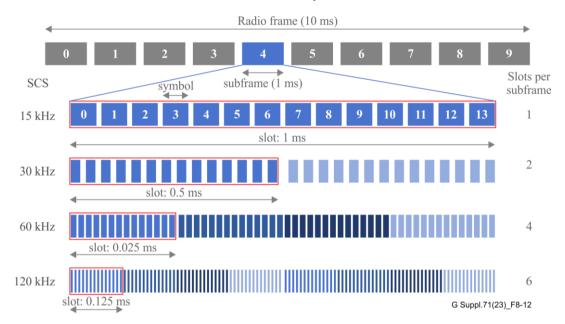
Figure 8-12 – Time structures in RAN (sub-6 GHz) [b-NGMN Alliance]
