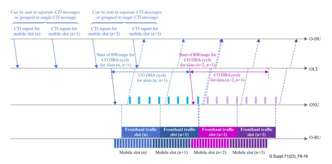
Figure 8-16 – Multiple reported time intervals per CO DBA cycle
