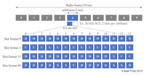
Figure 8-13 – Dynamic slot configurations in 5G TDD: D – downstream symbol; U – upstream symbol; X – Flexible symbol: U, D or guard period
