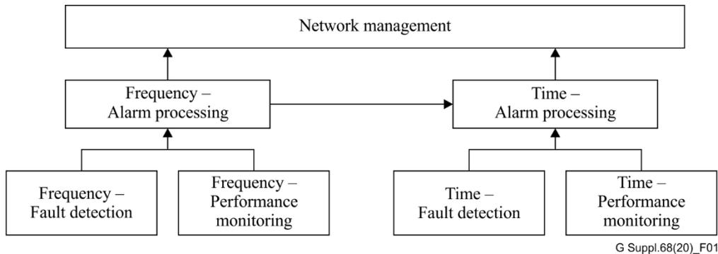
**Figure 1 – Synchronization OAM functional diagram**
