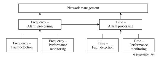
Figure 1 – Synchronization OAM functional diagram
