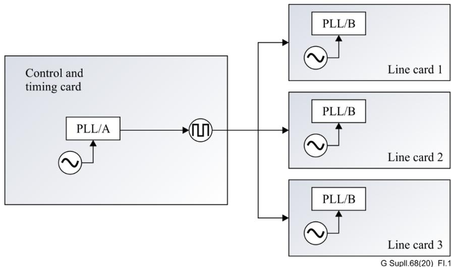
**Figure I.1 – Clock flow and detection within chassis system**
