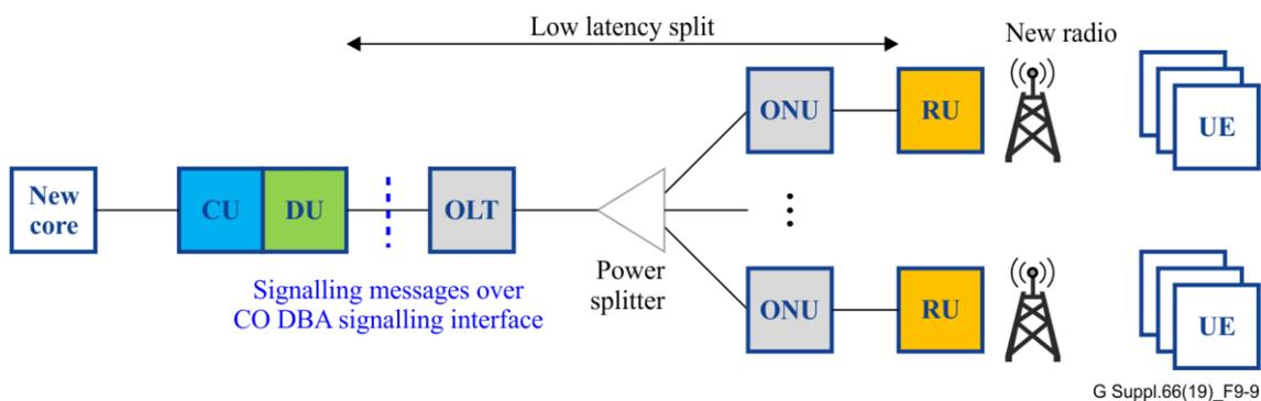
**Figure 9-9 – CO DBA signalling interface for mobile fronthaul**
