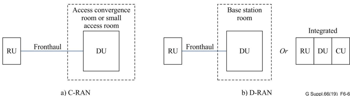
**Figure 6-6 – RAN deployment scenario schematic diagram**
