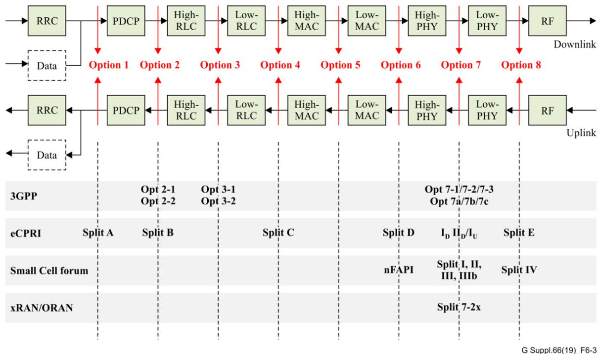
**Figure 6-3 – Mapping different split points to the 3GPP model in 3GPP [3GPP TR 38.801], CPRI group [eCPRI], SCF [SCF] and O-RAN [ORAN-FH]**
