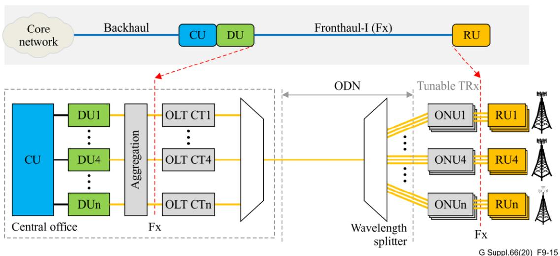
**Figure 9-15 – An example of WDM-PON implementation for Fx fronthaul interface**
