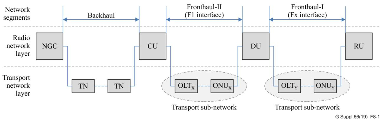
**Figure 8-1 – Concept of layered structure showing RNL (CU, DU, RU) and TNL (OLT, ONU). TN: Transport network [IEEE 1914.1]**
