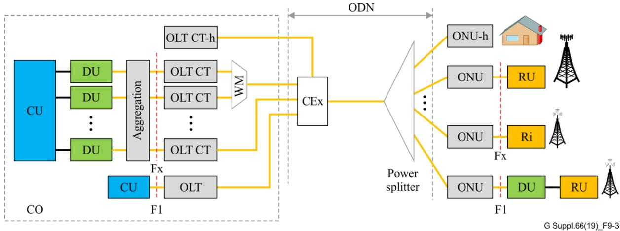
**Figure 9-3 – High layer and low layer split fronthaul based for legacy PON with WDM overlay**
