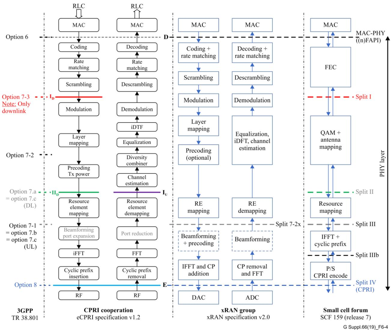
**Figure 6-4 – Detailed comparison and mapping of option 7 sub-splits**
