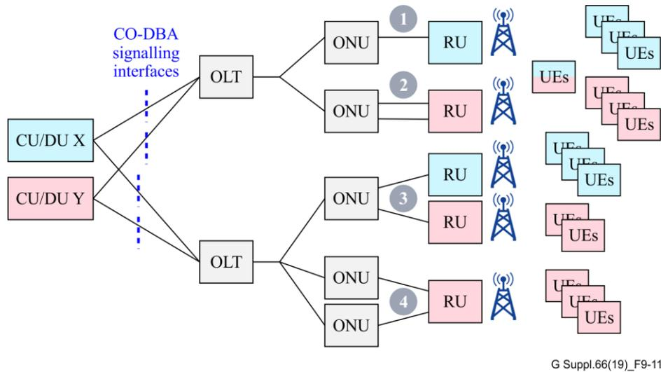
**Figure 9-11 – Architecture variants for CO DBA**
