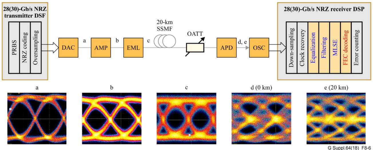
**Figure 8-6 – Schematic of the 28-Gbit/s NRZ-DSP equalization experiment set-up.
