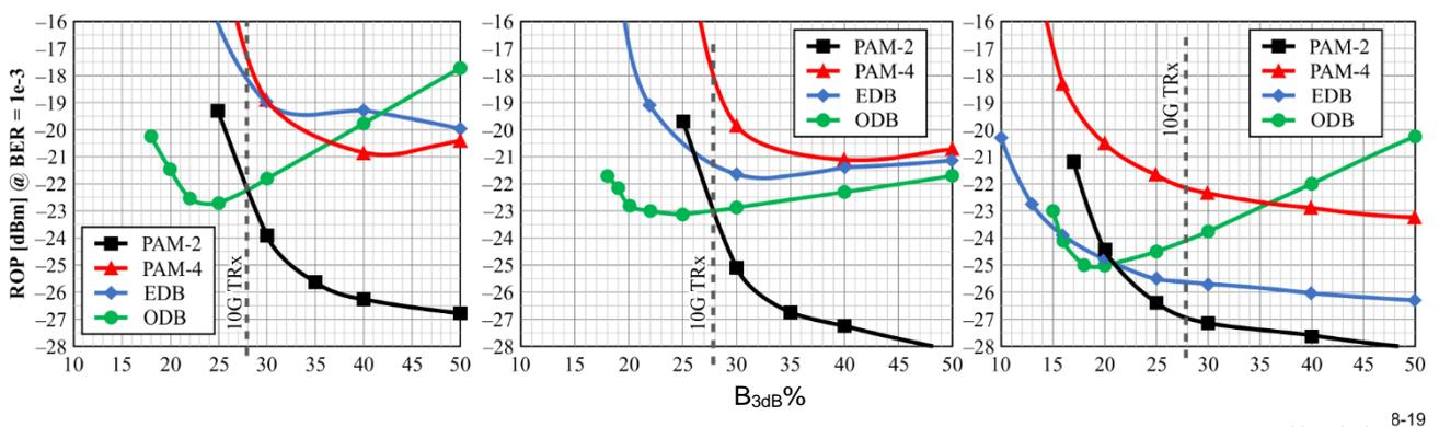
**Figure 8-19 – back-to-back performance, ER = ∞, a) without equalizer, fixed threshold; b) without equalizer, optimized threshold; c) with equalizer, optimized threshold**
