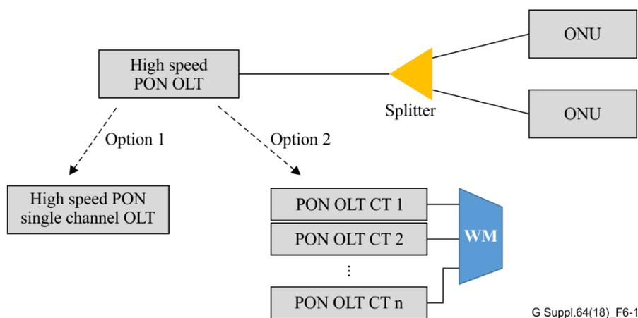
**Figure 6-1 – High speed PON architecture**
