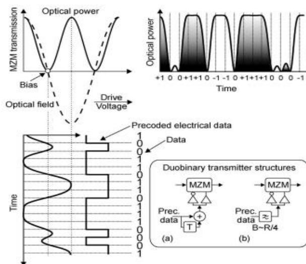
**Figure 8-12 – ODB modulation principle**
