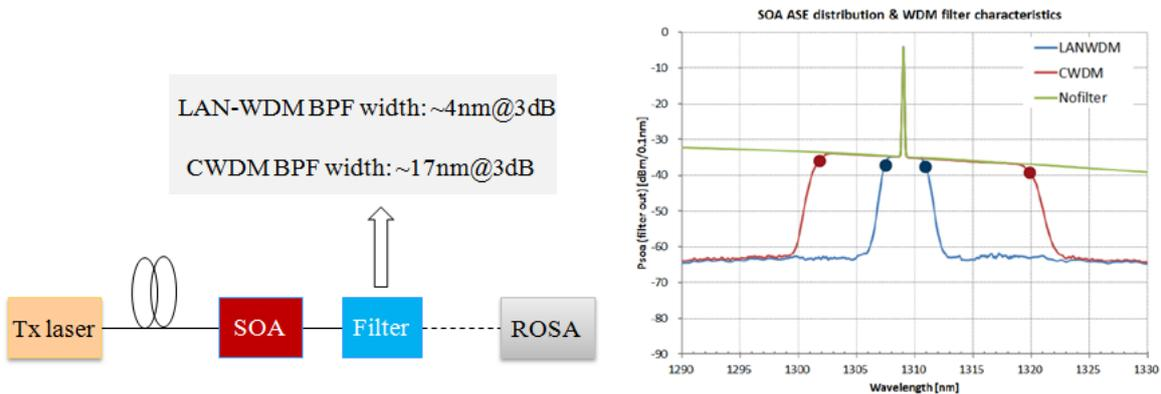
**Figure 8-33 – SOA spectrum after narrow band pass filters**
