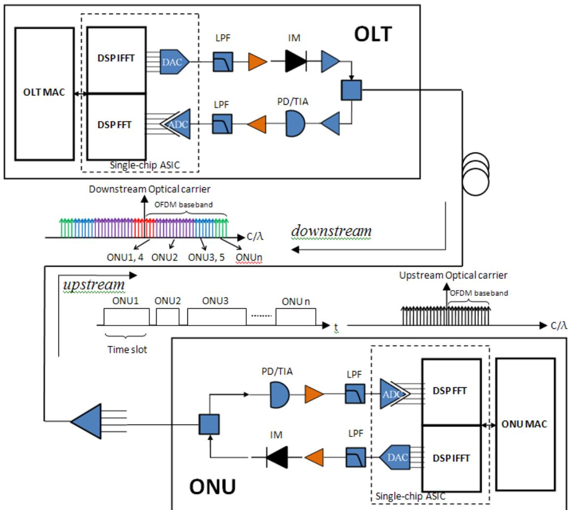
**Figure 8-17 – Example architecture of DMT modulation**
