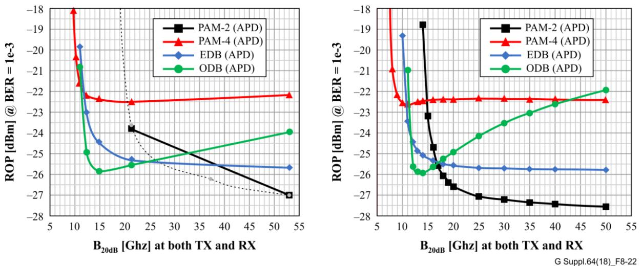
Figure 8-22 – Effect of TX/RX frequency response, comparison of Butterworth (left) and S-Gaussian (right) filter models, varying B<sub>20dB</sub>
