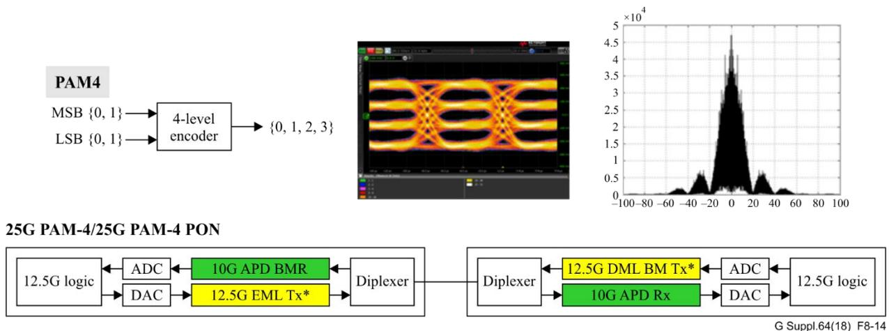
Figure 8-14 – Schematic of PAM4 modulation
