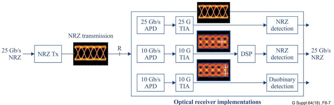
**Figure 8-7 – NRZ transmission and multiple receiver implementation options**
