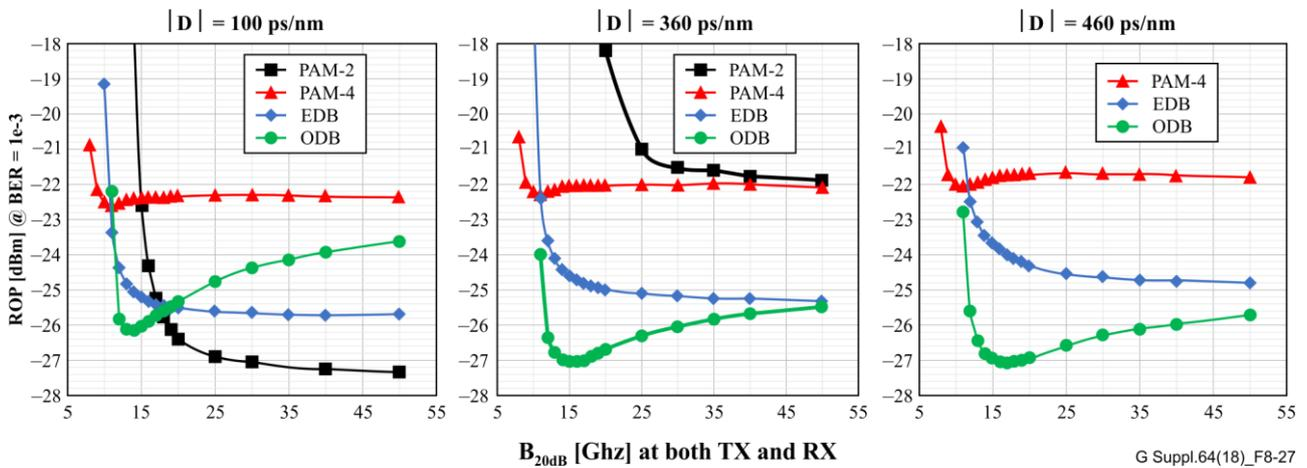
**Figure 8-27 – Effect of dispersion and TX/RX frequency response, S-Gaussian filter model, B<sub>3dB</sub>=7 GHz, varying B<sub>20dB</sub> and |D| (note: |D| values are not the same of Figure 8-25)**
