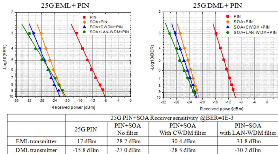
Figure 8-34 – 25 Gbit/s PIN+SOA receiver performance on EML and DML signal
