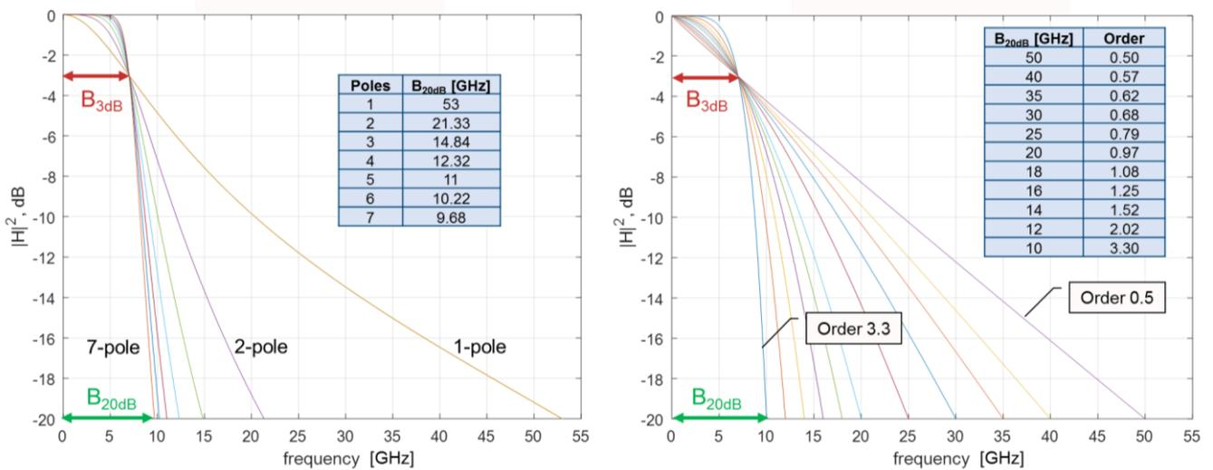
Figure 8-20 – 3 dB and 20 dB bandwidths for Butterworth (left) and S-Gaussian (right) filters
