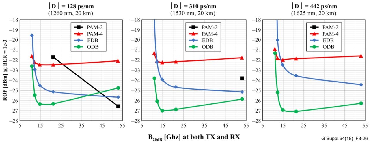
**Figure 8-26 – Effect of dispersion and TX/RX frequency response, Butterworth filter model, B<sub>3dB</sub>=7 GHz, varying B<sub>20dB</sub> and |D|**
