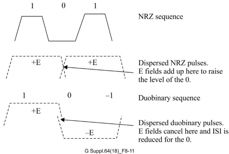
**Figure 8-11 – ODB interference offset to avoid ISI**
