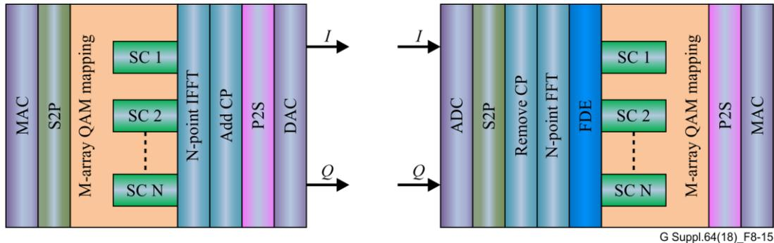
**Figure 8-15 – Basic OFDM system architecture**
