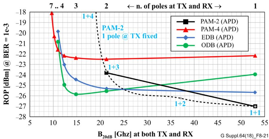
Figure 8-21 – Effect of TX/RX frequency response, Butterworth filter model, varying B<sub>20dB</sub> (number of poles); the dashed line represents the case with a single-pole TX and a varying number of poles at RX
