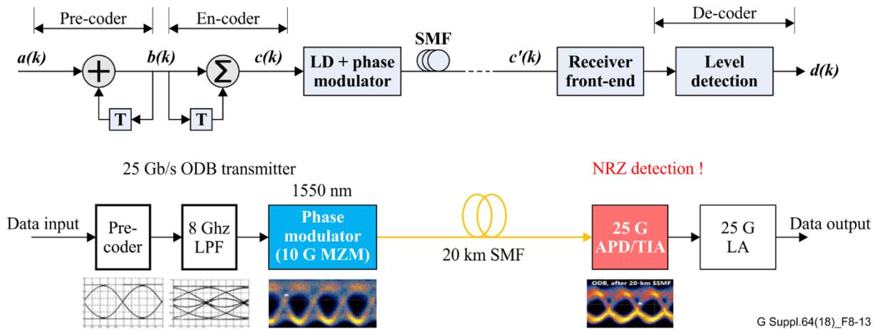
Figure 8-13 – Coding and decoding schematic diagram of 25 Gbit/s ODB
