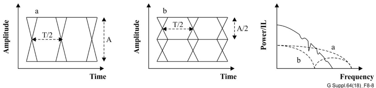
**Figure 8-8 – Schematic of NRZ waveform (left), EDB waveform (middle) and the corresponding power spectrum diagram (right)**
