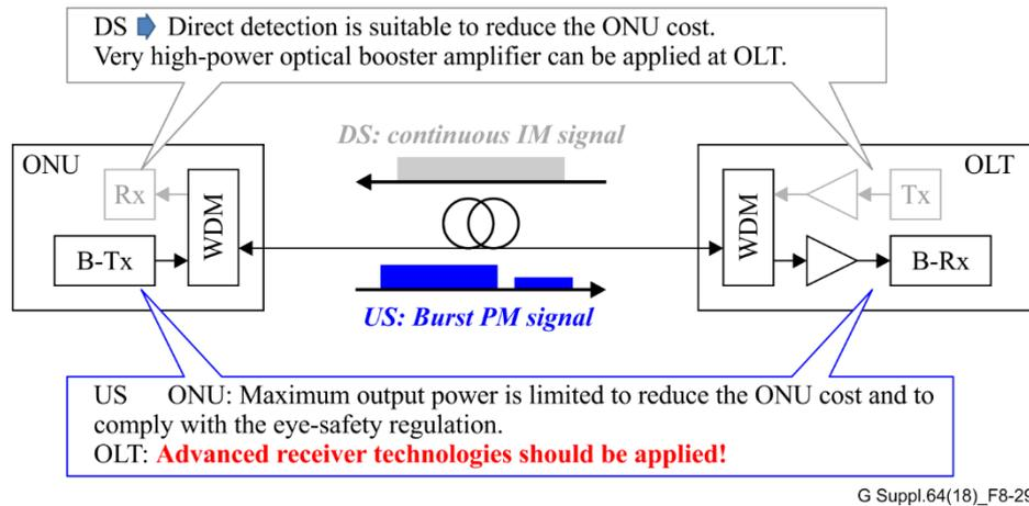
**Figure 8-29 – System configuration assumed in this study**
