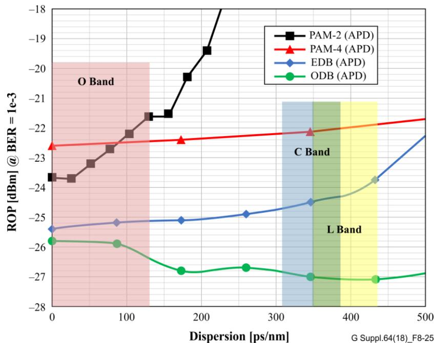
Figure 8-25 – Effect of chromatic dispersion, two-pole Butterworth TX/RX response,  $B_{3\text{dB}}=7 \text{ GHz}$
