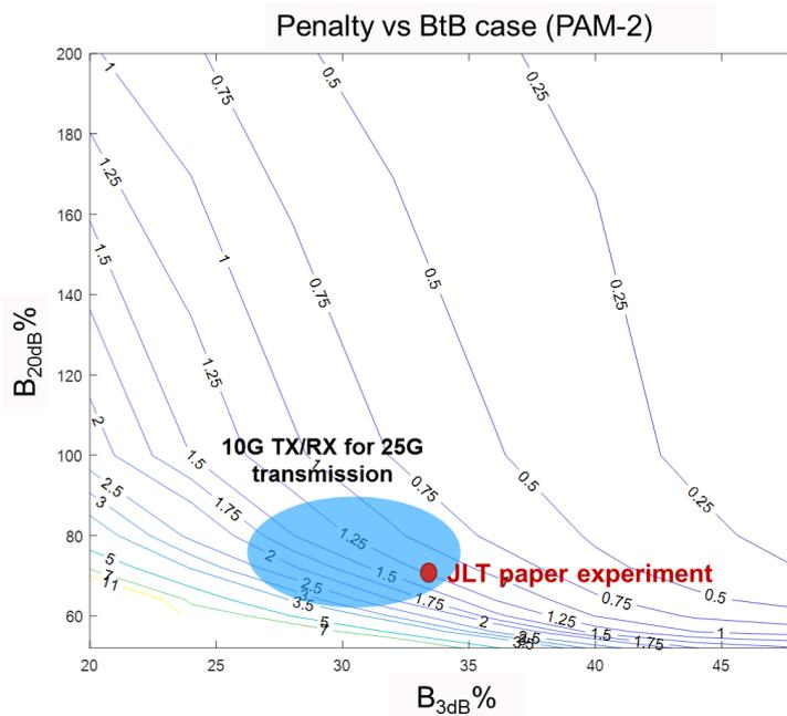
**Figure 8-23 – Penalty for PAM-2 transmission versus TX/RX 3dB and 20dB bandwidths; the red dot corresponds to the case analysed in the JLT paper**
