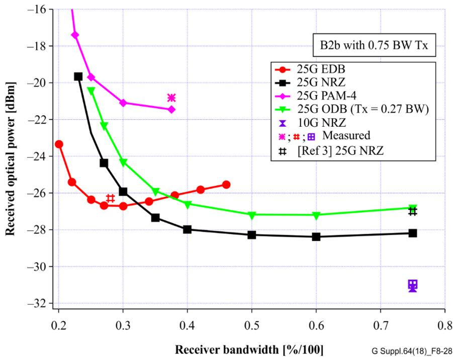
**Figure 8-28 – Back-to-back experiment results, ER = 13 dB (5.5 dB PAM-4). TX filter response –3 dB point at 0.75 x bit rate for NRZ and EDB, 0.27 x bitrate for ODB, 0.75 x baud rate (0.375 x bit rate) for PAM-4**
