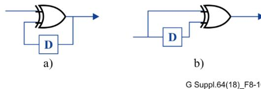
**Figure 8-10 – (a) Transmitter pre-coder (b) NRZ receiver decoder**
