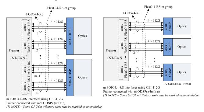
Figure 10-2c – Third example applications of FOIC4.4-RS interface
