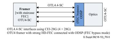
Figure 8-5 – Example application of OTL4.4-SC interface
