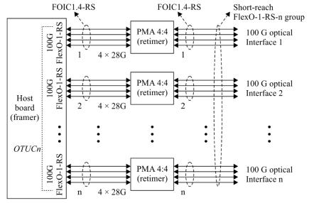
n FOIC1.4-RS interface using CEI-28G to n bonded 100G optical modules
