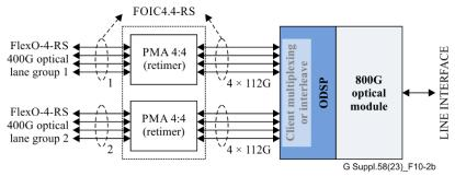
Single 800G optical module/ODSP witj 2 FOIC4.4-RS interfaces on host using 8 × CEI-112G connected with either an 800G 8-lane pluggable module or two 400G 4-lane pluggable modules
