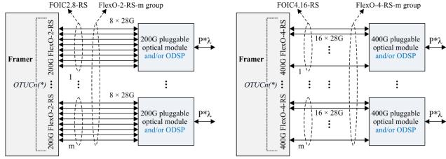
m FOIC2.8-RS (short-reach) interfaces using CEI-28G  $(2m \ge n)$  Framer connected with m pluggable modules and/or ODSPs (\*) NOTE – Some OPUCn tributary slots may be marked as unavailable
