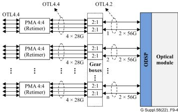
n OTL4.2 (and/or FOIC1.2-RS) interfaces using CEI-56G Framer connected with optical module/ODSP
