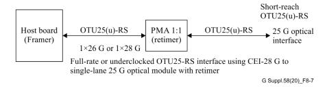
Figure 8-7 – Example application of single lane OTU25-RS and OTU25u-RS interfaces
