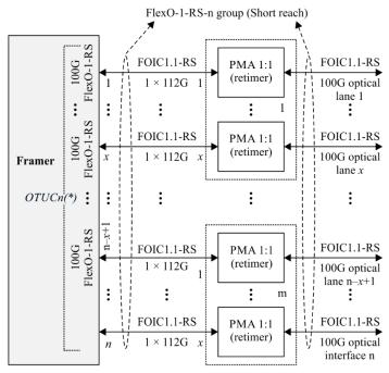
Framer with n FOIC1.1-RS interfaces connected through CEI-112G electrical lanes with m x00G pluggable modules with x\*100G optical lane each ( $n \le m \times x$ )
