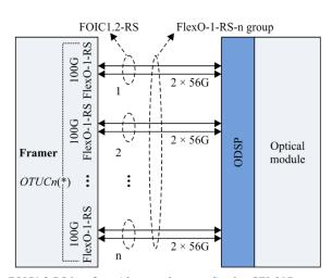
n FOIC1.2-RS interfaces (short-reach protocol) using CEI-56G Framer connected with single optical module/ODSP (\*) NOTE – Some OPUCn tributary slots may be marked as unavailable
