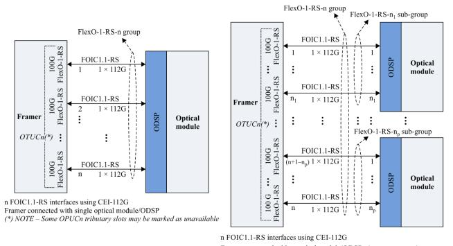
Framer connected with p optical module/ODSPs  $(n_1+n_2+..+n_p=n)$  (\*) NOTE – Some OPUCn tributary slots may be marked as unavailable G Suppl.58(23)\_F10-1a
