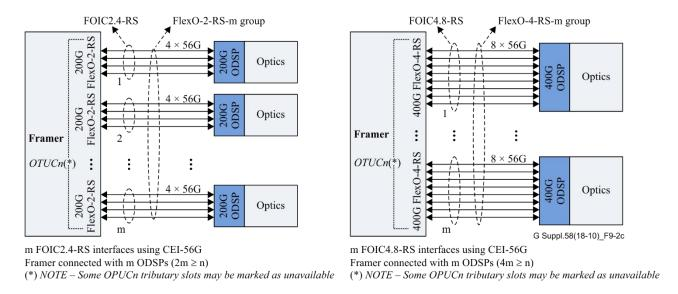
Figure 9-2c – Alternate application of FOIC2.4-RS and FOIC4.8-RS interfaces
