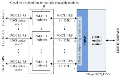
[x00G] optical module/ODSP with xFOIC1.1-RS interfaces on host using  $x \times \text{CEI-}112G$  connected with m pluggable modules (m  $\geq$  1) with one or multiple 100G optical lane each
