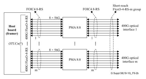
Figure 9-2b – FOIC4.8-RS interface main application example
