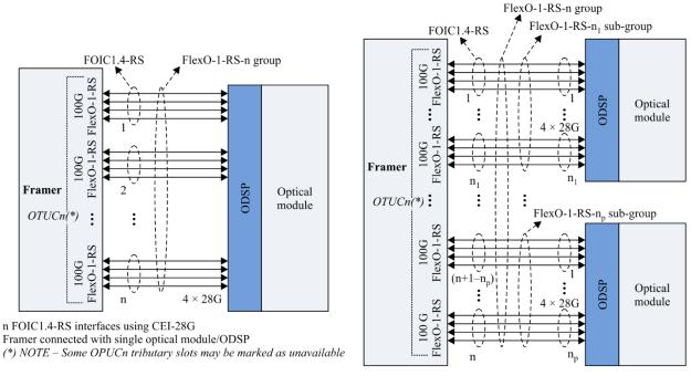
n FOIC1.4-RS interfaces using CEI-28G Framer connected with p optical module/ODSPs  $(n_1+n_2+..+n_p = n)$
