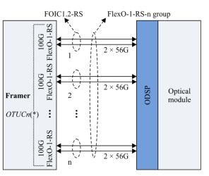
n FOIC1.2-RS interfaces (short-reach protocol) using CEI-56G Framer connected with single optical module/ODSP (\*) NOTE – Some OPUCn tributary slots may be marked as unavailable
