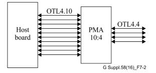
Figure 7-2 – Illustration of the original application of an OTL4.10 interface
