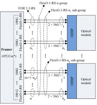
n FOIC1.2-RS interfaces (short-reach protocol) using CEI-56G Framer connected with p optical modules/ODSPs  $(n_1+n_2+...+n_p = n)$ (\*) *NOTE – Some OPUCn tributary slots may be marked as unavailable* G Suppl.58(18-10)\_F9-1
