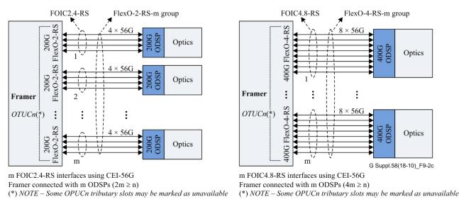
Figure 9-2c - Alternate application of FOIC2.4-RS and FOIC4.8-RS interfaces
