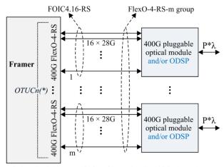
m FOIC4.16-RS (short-reach) interfaces using CEI-28G ( $4m \ge n$ ) Framer connected with m pluggable optics and/or ODSPs (\*) NOTE – Some OPUCn tributary slots may be marked as unavailable G Suppl.58(18-10)\_F8-4
