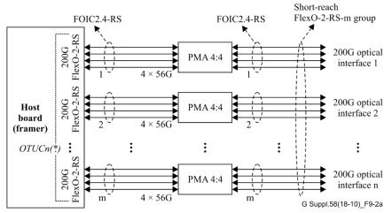
m FOIC2.4-RS short-reach interfaces using CEI-56G to m bonded 200G optical modules  $(2m \ge n)$ (\*) *NOTE* – *Some OPUCn tributary slots may be marked as unavailable; if* 2m = n, then each 200G *FlexO-2-RS carries two OTUC; else if* 2m > n, *some 200G FlexO-2-RS signal frames within the group only carry one OTUC in their first 100G FlexO instance (second 100G FlexO instance being unequipped)*
