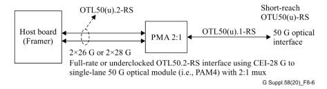
Figure 8-6 – Example application of OTL50.2-RS and OTL50u.2-RS interfaces
