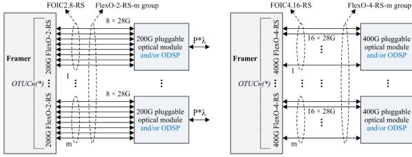
m FOIC2.8-RS (short-reach) interfaces using CEI-28G ( $2m \ge n$ ) Framer connected with m pluggable modules and/or ODSPs (\*) NOTE – Some OPUCn tributary slots may be marked as unavailable
