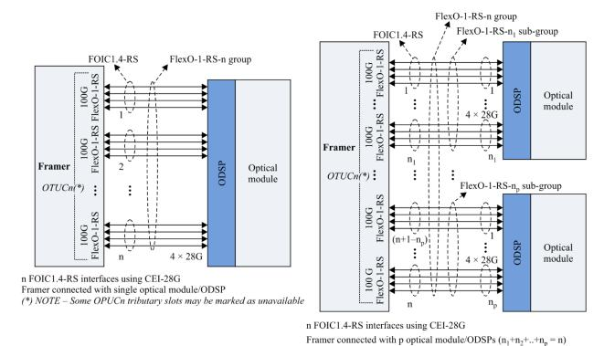
Figure 8-3b – Alternate application of a FOIC1.4-RS interface
