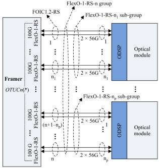
n FOIC1.2-RS interfaces (short-reach protocol) using CEI-56G Framer connected with p optical modules/ODSPs ( $n_1+n_2+...+n_p=n$ ) (\*) NOTE – Some OPUCn tributary slots may be marked as unavailable G Suppl.58(18-10)\_F9-1
