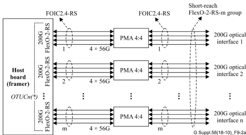
$m$  FOIC2.4-RS short-reach interfaces using CEI-56G to  $m$  bonded 200G optical modules ( $2m \geq n$ )
