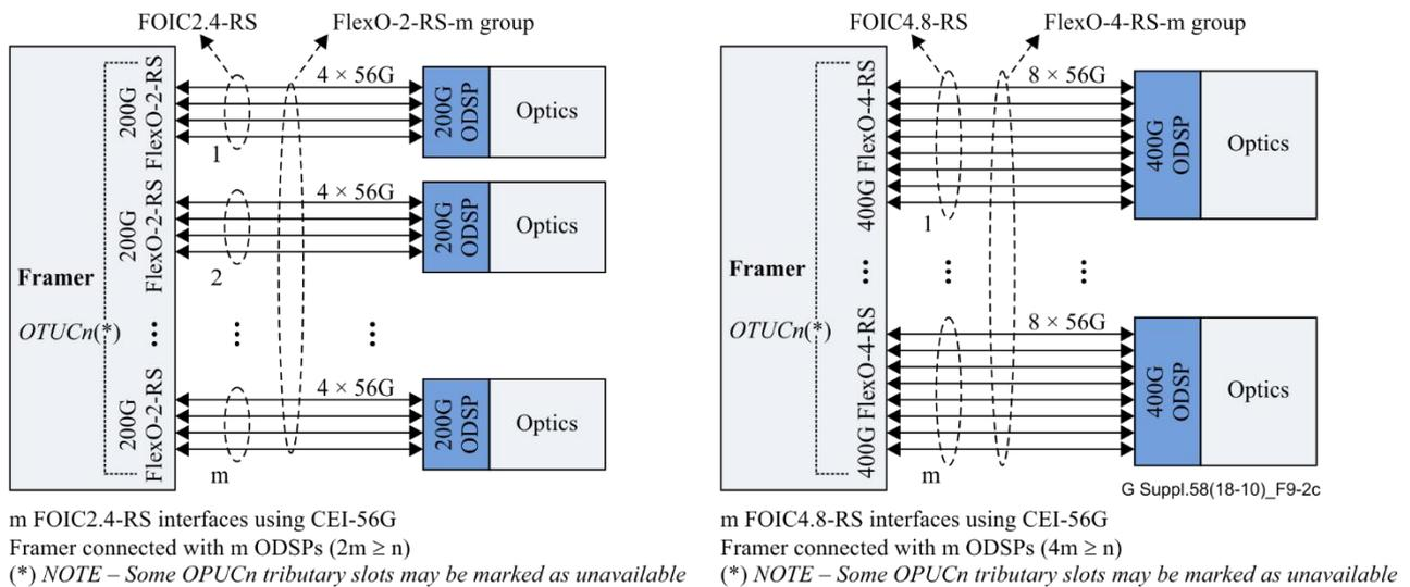
**Figure 9-2c – Alternate application of FOIC2.4-RS and FOIC4.8-RS interfaces**
