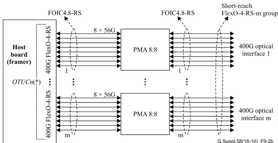
**Figure 9-2b – FOIC4.8-RS interface main application example**
