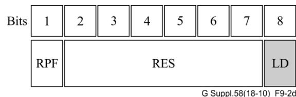
**Figure 9-2d – Optional Rx line pre-FEC local degrade (LD) status bit location in 1<sup>st</sup> instance of FlexO OH STAT field (Rx ODSP to framer direction)**
