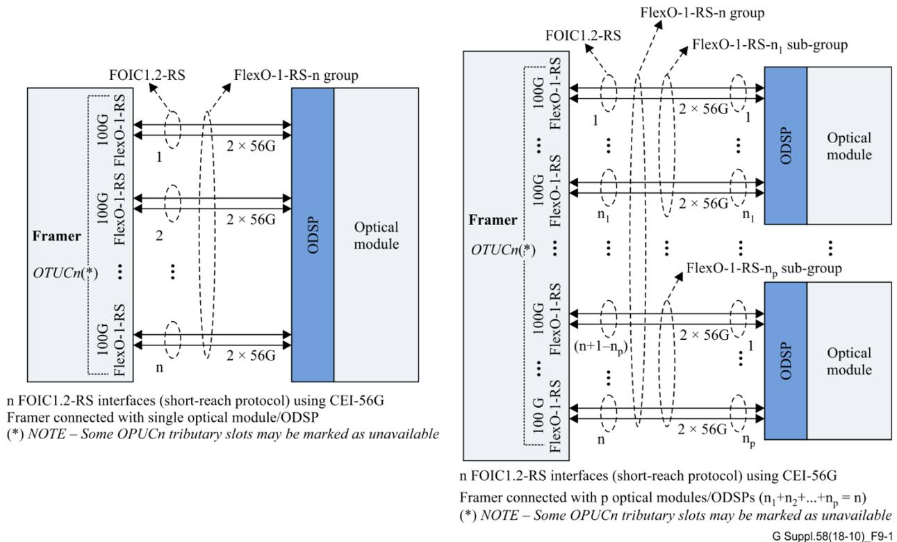
**Figure 9-1 – Example applications of a FOIC1.2-RS interface**
