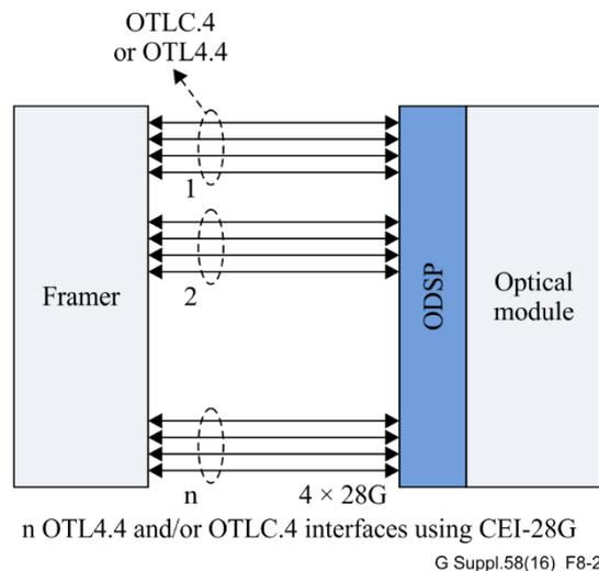
**Figure 8-2 – Example applications of an OTL4.4/OTLC.4 interface**
