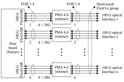
n FOIC1.4 short-reach interface using CEI-28G to n bonded 100G optical modules G Suppl.58(17)\_F8-3a
