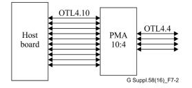
Figure 7-2 – Illustration of the original application of an OTL4.10 interface
