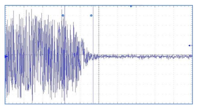
Figure 8 – Example trace of gradual LOS upon fibre cut
