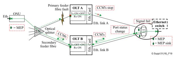
Figure 19 – Ethernet linear protection at a glance
