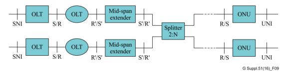
Figure 9 – Extended Type B protection architecture with two independent RE units
