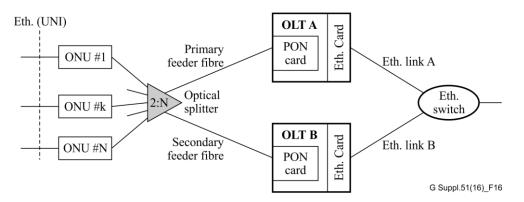
Figure 16 – General physical configuration of a dual-parented type B PON protection
