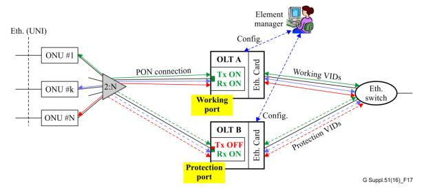
Figure 17 – Initial PON system connection configuration and protected Ethernet connections with two associated VLAN identifiers (VIDs)
