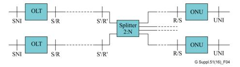
**Figure 4 – Dual-parented Type B protection**
