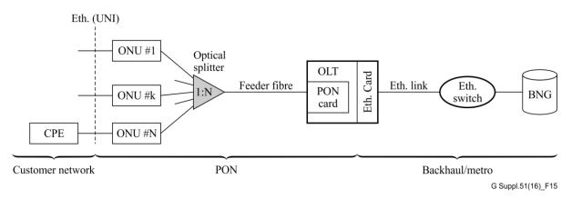
Figure 15 – Elements of a connection between a CPE and BNG over a PON and backhaul
