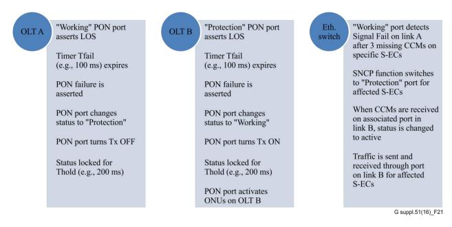
Figure 21 – Step by step description of the solution
