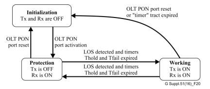
Figure 20 – OLT PON port state machine diagram
