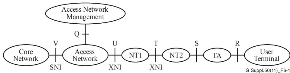
**Figure 6-1 – A reference configuration for a generic ITU-T G.99x system**
