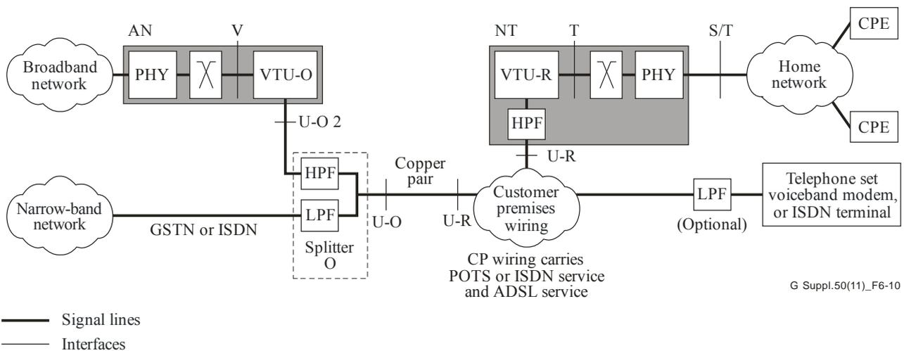
**Figure 6-10 – Generic application reference model for splitterless remote deployment**
