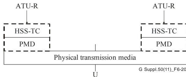
**Figure 6-20 – User plane protocol reference architecture for ITU-T G.994.1**
