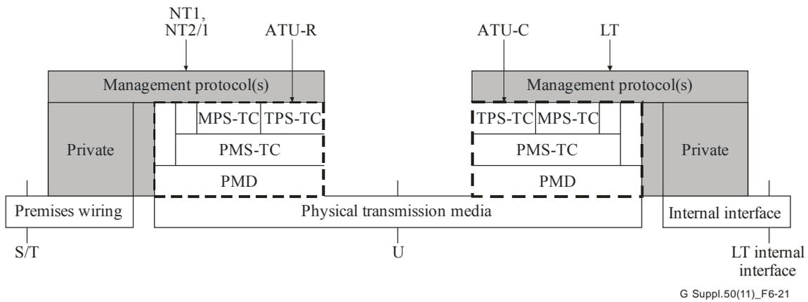
**Figure 6-21 – Management plane protocol reference architecture for ITU-T G.99x Recommendations**
