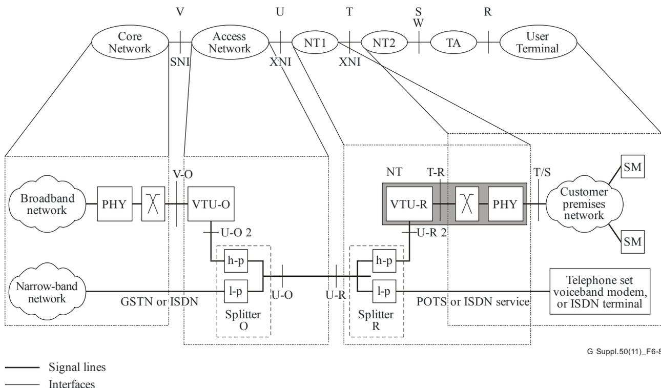
**Figure 6-8 – ITU-T G.993.1 system reference model and its alignment with the generic reference configuration**
