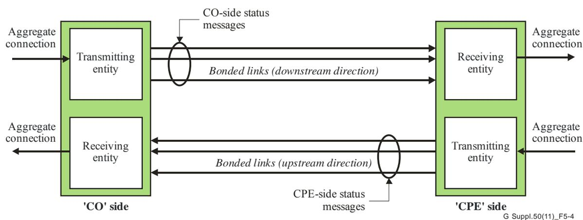
**Figure 5-4 – Status message flow. Each transmission direction is treated independently**
