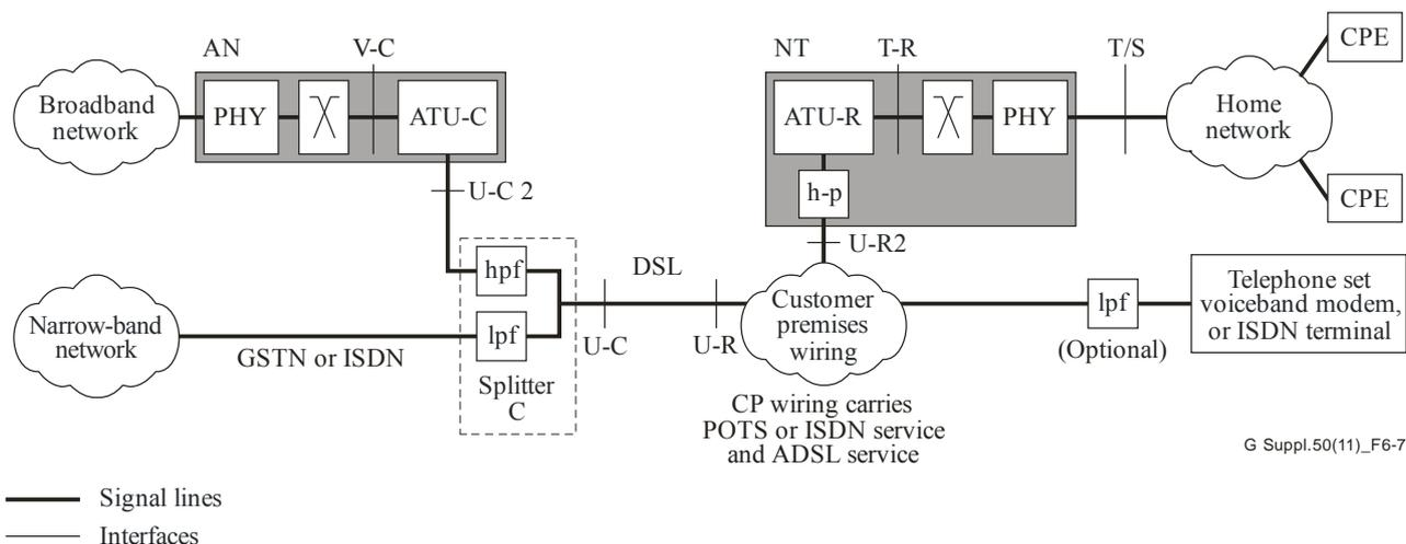
**Figure 6-7 – Generic application reference model for splitterless remote deployment**
