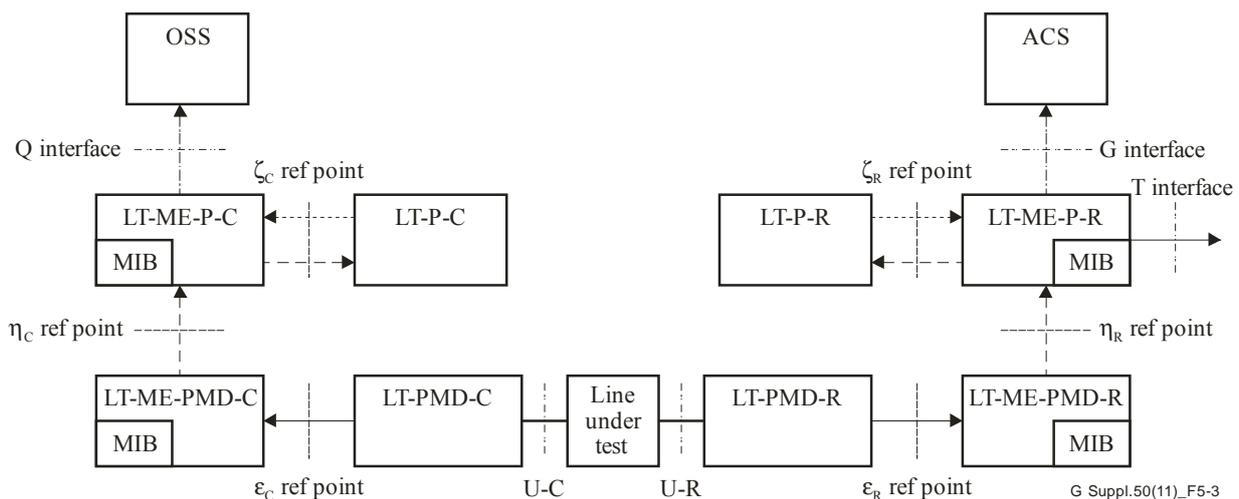
NOTE: arrows show flow of data elements only; flow of control elements are bi-directional (not shown).
