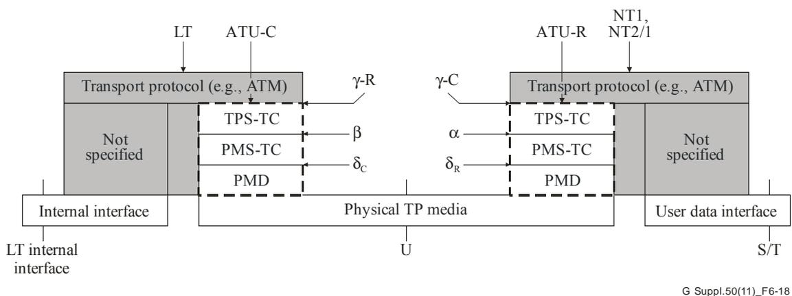
**Figure 6-18 – User plane protocol reference architecture for ITU-T G.992.3, ITU-T G.992.4, and ITU-T G.992.5**
