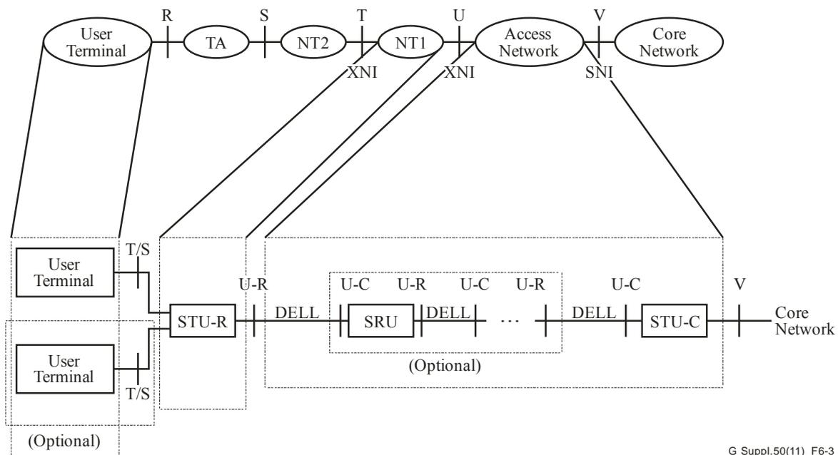
**Figure 6-3 – ITU-T G.991.2 system reference model and its alignment with the generic reference configuration**
