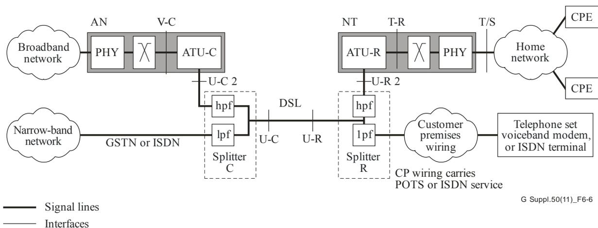
**Figure 6-6 – Generic application reference model for remote deployment with splitter**
