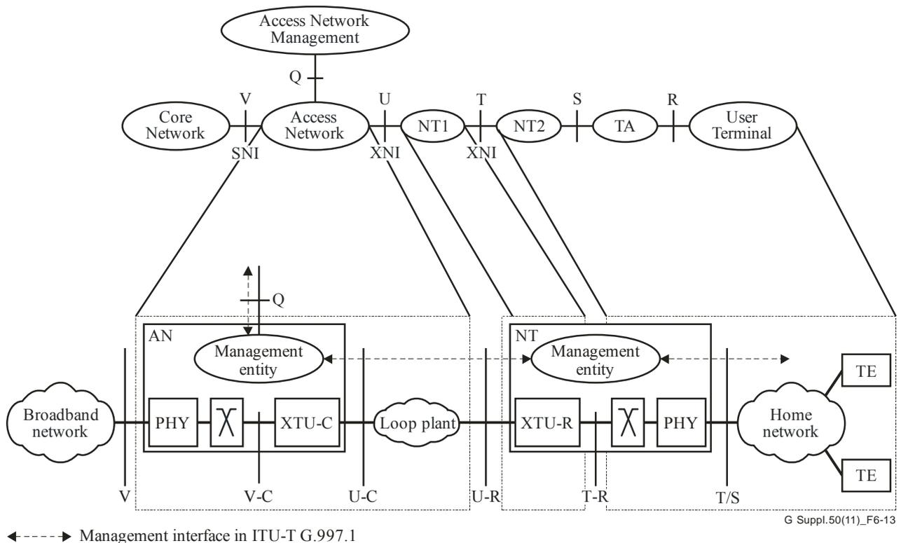
**Figure 6-13 – ITU-T G.997.1 system reference model and its alignment with the generic reference configuration**
