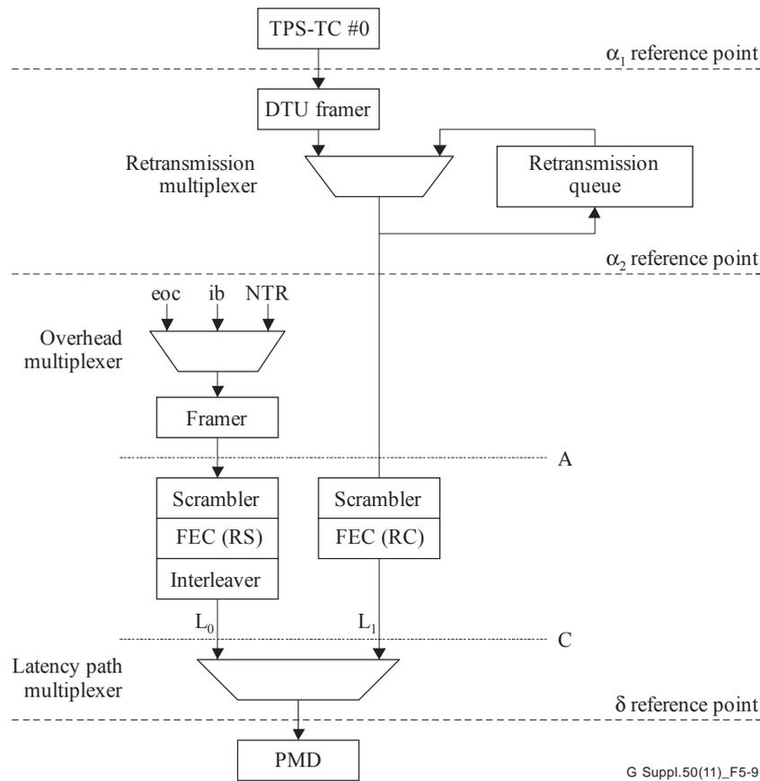
**Figure 5-9 – Reference model in the forward direction when retransmission is enabled in a single direction**
