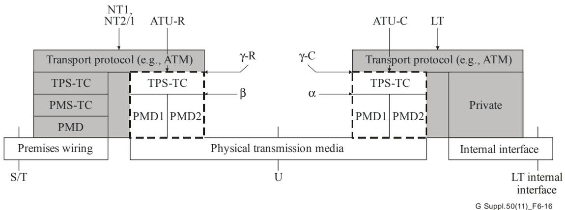
**Figure 6-16 – User plane protocol reference architecture for ITU-T G.991.1**
