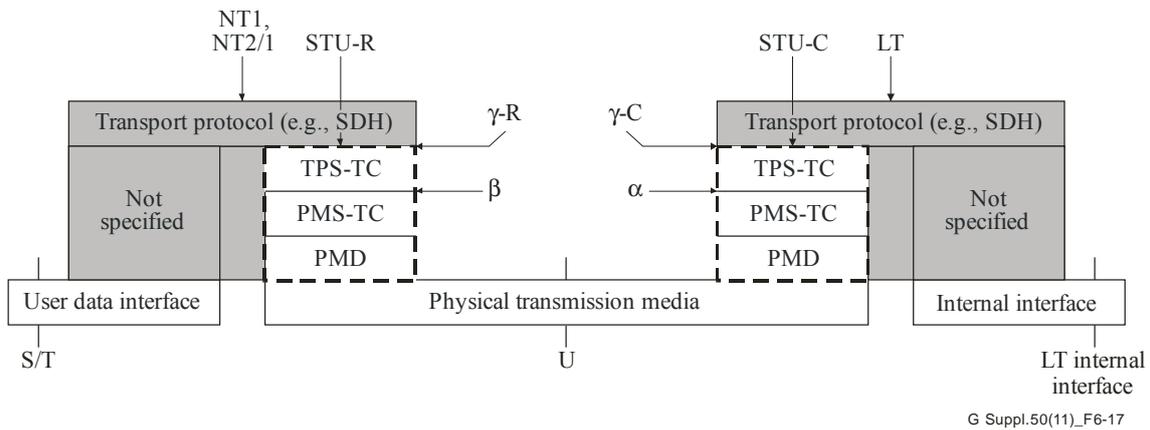
**Figure 6-17 – User plane protocol reference architecture for ITU-T G.991.2**
