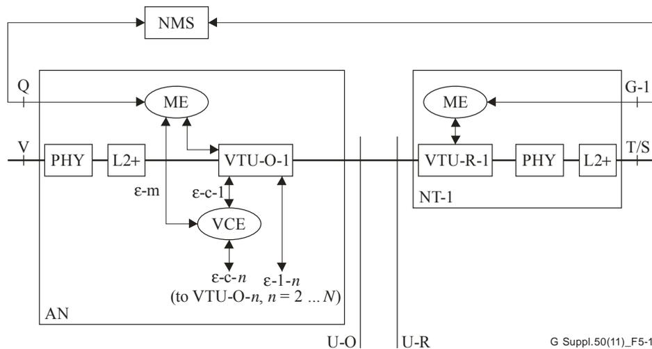
**Figure 5-1 – Reference model for a vectored system (shown for line 1 in a vectored group of  $N$  lines)**
