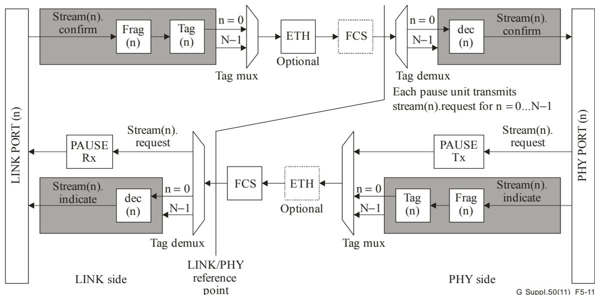
**Figure 5-11 – Reference model for the LINK/PHY interface**
