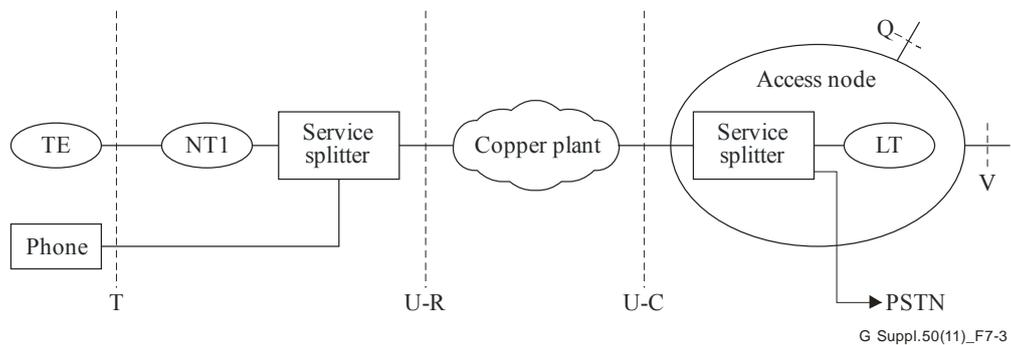
**Figure 7-3 – ITU-T G.992.1 data service presentation at the T interface**
