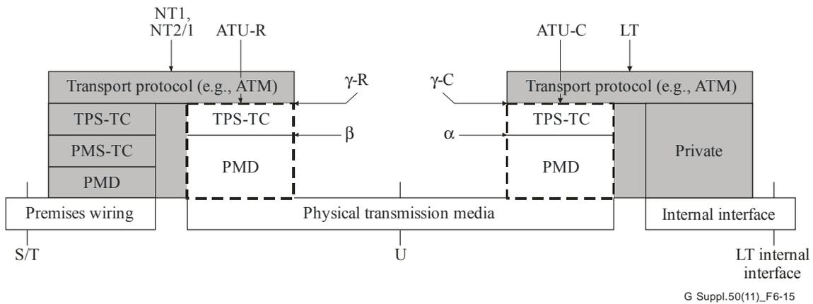
**Figure 6-15 – User plane protocol reference architecture for ITU-T G.992.1 and ITU-T G.992.2**
