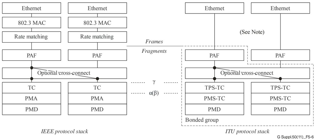
NOTE – A rate matching algorithm may be implemented somewhere above the PAF. The IEEE rate matching algorithm is specifically designed for the Ethernet MAC.
