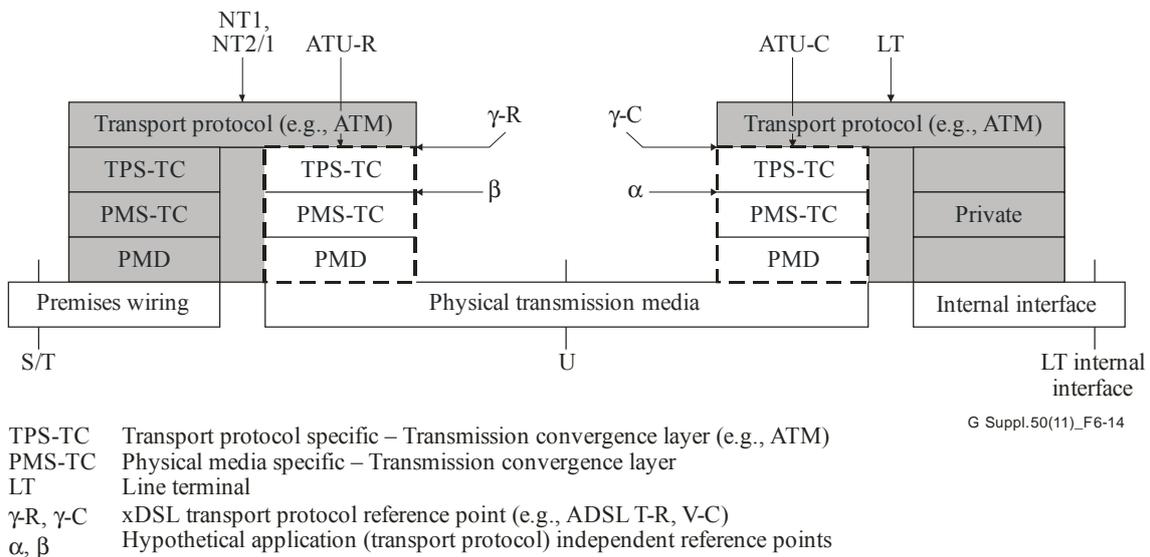
**Figure 6-14 – User plane protocol reference architecture**
