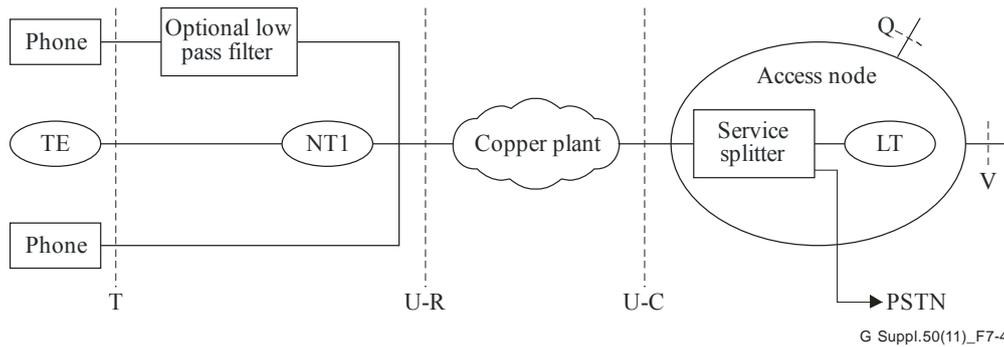
**Figure 7-4 – ITU-T G.992.2 data service presentation at the T interface**
