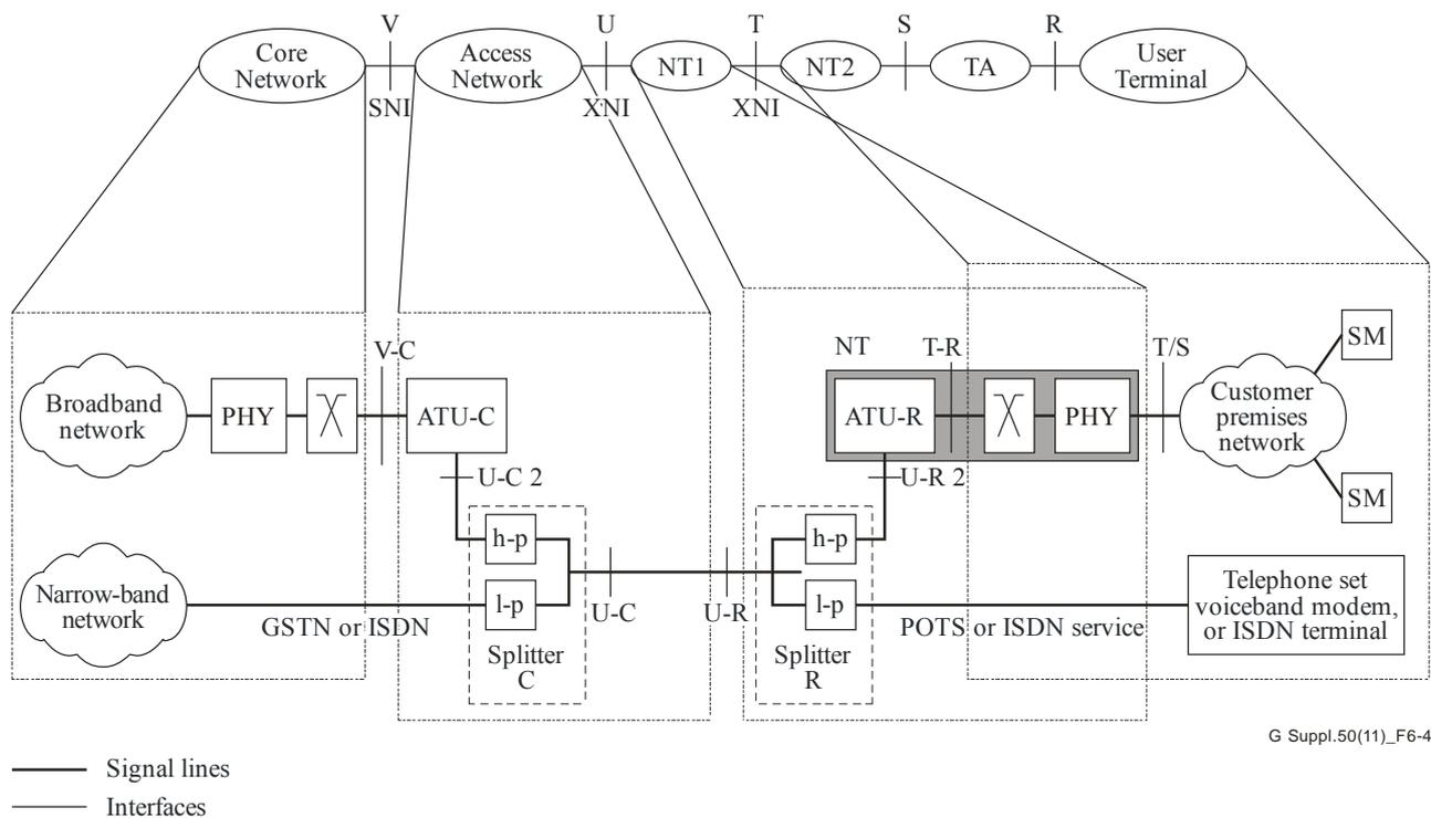
**Figure 6-4 – ITU-T G.992.1 system reference model and its alignment with the generic reference configuration**
