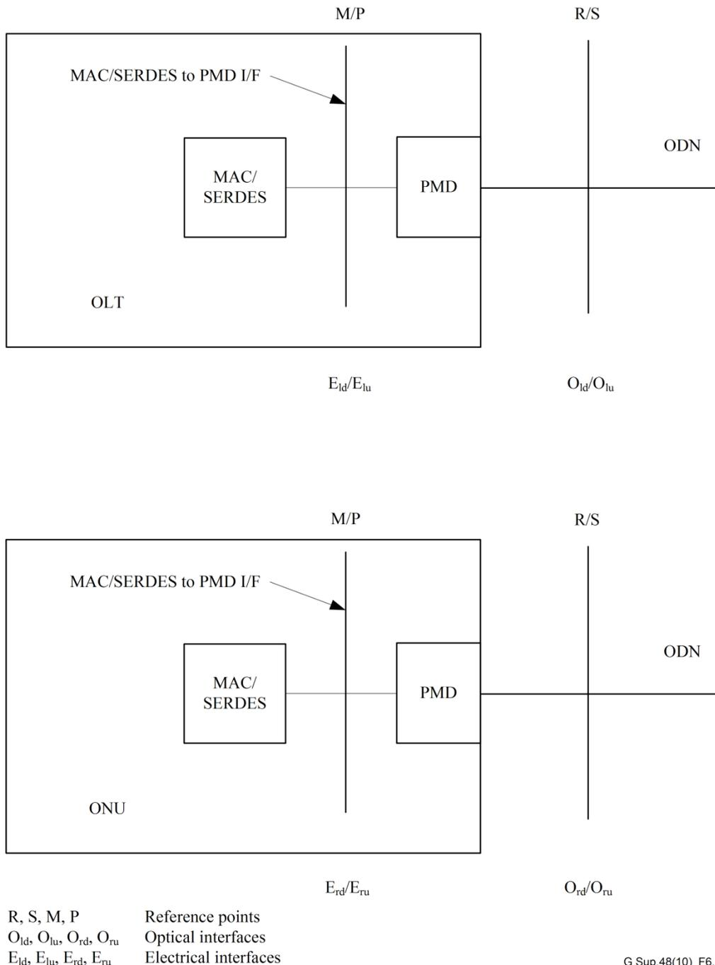
**Figure 6-2 – Reference points between the MAC/SERDES and PMD at the architecture of the ONU and OLT**
