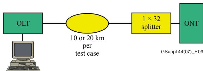
**Figure 9 – Test setup**
