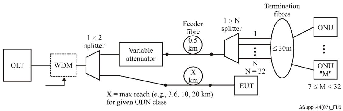
**Figure I.6 – ODN configuration #4 – Far EUT, near cluster**
