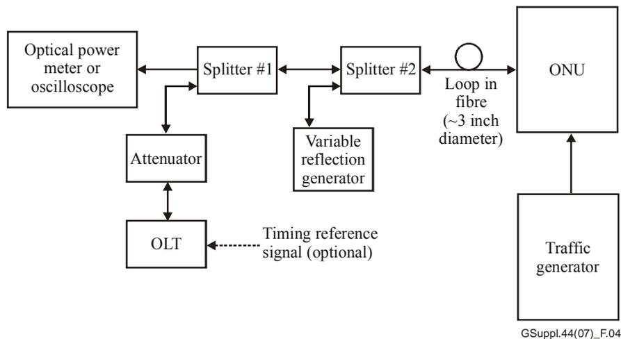
**Figure 4 – ONU mean launched power test configuration<sup>2</sup> – Test setup**
