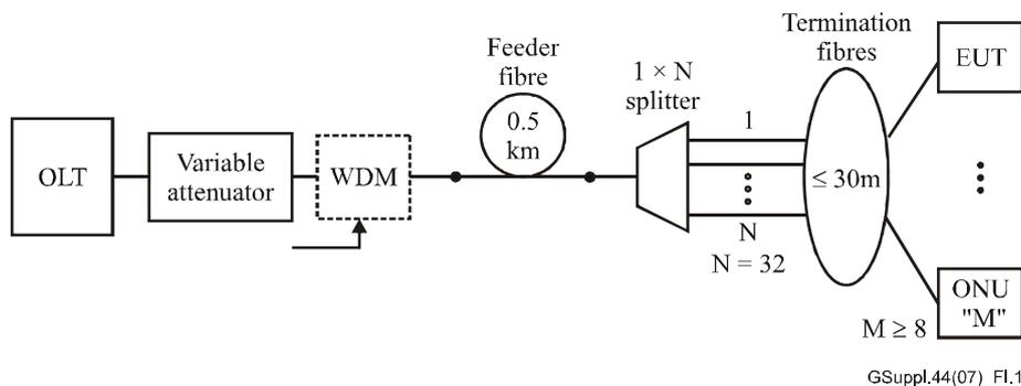
Figure I.1 – ODN configuration #1a – Near cluster, single-stage ODN
