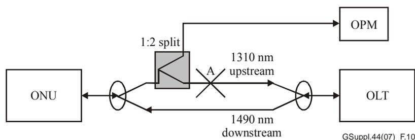
**Figure 10 – Reaction to Deactivate\_PON\_ID test setup**
