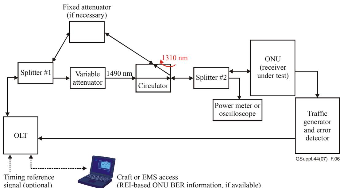
**Figure 6 – Receiver sensitivity test configuration – Test setup**
