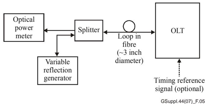
**Figure 5 – OLT mean launched power test configuration – Test setup**
