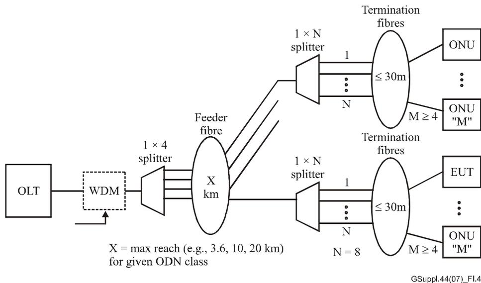
**Figure I.4 – ODN configuration #2b – Far cluster, multi-stage ODN**
