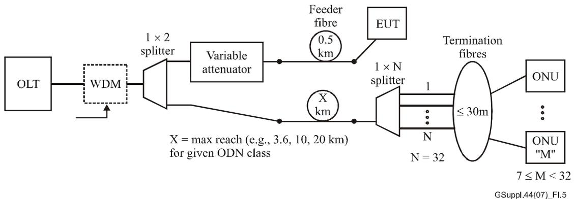
**Figure I.5 – ODN configuration #3 – Near EUT, far cluster**
