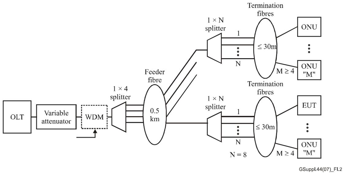
**Figure I.2 – ODN configuration #1b – Near cluster, multi-stage ODN**
