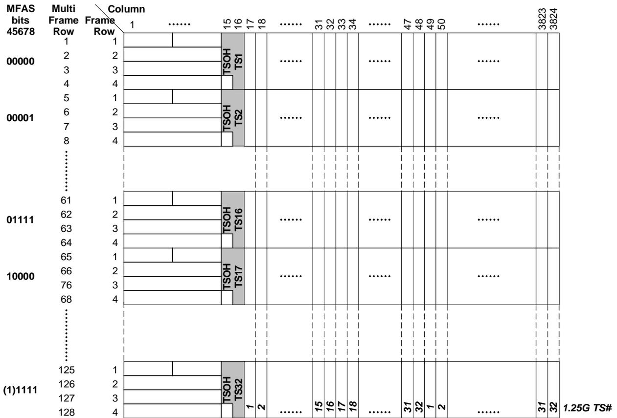
**Figure 9-8 – OPU3e2 tributary slot allocation**
