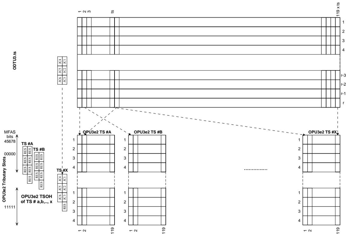
**Figure 9-9 – Mapping of ODTU3e2.ts into 'ts' OPU3e2 1.25G tributary slots**
