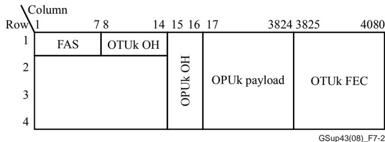
**Figure 7-2 – Mapping frame without fixed stuff bytes**
