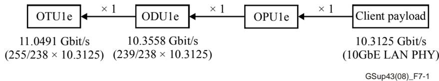
**Figure 7-1 – Mapping structure without fixed stuffing**
