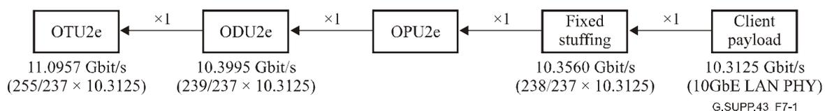
**Figure 7-1 – Mapping structure with fixed stuffing**
