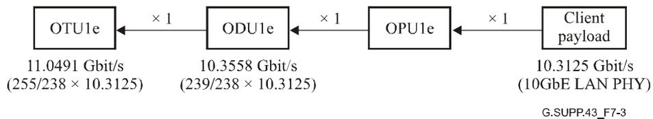
**Figure 7-3 – Mapping structure without fixed stuffing**
