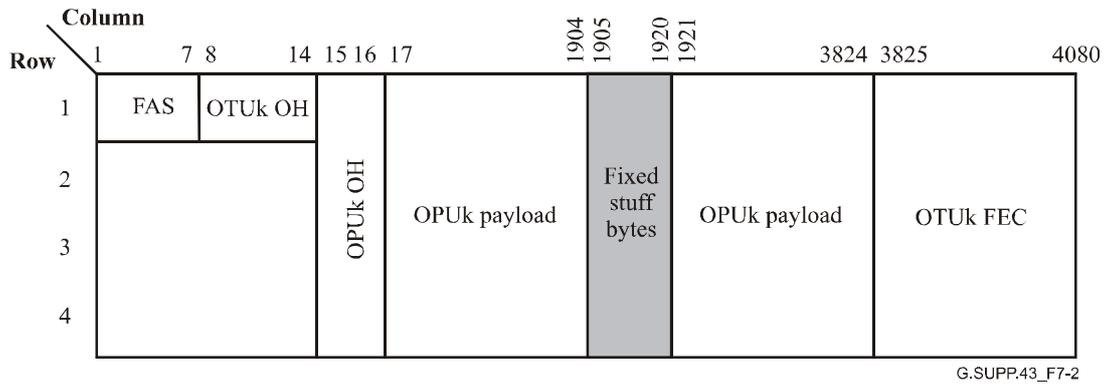
**Figure 7-2 – Mapping frame with fixed stuff bytes**
