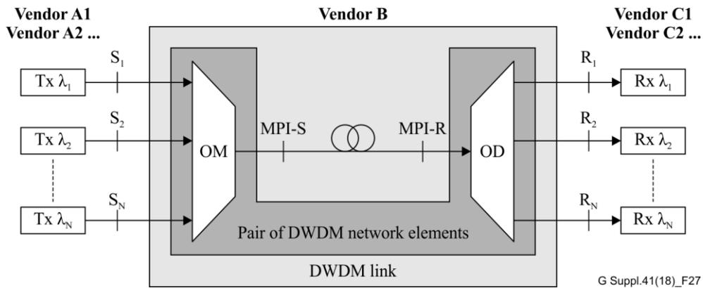
Figure 27 – Single-span black-link transverse compatibility
