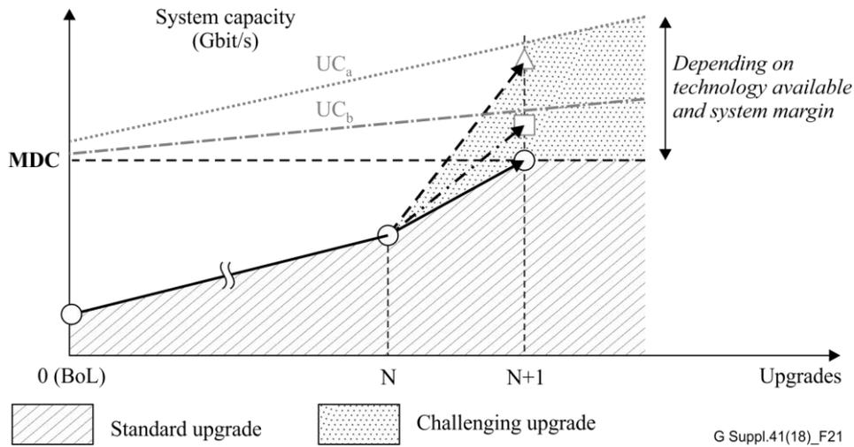
NOTE –  $UC_a$  (resp.  $UC_b$ ) is UC when replacing (resp. keeping) the existing equipment.
