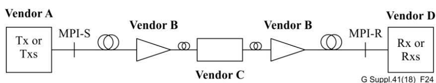
**Figure 24 – Multi-span black-box full transverse compatibility**
