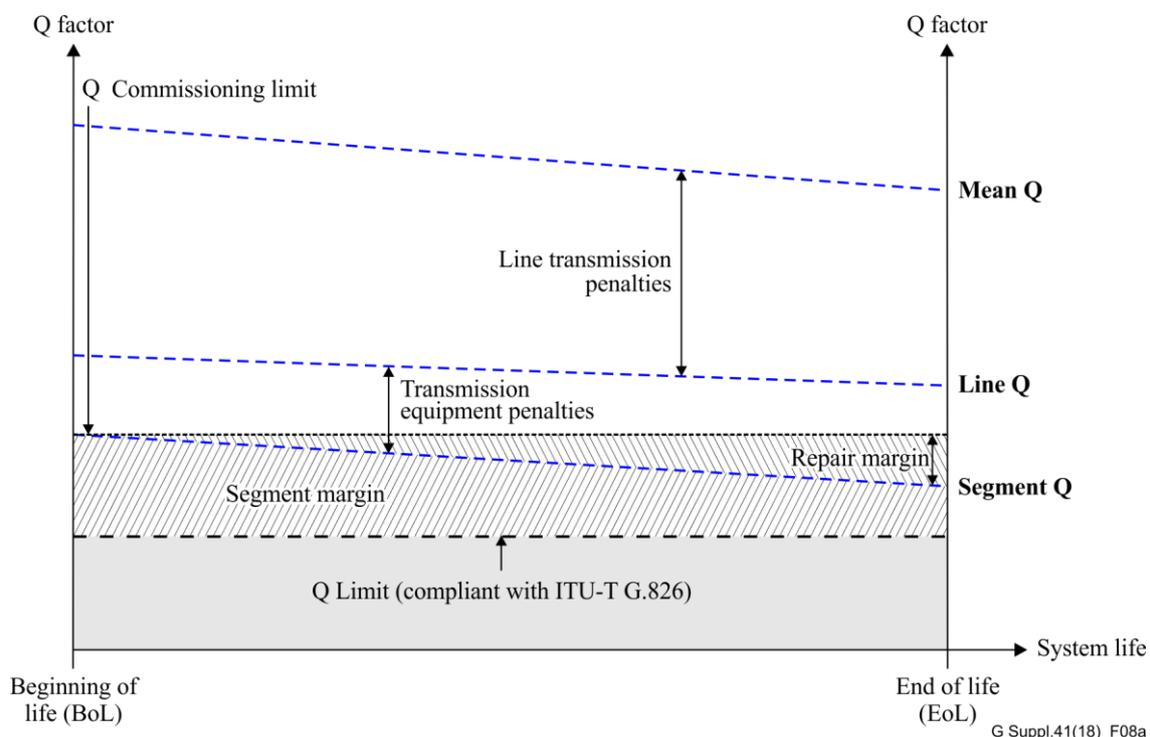
**Figure 8-a – Power budget structure of example 1**
