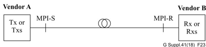
**Figure 23 – Single-span black-box transverse compatibility**
