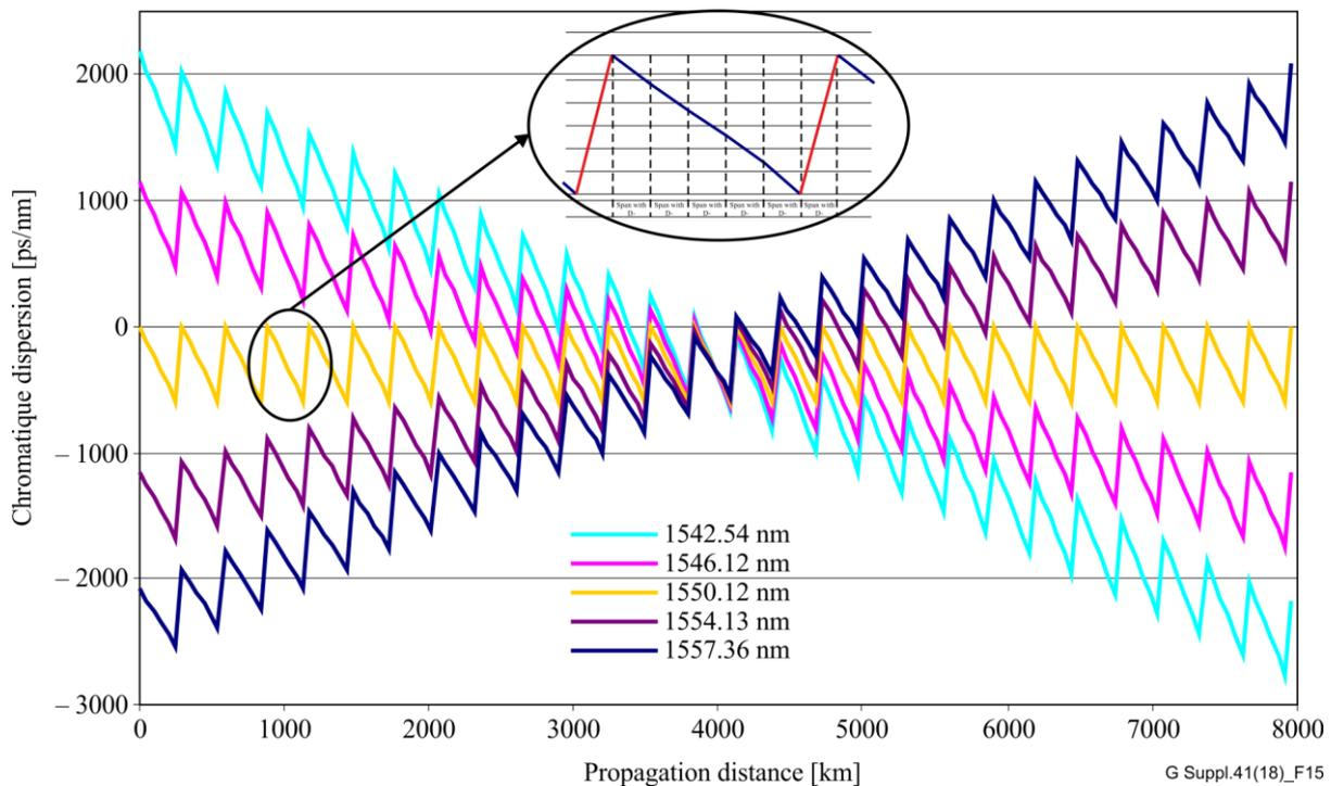
**Figure 15 – Typical chromatic dispersion map for a submarine WDM system with 163 spans designed for 40 wavelengths centred around 1550.12 nm**
