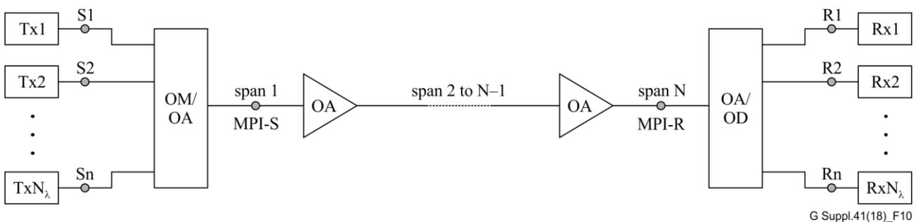
**Figure 10 – Representation of optical line system interfaces
