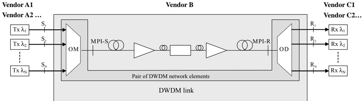
Figure 11-7 – Multi-span black-link transverse compatibility
