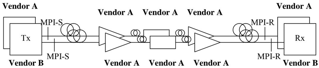
**Figure 11-5 – Multi-span black-box multiple-link transverse compatibility**
