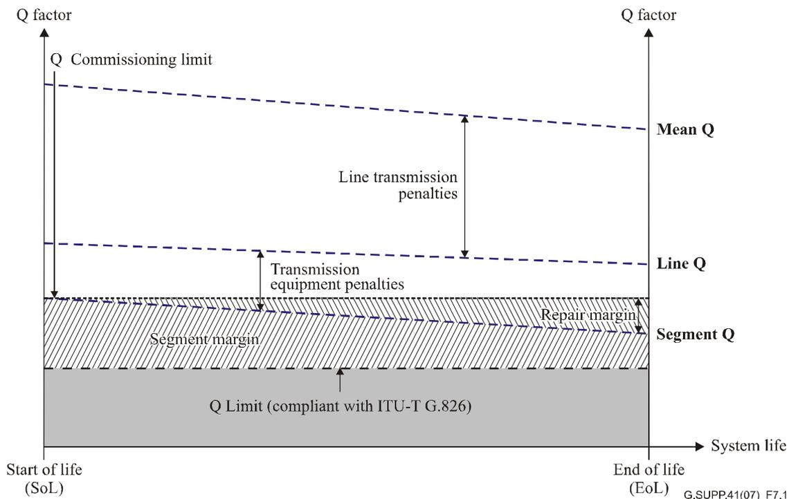
**Figure 7-1 – Power budget structure example**
