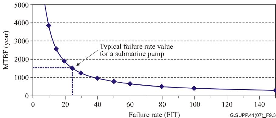
**Figure 9-3 – MTBF for a second pump failure in the same repeater in a typical transatlantic link composed by 1 fibre pair and 150 repeaters with four redundant pumps each**
