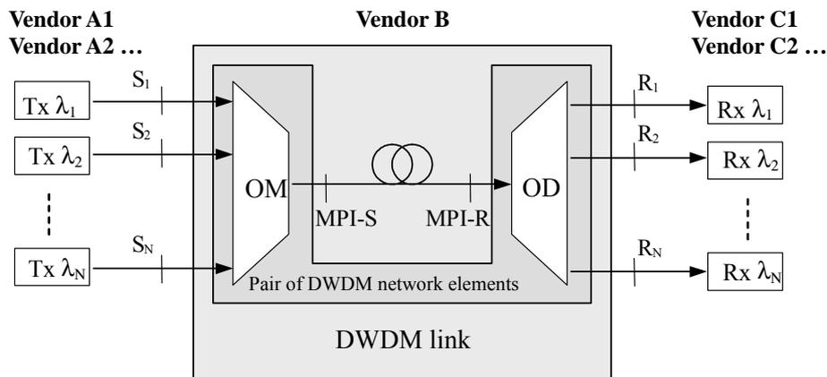
**Figure 11-6 – Single-span black-link transverse compatibility**
