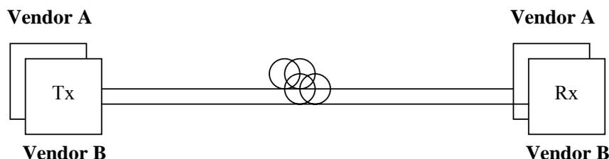
Figure 11-1 – Single-span longitudinal compatibility
