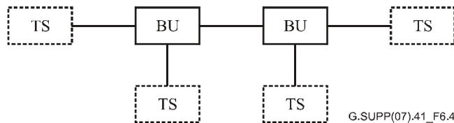
Figure 6-4 – Topology of trunk and branch
