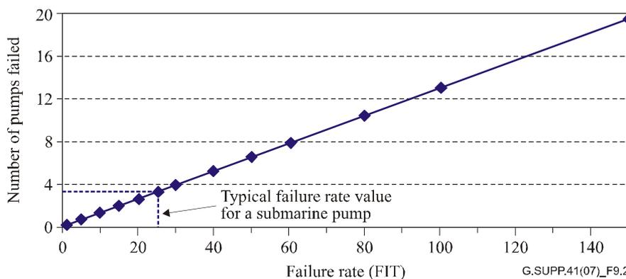
**Figure 9-2 – Estimated number of pump failed in the 25 years for a typical transatlantic link composed of 1 fibre pair and 150 repeaters containing four pumps each**
