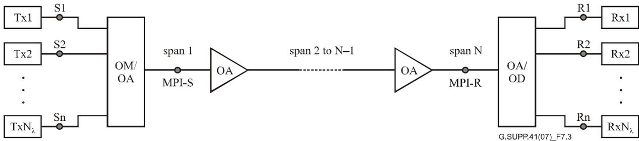
**Figure 7-3 – Representation of optical line system interfaces
