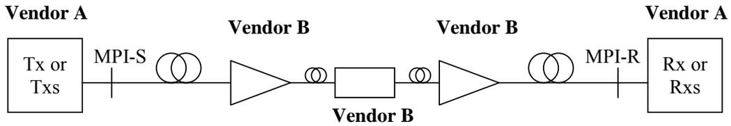
**Figure 11-4 – Multi-span black-box single-link transverse compatibility**
