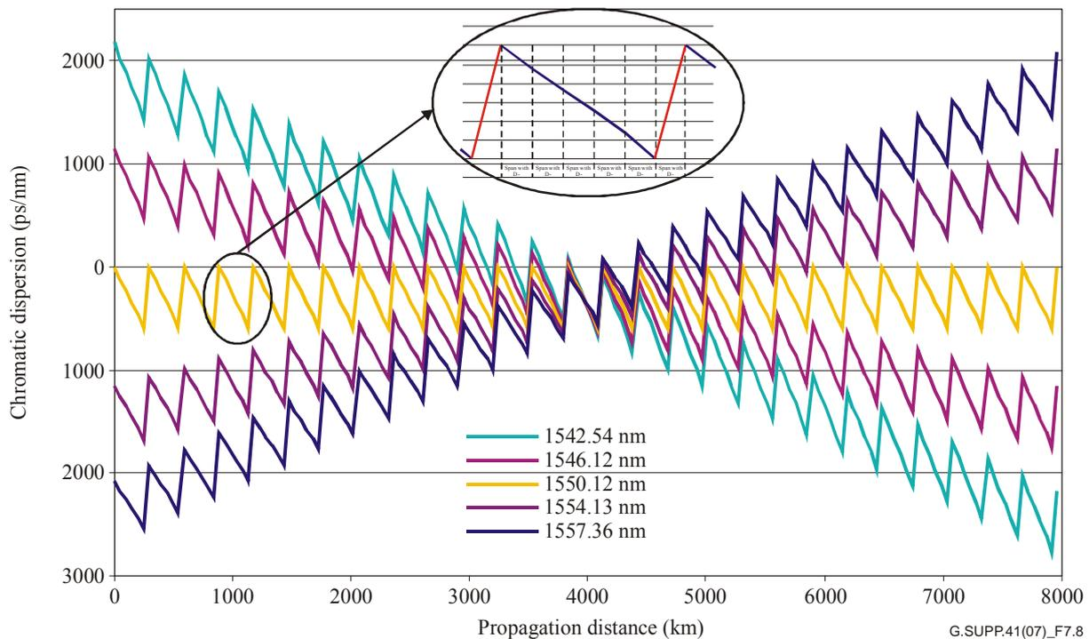
**Figure 7-8 – Typical chromatic dispersion map for a submarine WDM system with 163 spans designed for 40 wavelengths centred around 1550.12 nm WDM system**
