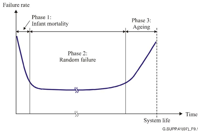
**Figure 9-1 – Typical failure's rate behaviour during the life of a system**
