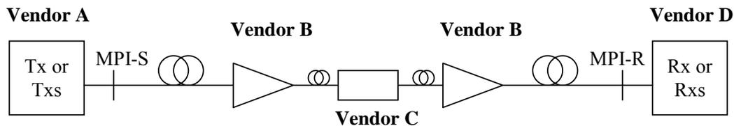
Figure 11-3 – Multi-span black-box full transverse compatibility
