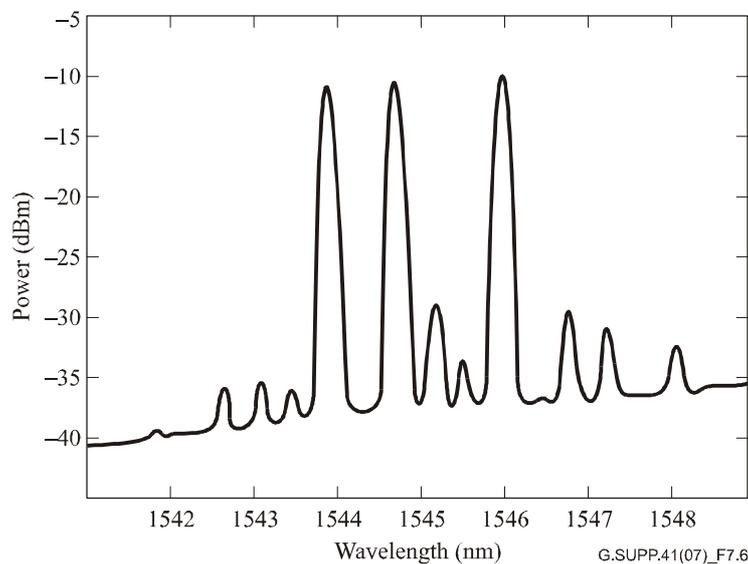
**Figure 7-6 – Optical power spectrum measured at the output of 25 km length of dispersion shifted ( $D = -0.2$  ps/nm · km at the central channel) when 3 mW channels are used [b-Tkach]**
