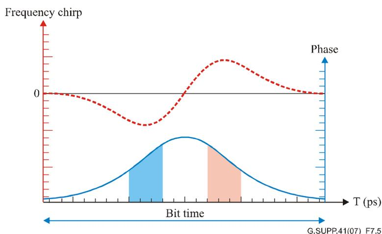
**Figure 7-5 – Temporal variation of the phase shift and the frequency chirp induced by SPM [b-Agrawal]**
