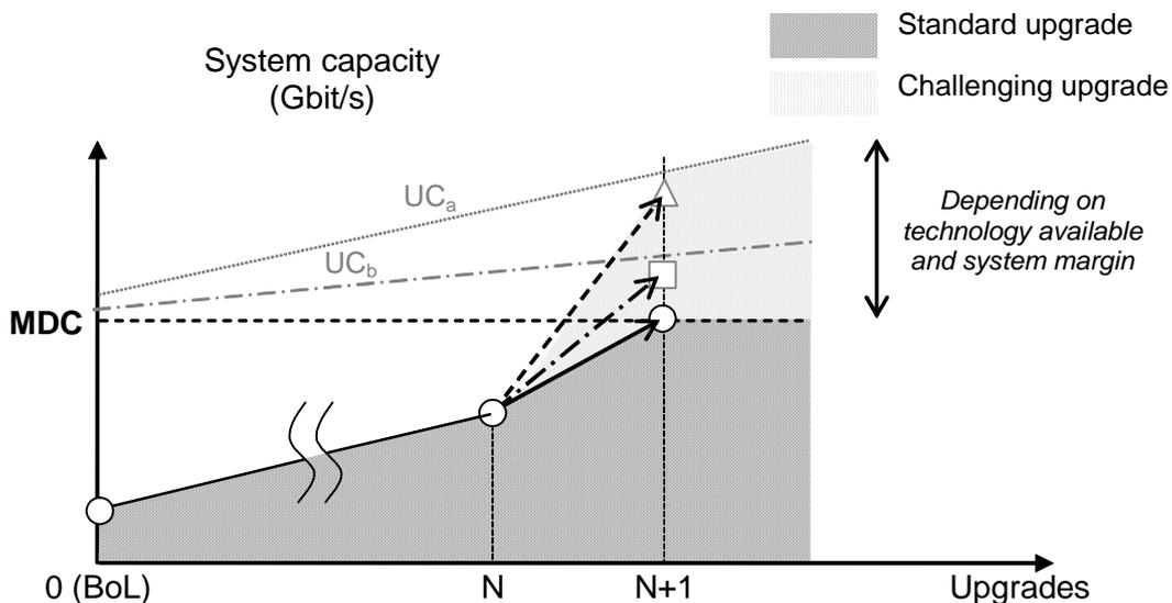
NOTE –  $UC_a$  (resp.  $UC_b$ ) is UC when replacing (resp. keeping) the existing equipment. Note that curve  $UC_b$  is deduced from curve  $UC_a$  and the actual system loading. For clarity purposes, curve  $UC_a$  was assumed quasi linear.
