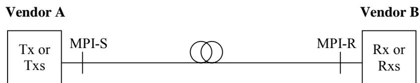
Figure 11-2 – Single-span black-box transverse compatibility
