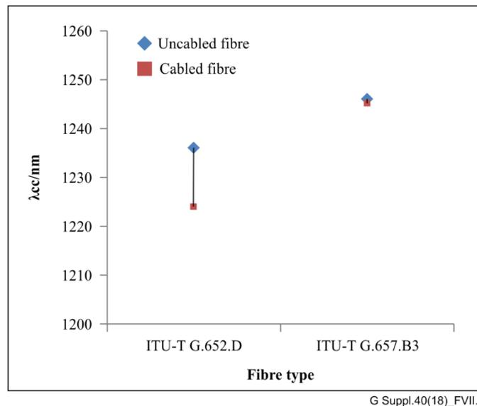
**Figure VII.4 – Comparison of  $\lambda_{cc}$  on cabled/uncabled fibres (Cable B, tight buffered fibre type)**
