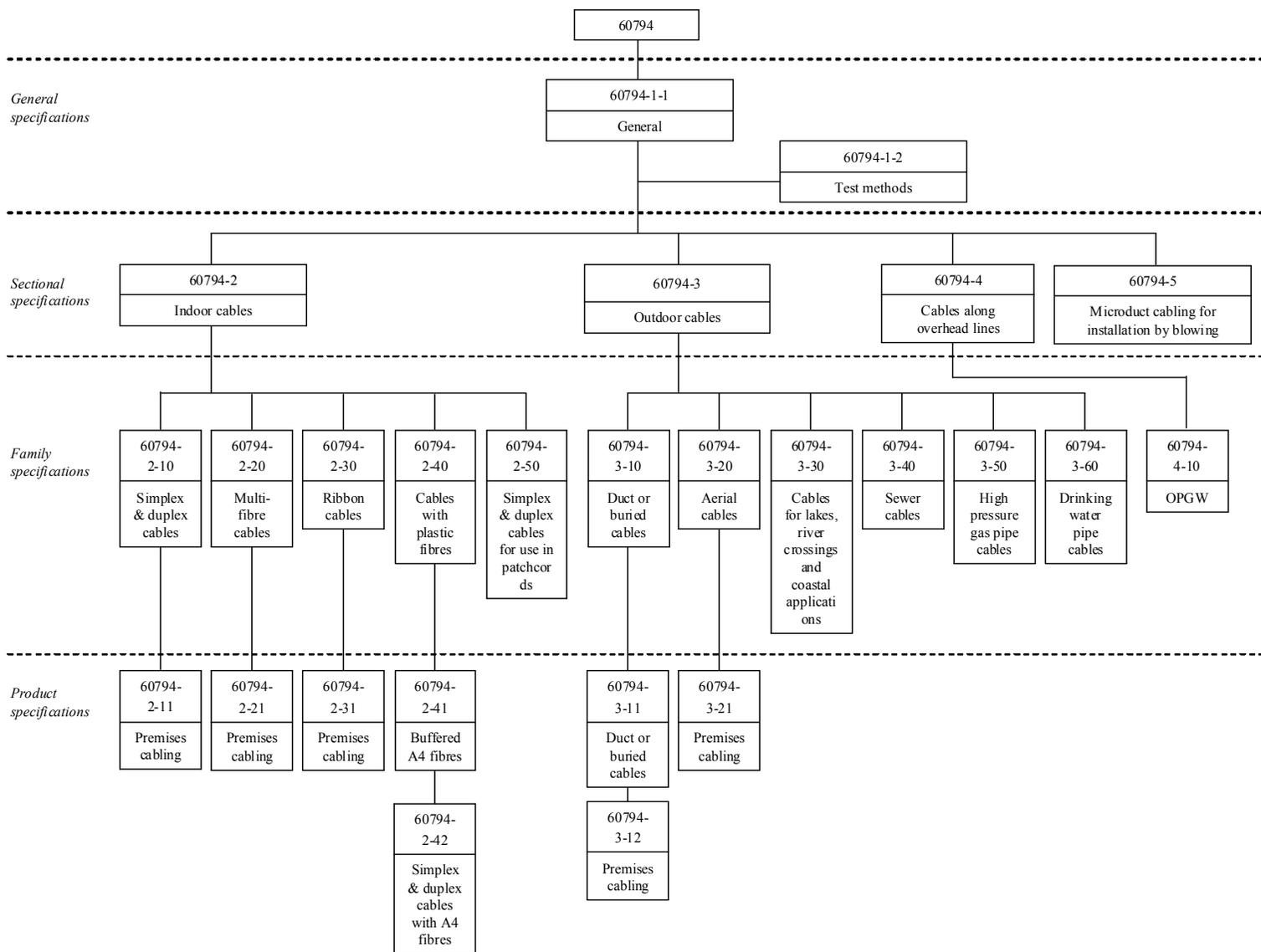
**Figure V.1 – Status of [IEC 60794.x] regarding optical cables**
