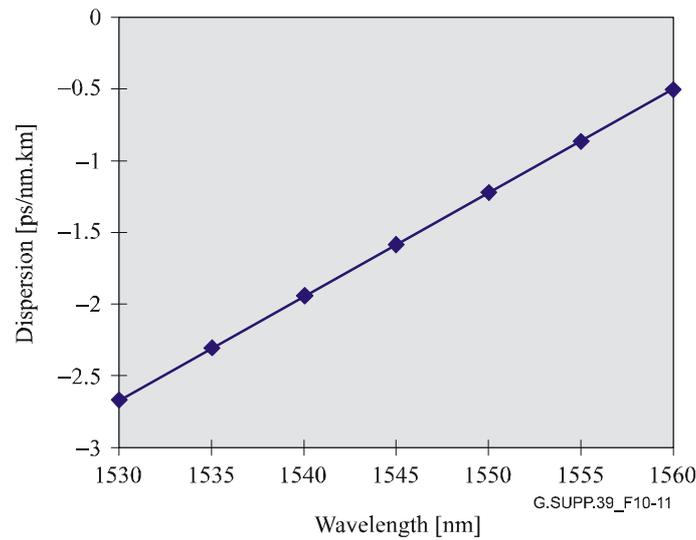
**Figure 10-11 – Average dispersion coefficient vs wavelength**
