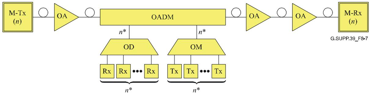
**Figure 8-7 – Example of a bus structure with optical amplifiers and one OADM**
