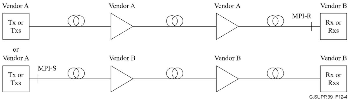
Figure 12-4 – Multi-span single interface transverse compatibility
