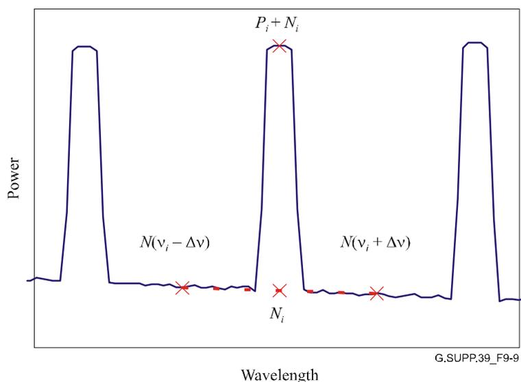
**Figure 9-9 – OSNR measurement from the optical spectrum**
