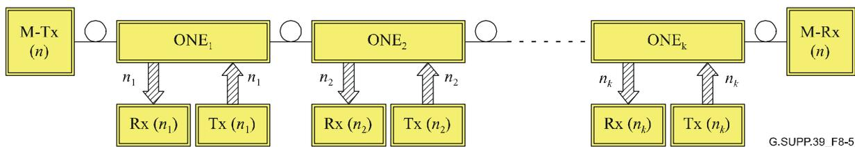
**Figure 8-5 – Generic representation of a bus structure**
