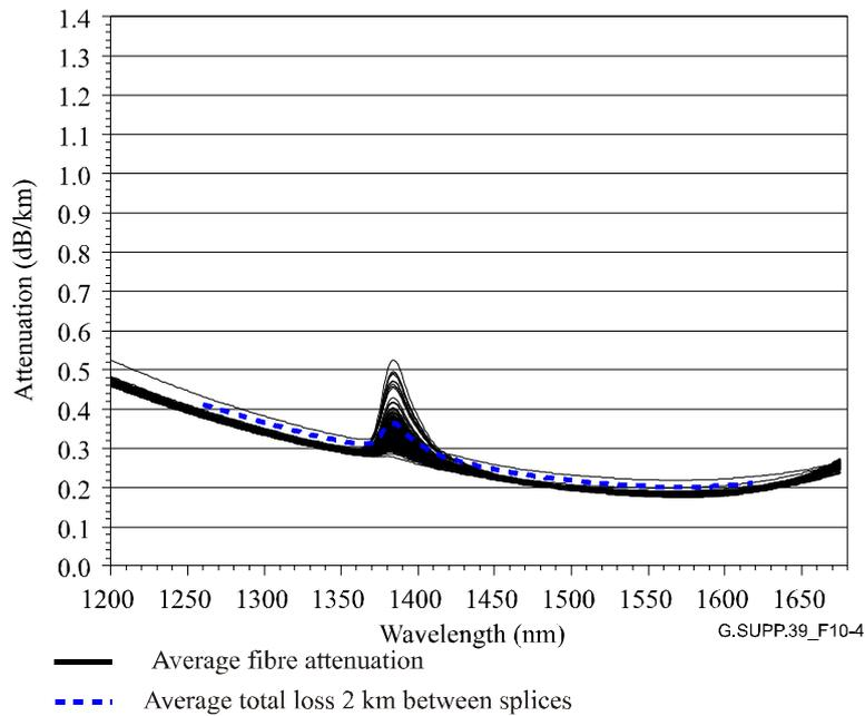
**Figure 10-4 – Measured fibre attenuation and splice loss in installed G.652 A&B cable – Cables installed in 2003**
