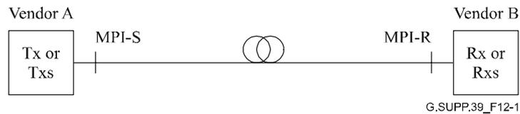
**Figure 12-1 – Single-span physical layer transverse compatibility**
