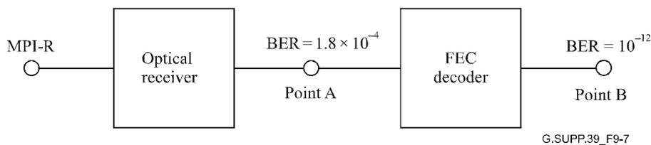
**Figure 9-7 – Effect of usage of FEC on receiver performance in relation to the Bit Error Ratio**
