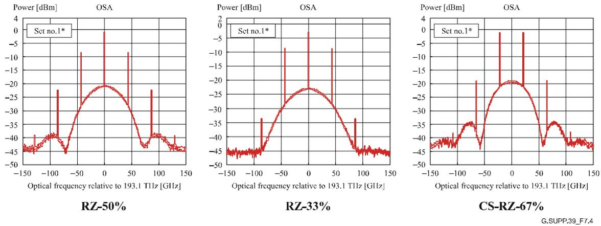
**Figure 7-4 – Optical spectra of RZ formats**
