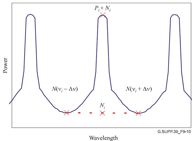
**Figure 9-10 – Inaccurate OSNR measurement due to noise shaping**
