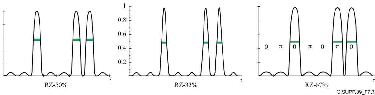
NOTE – The bar indicates FWHM and the duty cycle of the pulses.  $\pi$  and 0 indicate the phase change of RZ pulses at CS-RZ-67%.
