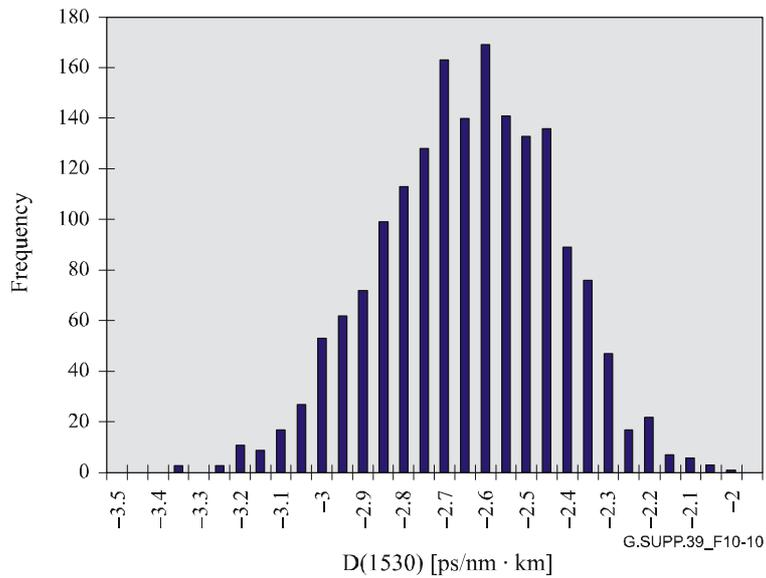
**Figure 10-10 – Histogram of dispersion coefficient values at 1530 nm**
