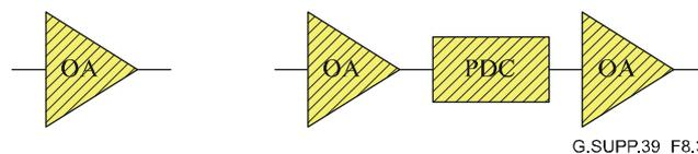
**Figure 8-3 – Examples of 1R regenerator realization schemes**
