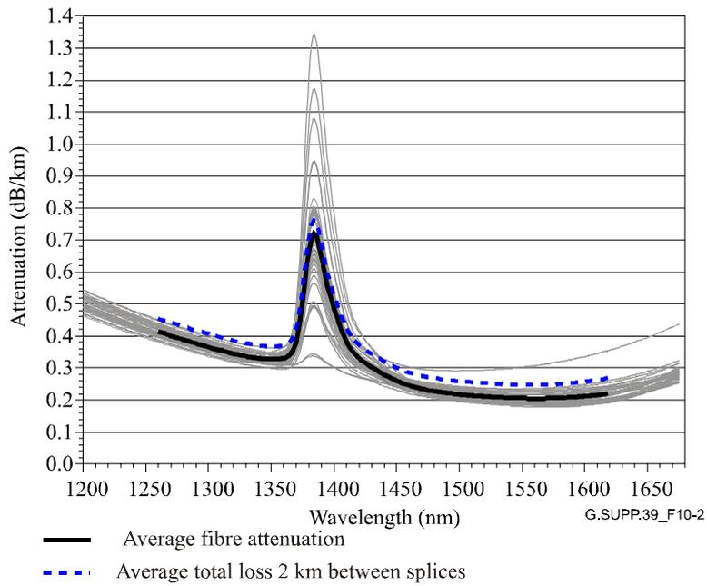
**Figure 10-2 – Measured fibre attenuation and splice loss in installed G.652 A&B cable – Cables installed before 1990**
