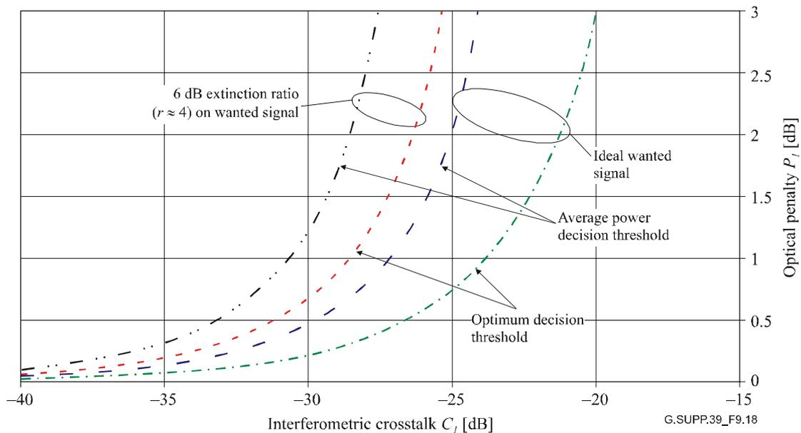
**Figure 9-18 – Graph of optical penalty vs interferometric crosstalk for multiple interferers (Gaussian model)**
