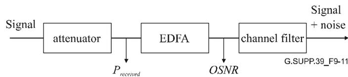
**Figure 9-11 – Setup for OSNR measurement**
