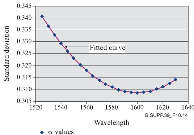
**Figure 10-14 – Standard deviation of chromatic dispersion coefficient of G.652 fibre**
