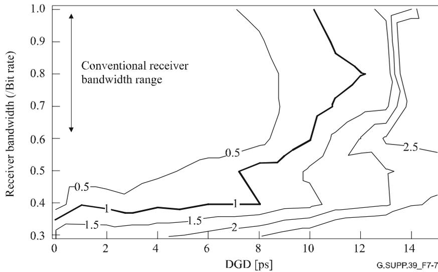
**Figure 7-7 – Contour map for DGD tolerance (RZ-33%)**
