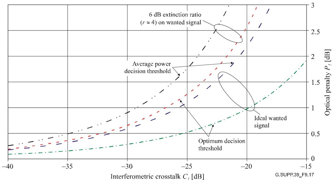
**Figure 9-17 – Graph of optical penalty vs interferometric crosstalk for a single interferer (bounded model)**
