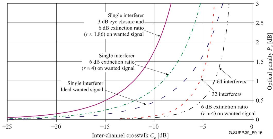
**Figure 9-16 – Graph of optical penalty vs inter-channel crosstalk**
