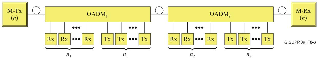
**Figure 8-6 – Example of a bus structure with two OADM and one fibre for each added/dropped WDM channel**
