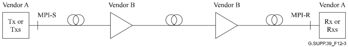
Figure 12-3 – Multi-span physical layer partial transverse compatibility
