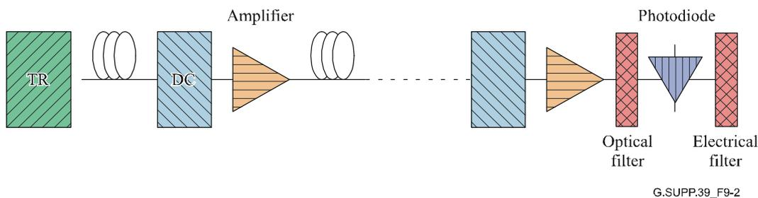
**Figure 9-2 – Scheme of the system with periodic post-compensation**
