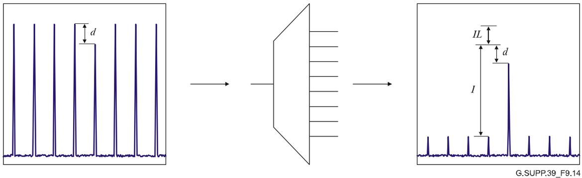
**Figure 9-14 – Simple demultiplexer example**
