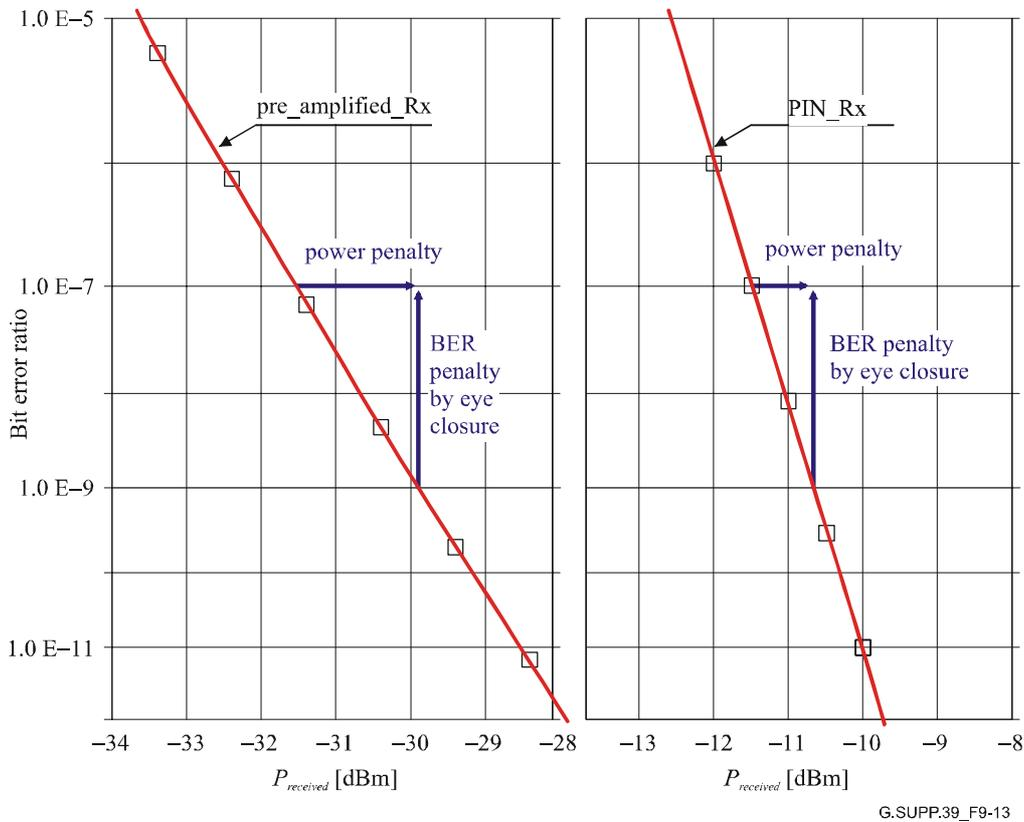
**Figure 9-13 – BER vs received power with and without an optical preamplifier**
