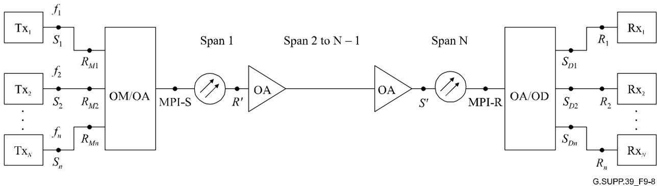
**Figure 9-8 – Representation of optical line system interfaces
