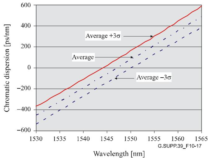
**Figure 10-17 – 3  $\sigma$  limits for combined G.652 fibre and compensators**
