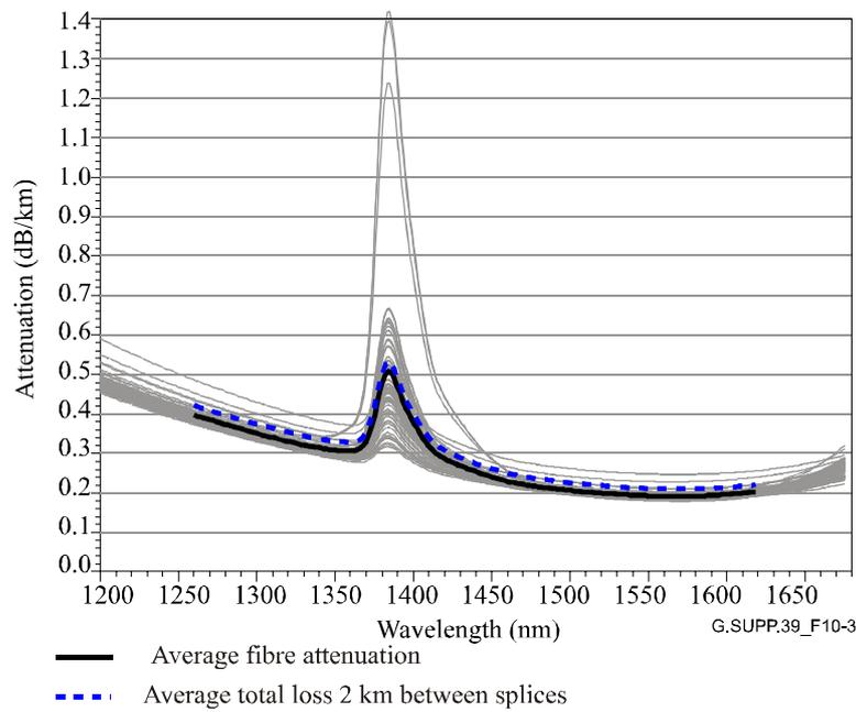
**Figure 10-3 – Measured fibre attenuation and splice loss in installed G.652 A&B cable – Cables installed around 2000**
