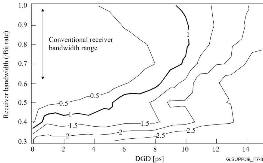
**Figure 7-8 – Contour map for DGD tolerance (RZ-50%)**
