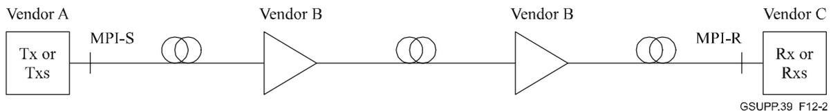
**Figure 12-2 – Multi-span physical layer full transverse compatibility**
