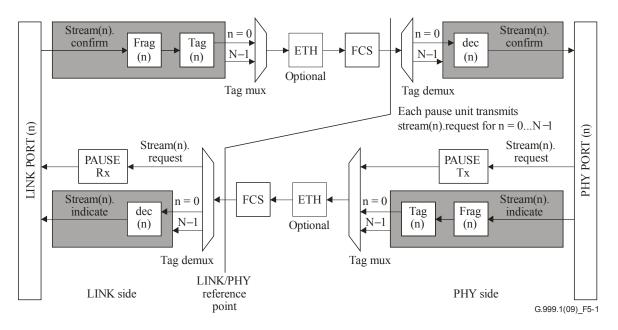
Figure 5-1 – Reference model for the LINK/PHY interface
