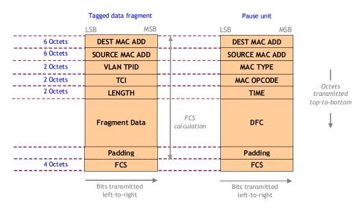
**Figure 6-8 – Final encapsulation format with Ethernet encapsulation**
