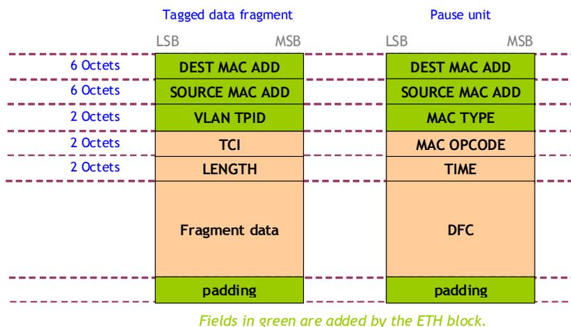
**Figure 6-5 – Ethernet adapted format**
