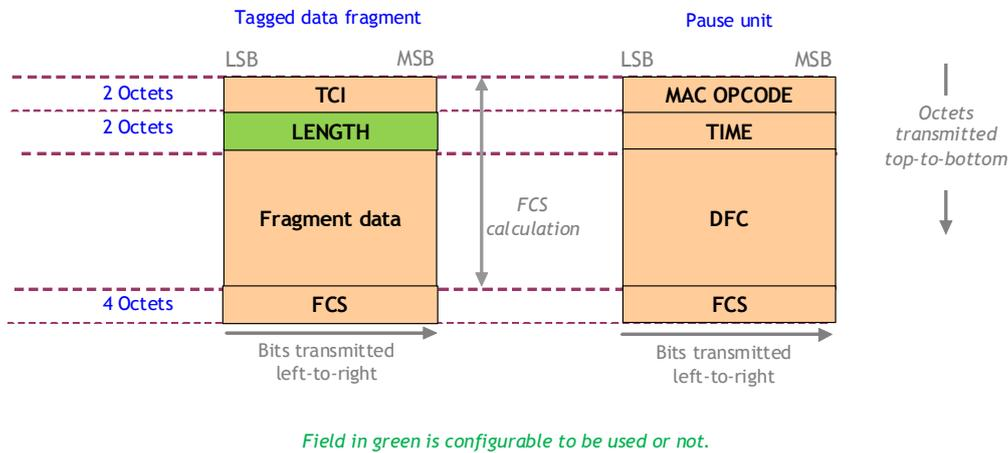
**Figure 6-7 – Final encapsulation format without Ethernet encapsulation**
