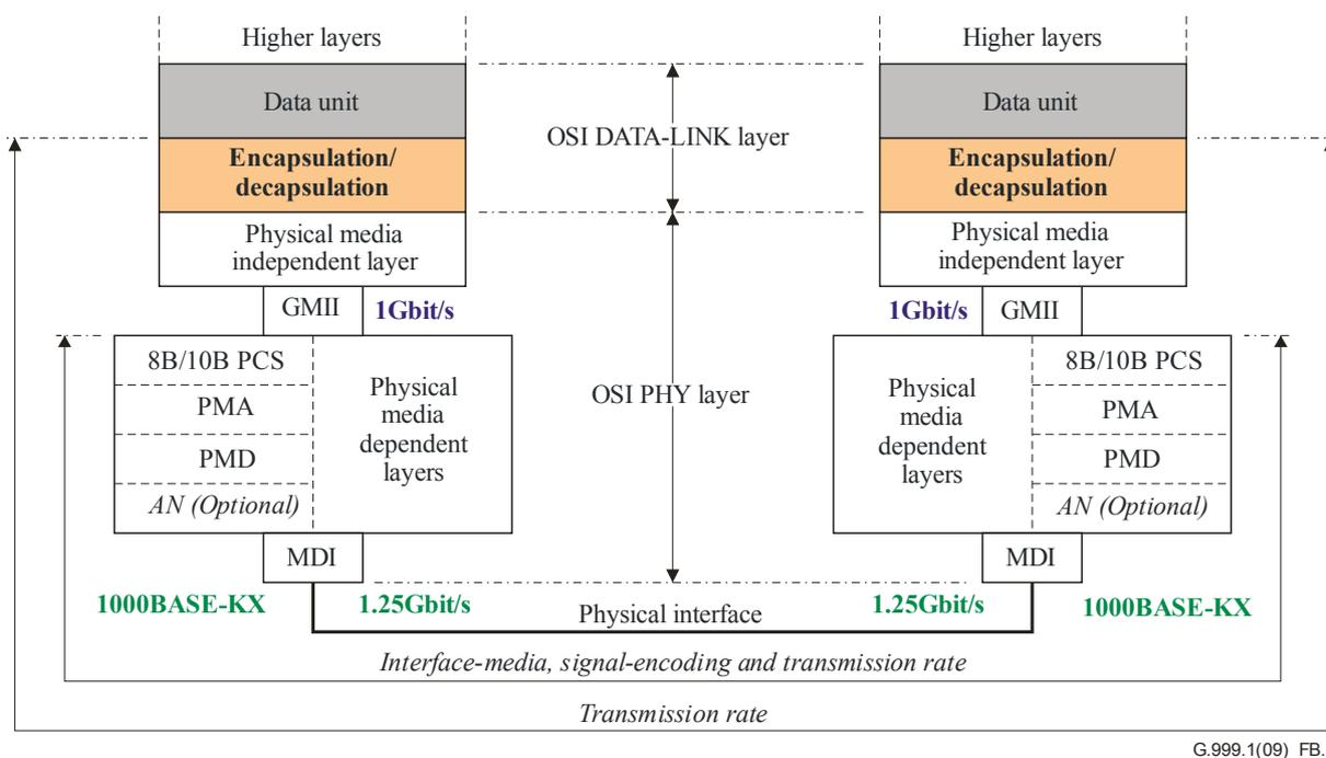
**Figure B.1 – LINK/PHY interface based on 1000BASE-KX**
