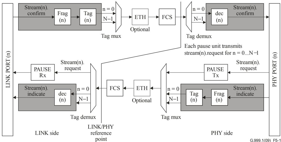
**Figure 5-1 – Reference model for the LINK/PHY interface**
