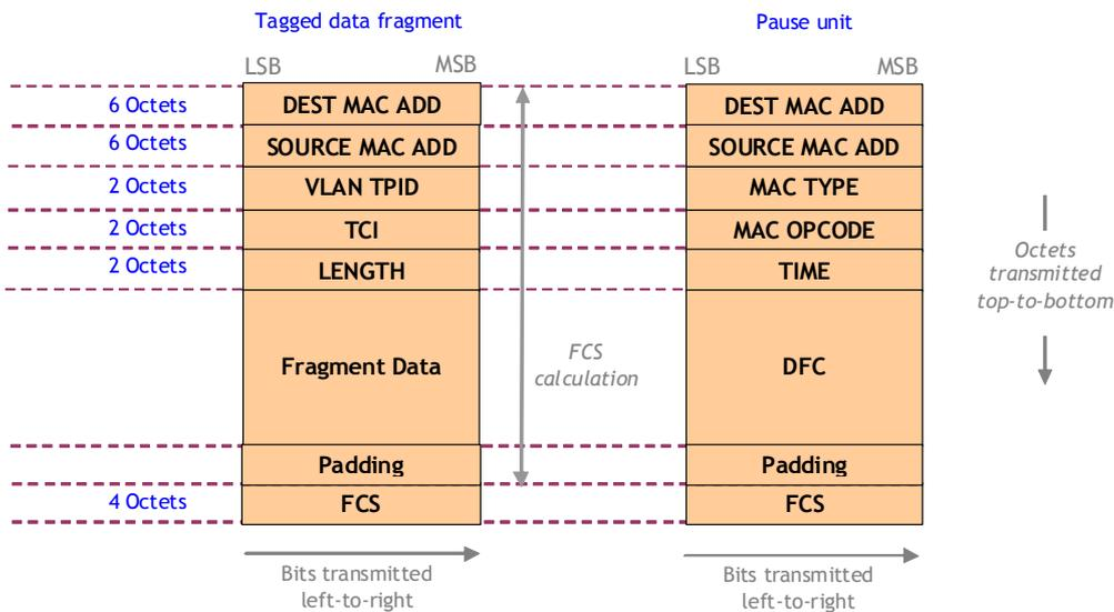
**Figure 6-8 – Final encapsulation format with Ethernet encapsulation**
