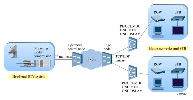
Figure 6-6 – Schematic architecture diagram of BTV unicast
