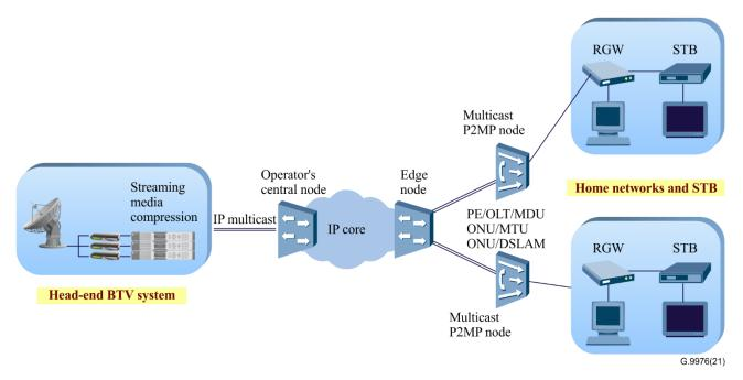
Figure 6-5 – Schematic architecture diagram of BTV multicast
