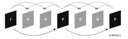
**Figure I.1 – Frame types during video encoding**
