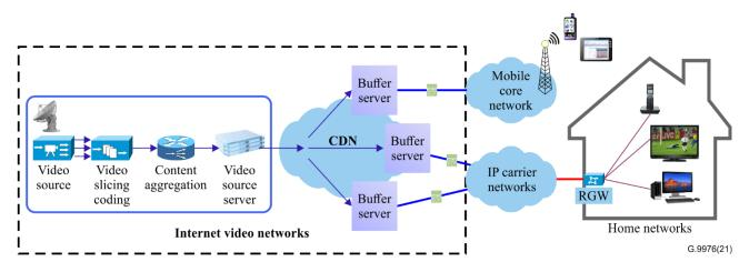
Figure 6-7 – Schematic architecture diagram of BTV by Internet
