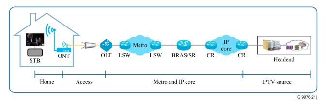
**Figure 8-2 – Decomposition diagram of bearer network for 4K**
