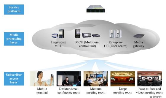
Figure 6-10 – Schematic diagram of video conferencing architecture
