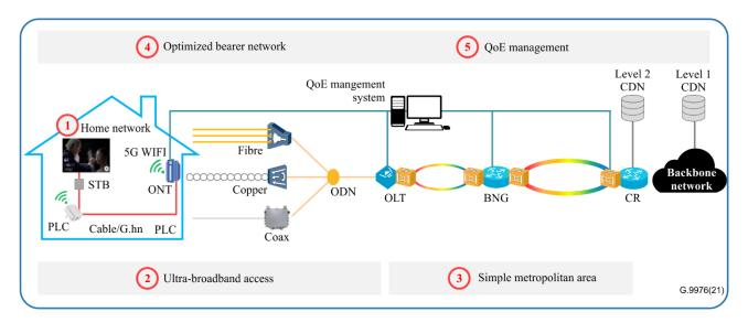
Figure 8-1 – The target architecture of the video carrier network with the best experience
