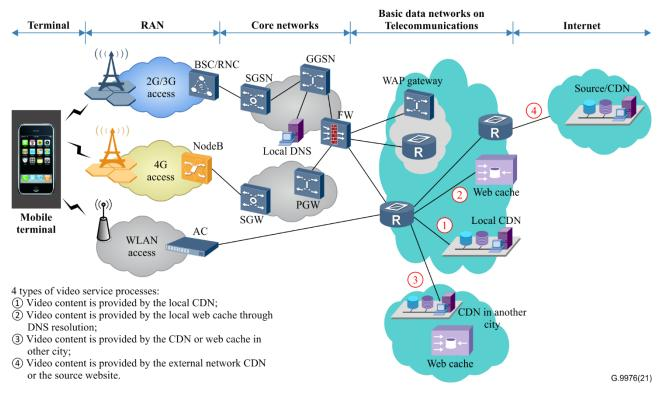
Figure 6-8 – Schematic architecture diagram of mobile BTV video broadcast
