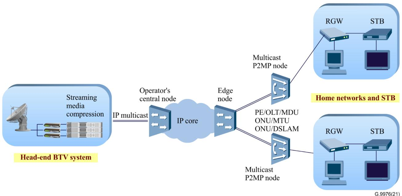
**Figure 6-5 – Schematic architecture diagram of BTV multicast**
