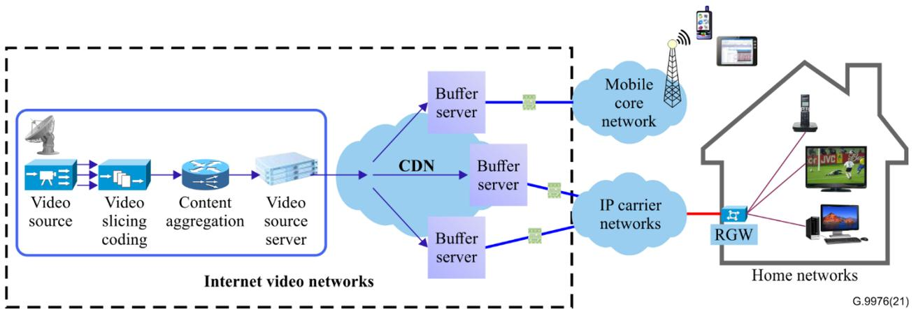
**Figure 6-7 – Schematic architecture diagram of BTV by Internet**
