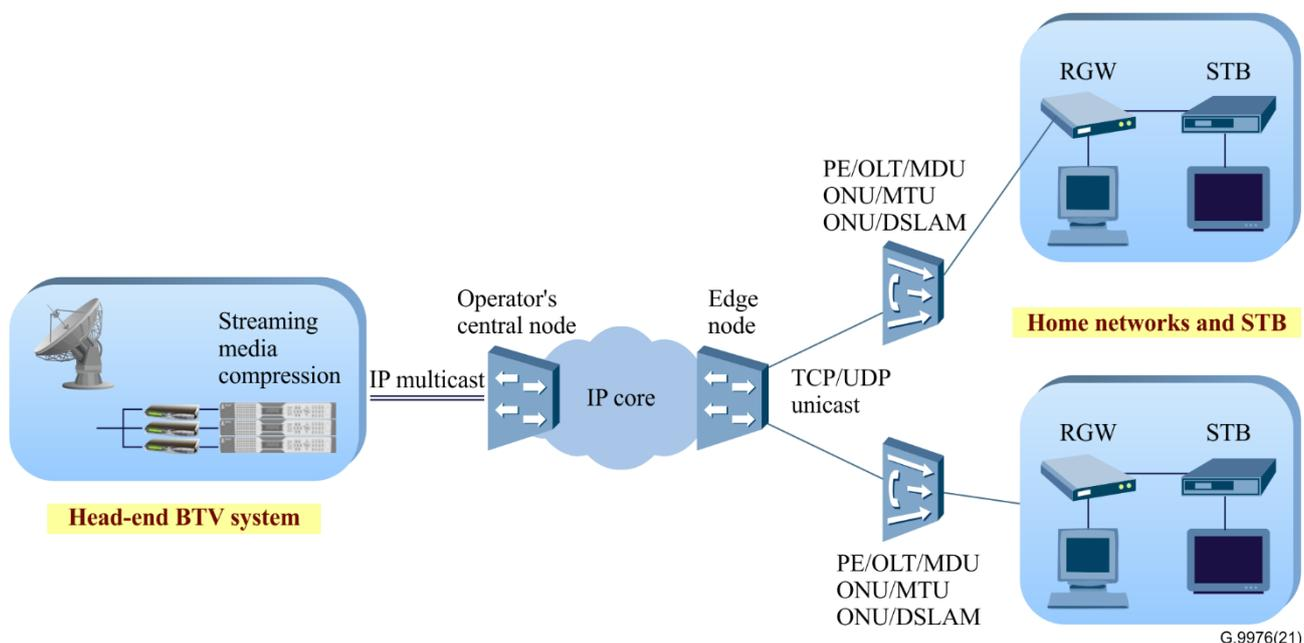
**Figure 6-6 – Schematic architecture diagram of BTV unicast**
