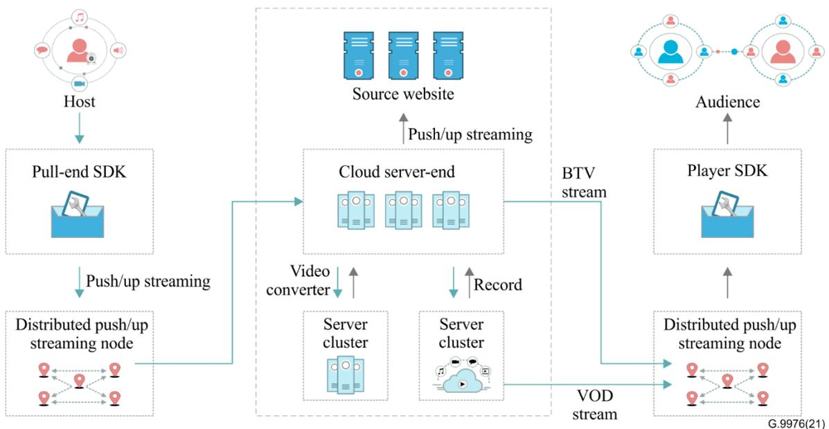
**Figure 6-13 – Schematic diagram of online live broadcasting**
