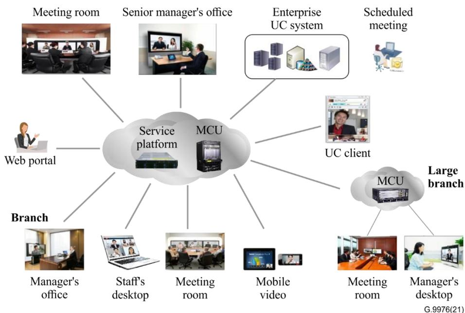
**Figure 6-11 – Schematic diagram of video conferencing for commercial and enterprise users**
