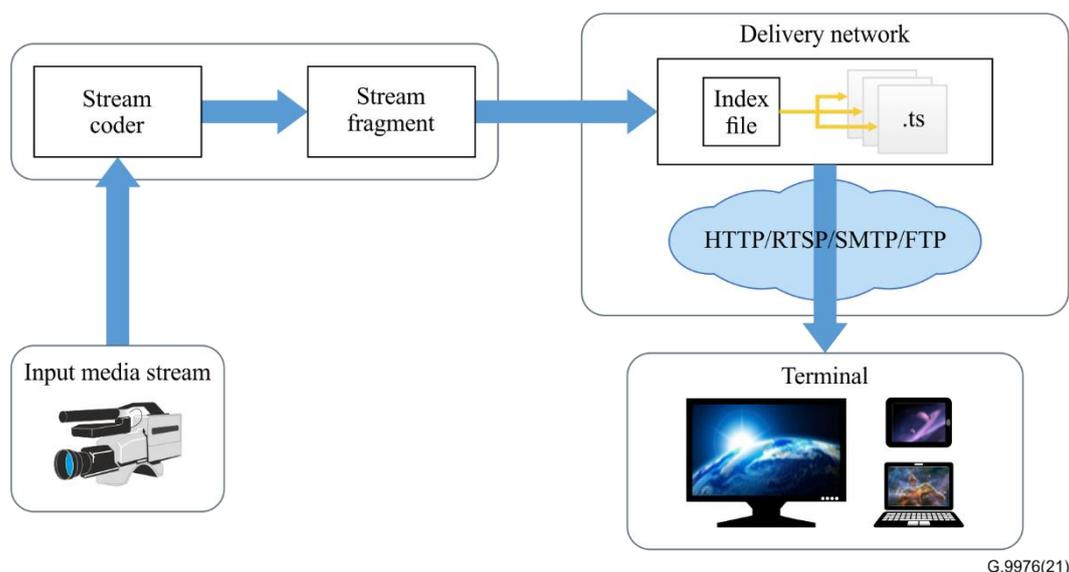
**Figure 6-9 – Example of architecture on VoD mode**
