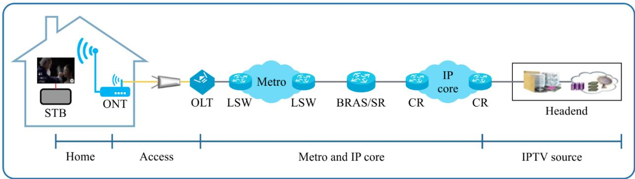
**Figure 8-2 – Decomposition diagram of bearer network for 4K**
