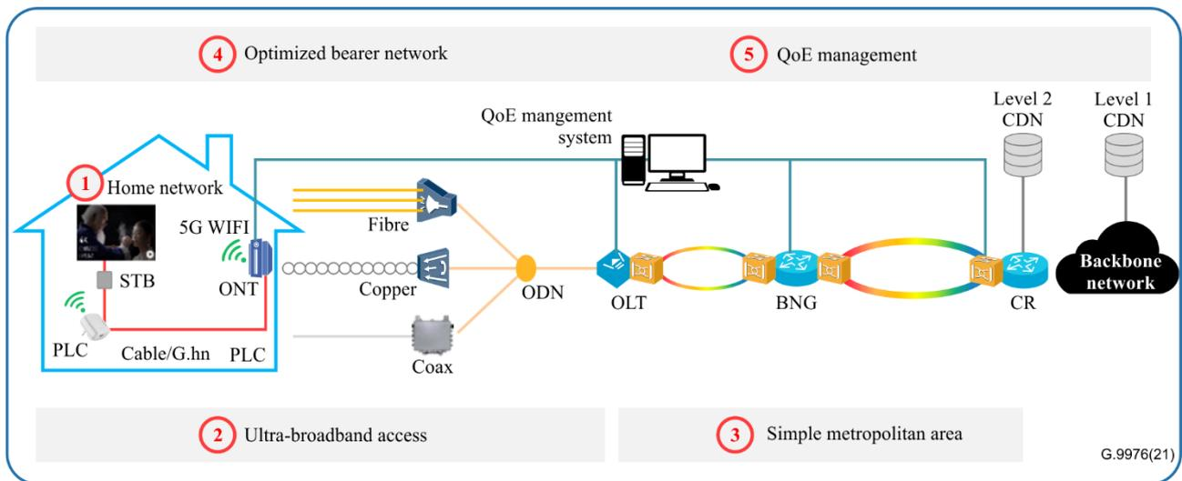
**Figure 8-1 – The target architecture of the video carrier network with the best experience**
