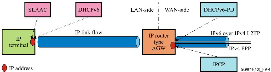
**Figure 9-4 – IPv6 over L2TP over IPv4 to AGW with IPv6 to IP terminal**
