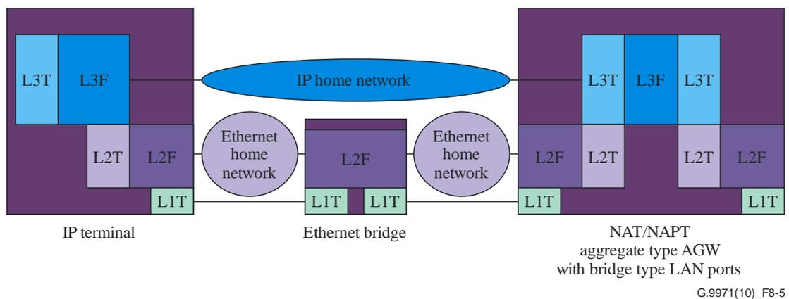
**Figure 8-5 – An example of home network functional architecture**
