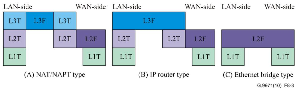
**Figure 8-3 – Functional components of aggregate type AGW**
