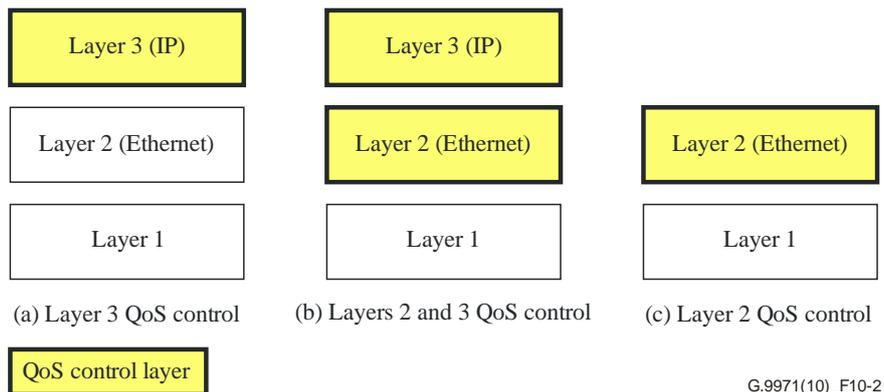
**Figure 10-2 – Three device types for QoS control**
