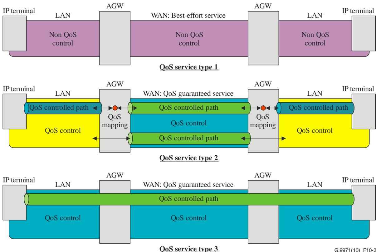
**Figure 10-3 – Relationship between QoS service types and QoS control**
