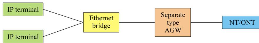
Configuration 1: Each IP terminal is connected to AGW via Ethernet bridge.
