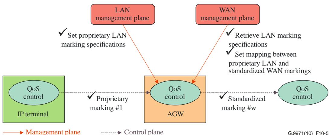
**Figure 10-5 – A realization of hop-by-hop QoS guaranteed services in QoS service type 2**
