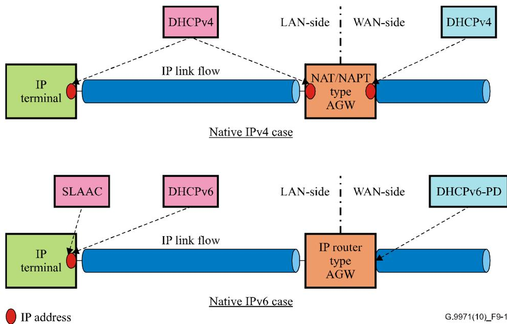
**Figure 9-1 – Native IPv4/IPv6 connection to AGW**
