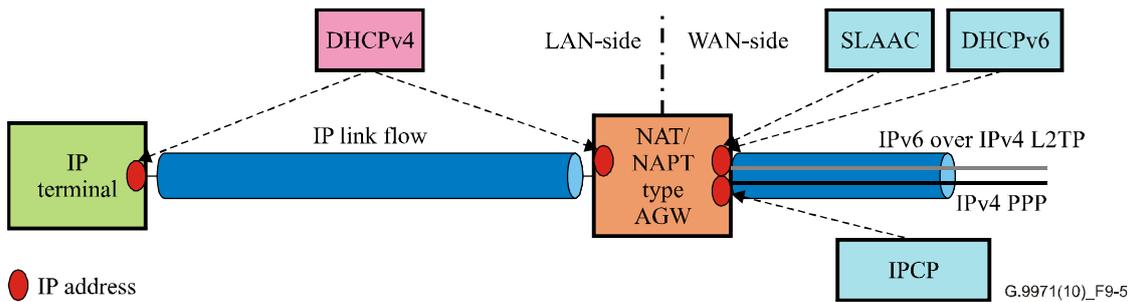
**Figure 9-5 – IPv6 over L2TP over IPv4 to AGW with IPv4 to IP terminal**
