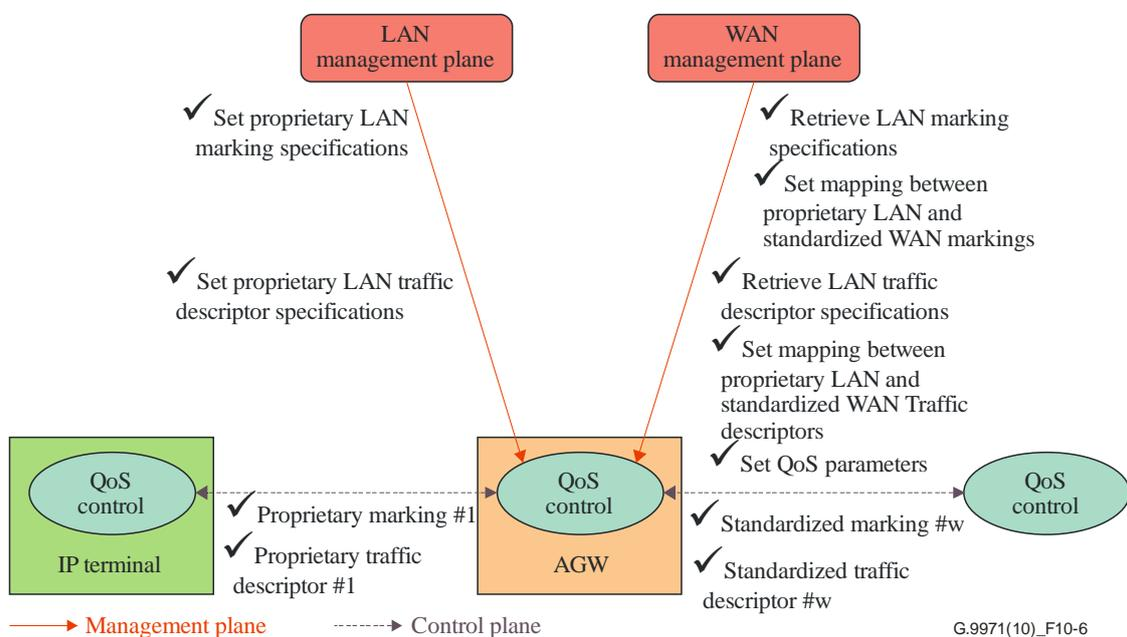
**Figure 10-6 – A realization of end-to-end QoS guaranteed services in QoS service type 2**
