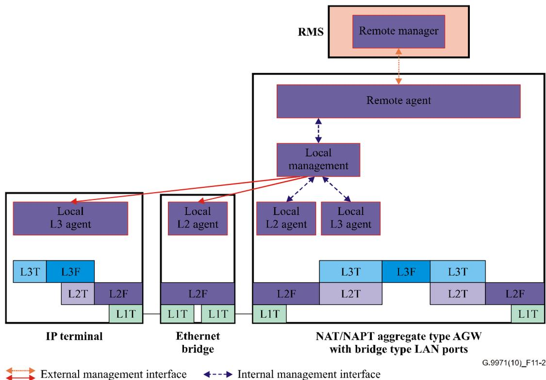
**Figure 11-2 – An example of functional management architecture for Scheme B**
