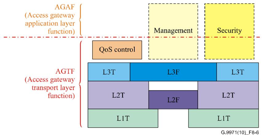
**Figure 8-6 – Functional architecture of separate type AGW**
