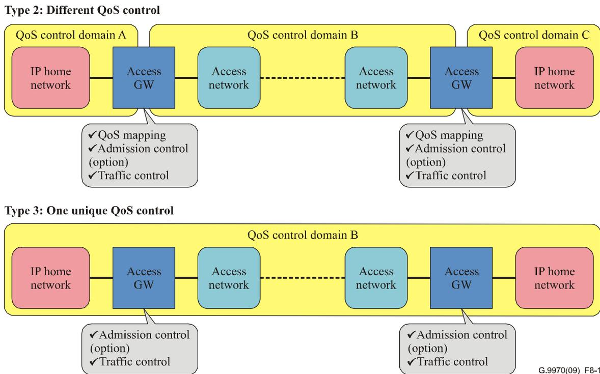
**Figure 8-1 – QoS control for network provider's network and IP home networks**
