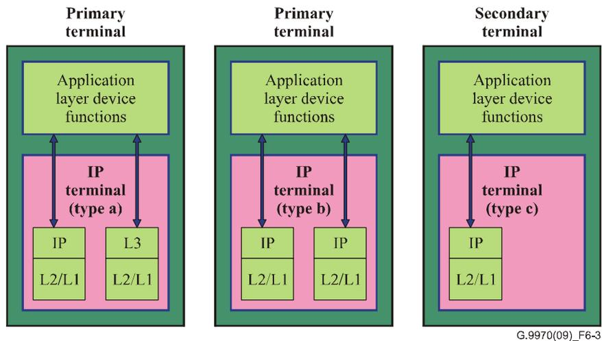
**Figure 6-3 – Three types of IP terminals**
