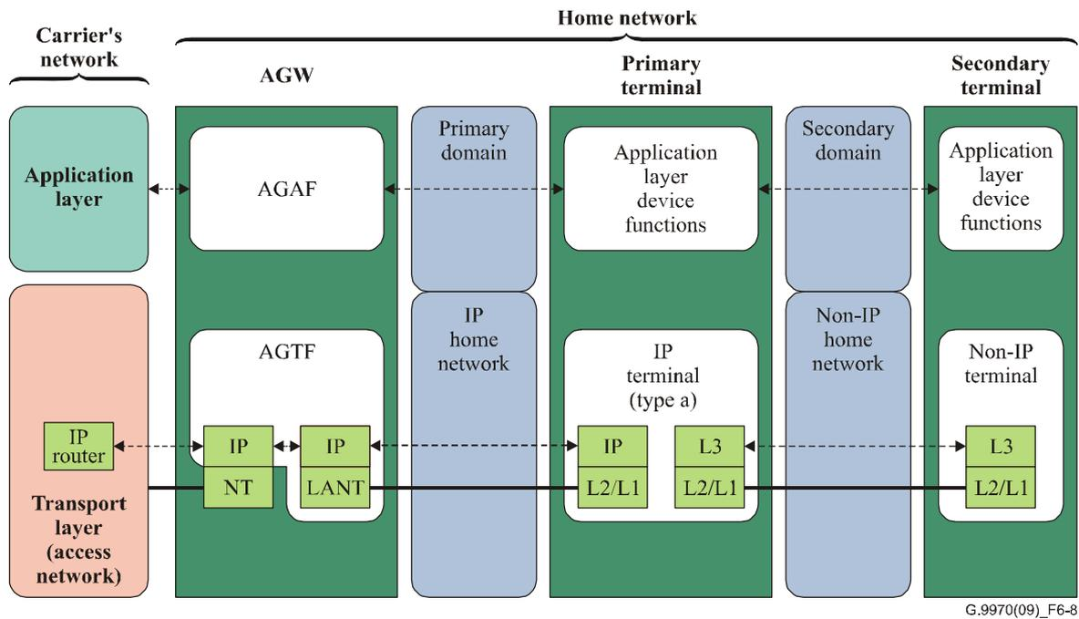
**Figure 6-8 – One physical configuration based on two generic home architectures**
