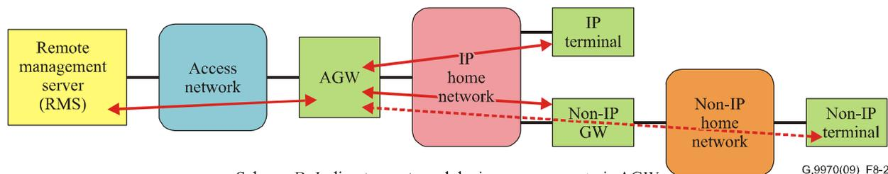
Scheme B: Indirect remote end device management via AGW
