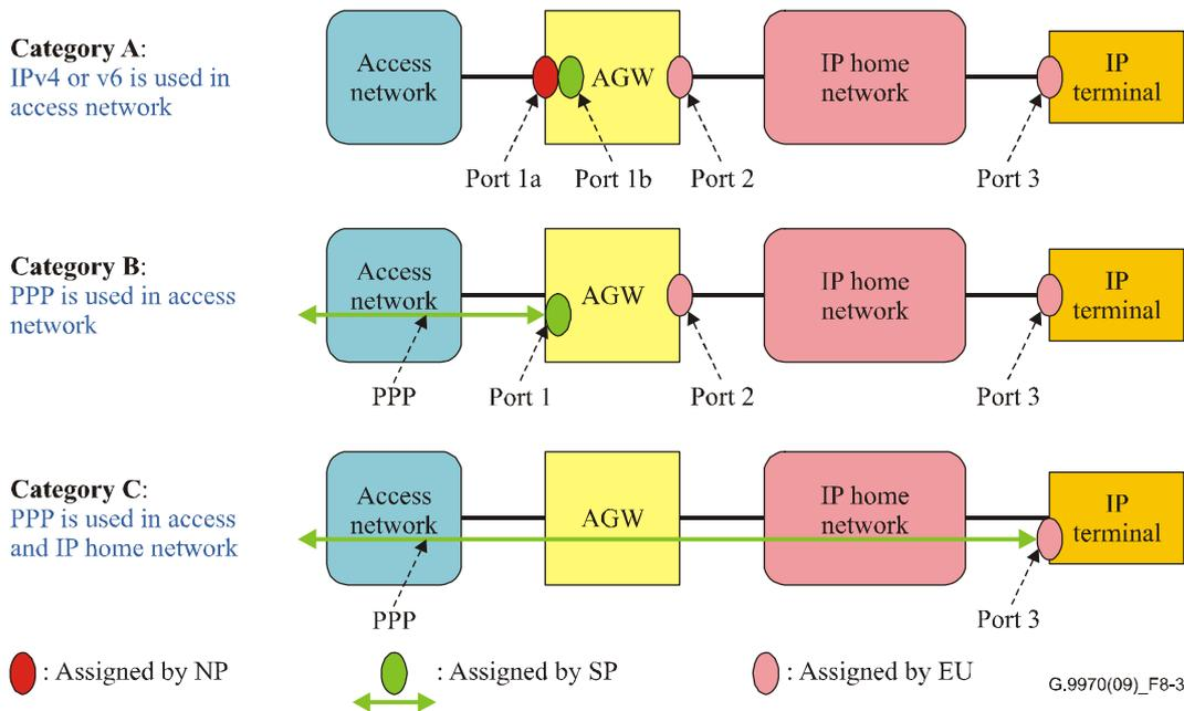
**Figure 8-3 – Examples of IP addressing schemes**
