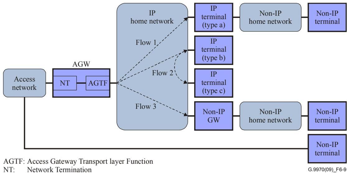
**Figure 6-9 – Three typical flows over the generic home network transport physical architecture**
