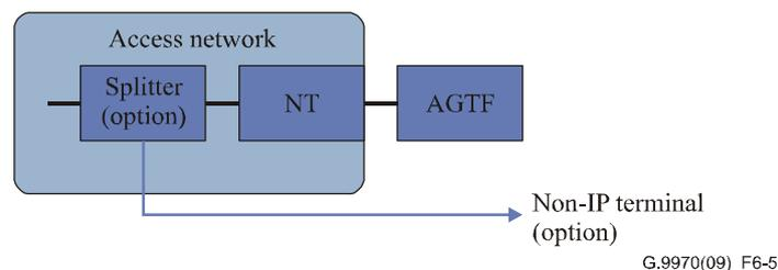
**Figure 6-5 – Access network to support non-IP terminal**
