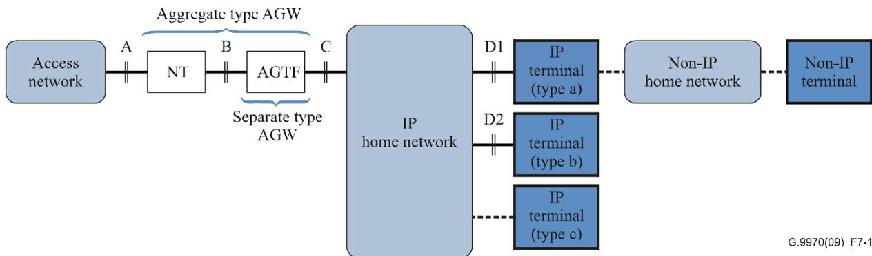
**Figure 7-1 – Possible demarcation points for IP terminals**
