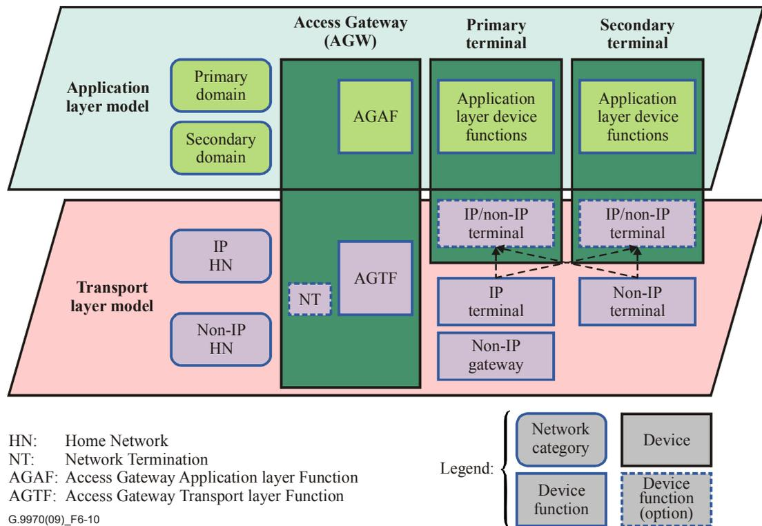
**Figure 6-10 – The conceptual diagram of two layered generic home network models**
