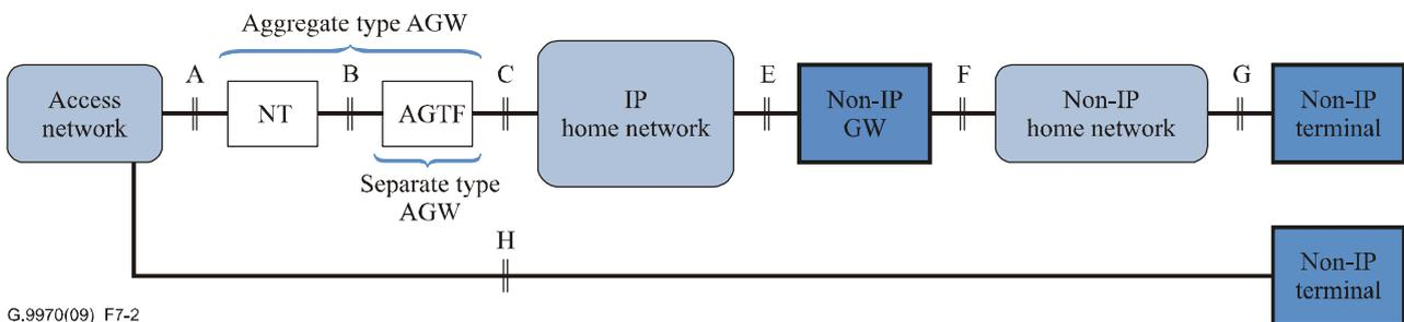
**Figure 7-2 – Possible demarcation points for non-IP terminals**
