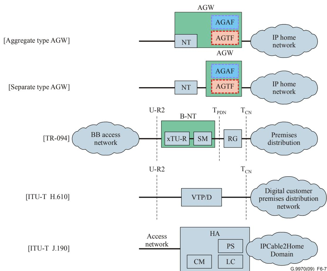
**Figure 6-7 – The configuration of AGW in comparison with some documents**
