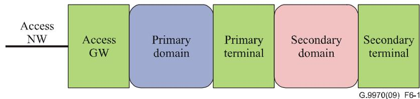
**Figure 6-1 – Application model of the home network**
