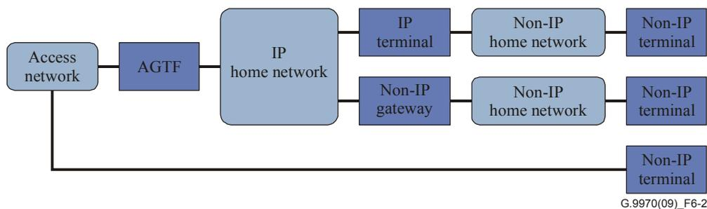
**Figure 6-2 – Generic home network functional architecture for the transport layer**
