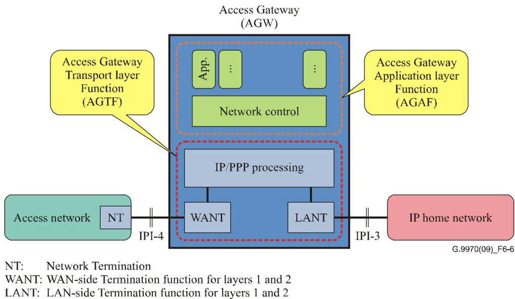
**Figure 6-6 – Decomposition of access gateway**
