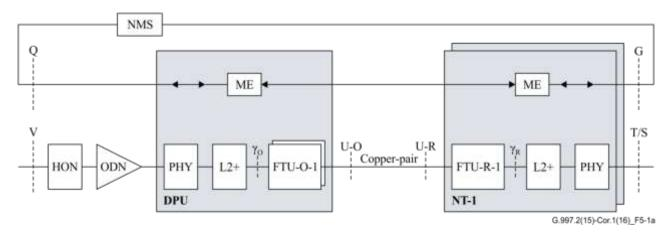
Figure 5-1a – Reference model of traditional AN deployment (shown for line 1 in all N lines (N≥1) connected to an AN)
