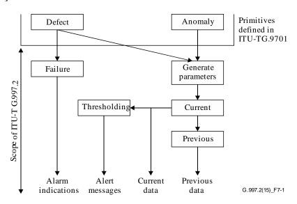
Figure 7-1 – In-service performance monitoring process
