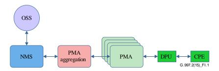
Figure I.1 – High-level PMA architecture (source: Broadband Forum)
