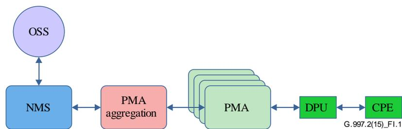
**Figure I.1 – High-level PMA architecture (source: Broadband Forum)**
