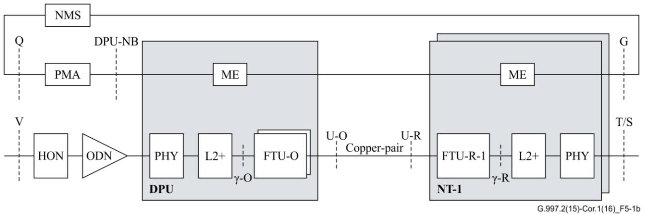
**Figure 5-1b – Reference model of FTTh deployment with PMA and DPU
