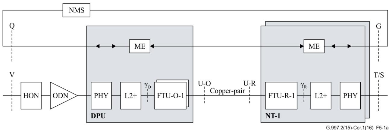
**Figure 5-1a – Reference model of traditional AN deployment
