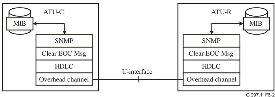
**Figure 6-2 – OAM communication channel layers for message-oriented clear EOC**
