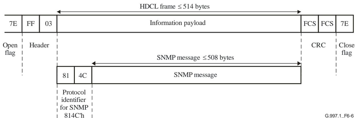
Figure 6-6 – OAM communication channel protocol over the U-interface
