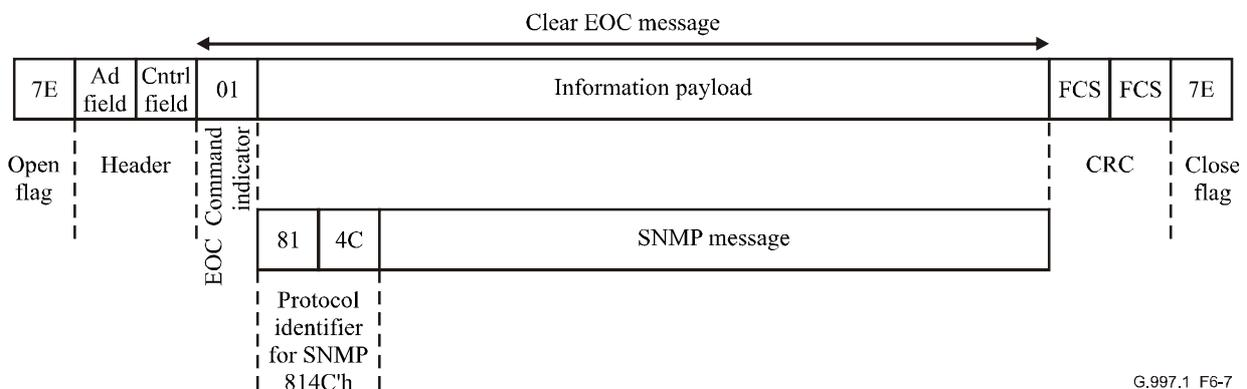
**Figure 6-7/G.997.1 – OAM communication channel protocol over the U-interface**
