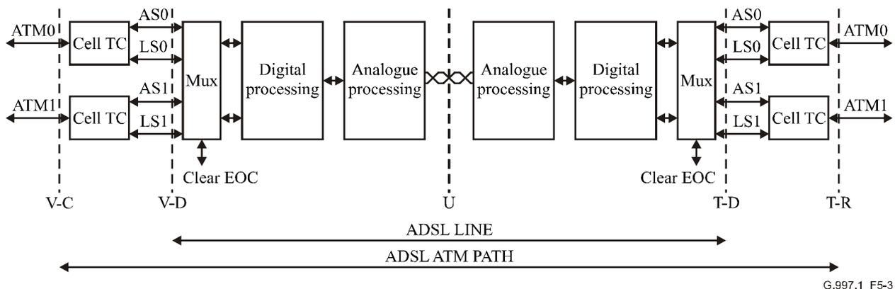
**Figure 5-3/G.997.1 – ADSL LINE and ADSL ATM PATH definition**
