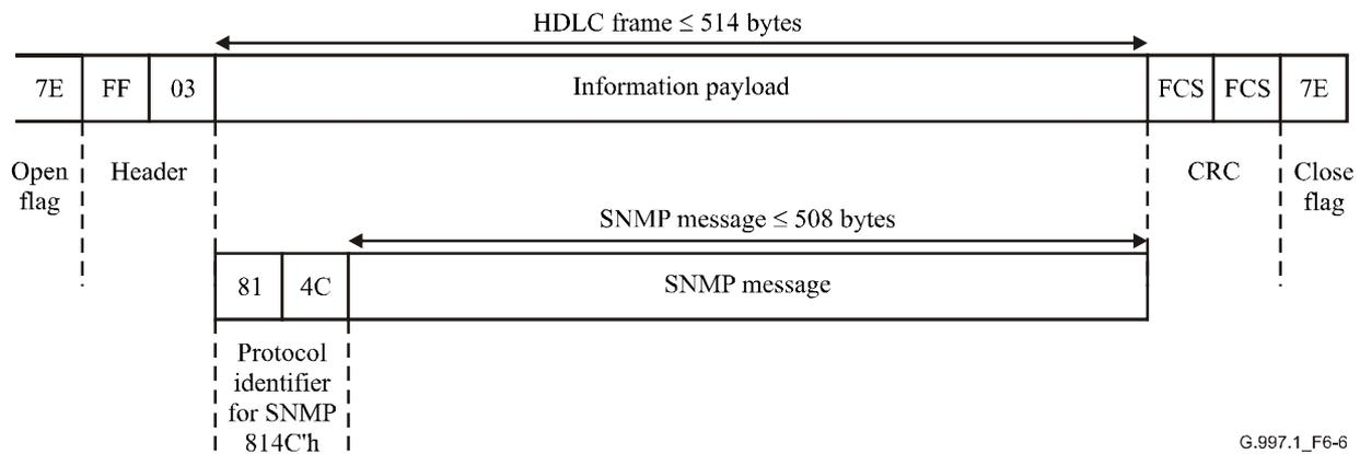
**Figure 6-6/G.997.1 – OAM communication channel protocol over the U-Interface**
