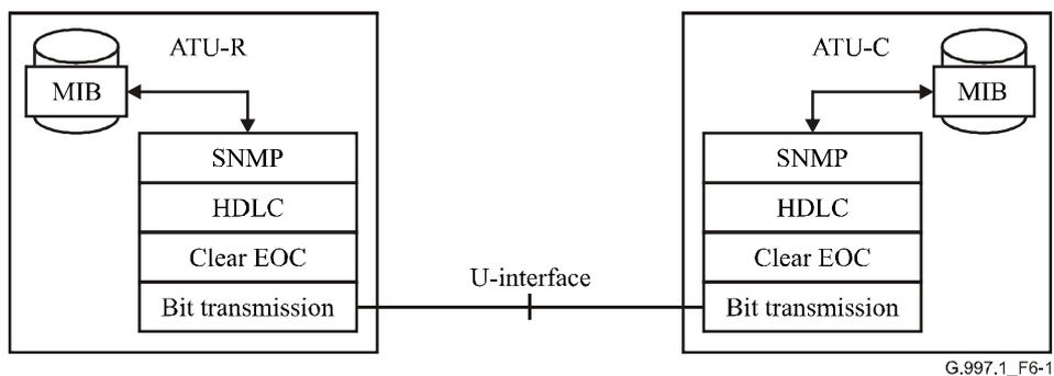
**Figure 6-1/G.997.1 – OAM communication channel layers for bit-oriented clear EOC**
