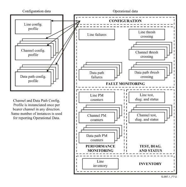
Figure 7-2/G.997.1 – Overview of the MIB elements provided for each line
