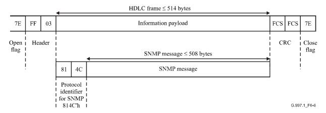
Figure 6-6/G.997.1 – OAM communication channel protocol over the U-Interface
