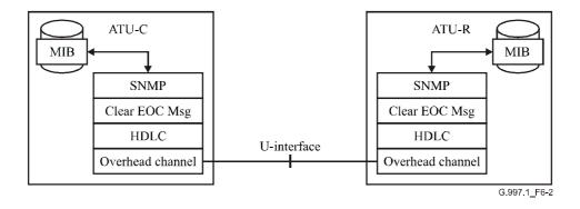
Figure 6-2/G.997.1 – OAM communication channel layers for message-oriented clear EOC
