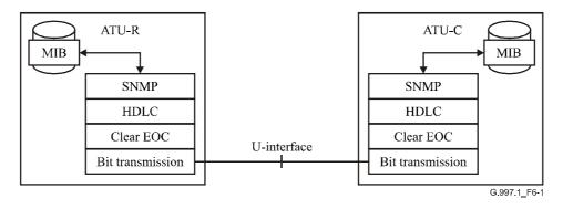
Figure 6-1/G.997.1 – OAM communication channel layers for bit-oriented clear EOC
