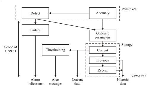
Figure 7-1/G.997.1 – In-service performance monitoring process
