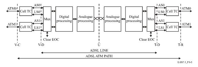
Figure 5-3/G.997.1 – ADSL LINE and ADSL ATM PATH definition
