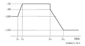
Figure 6-4 – Limit PSD mask of baseband coax (Profile 1 OFBs)
