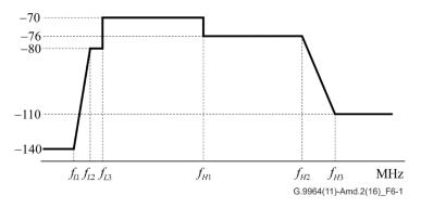
Figure 6-1 – Limit PSD mask for transmission over telephone lines (amateur radio-band notches are not shown)
