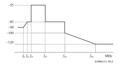
Figure 6-2 – Limit PSD mask for baseband transmission over power lines for 25 MHz-PB, 50 MHz-PB and 100 MHz-PB bandplans <u>OFBs</u> (amateur radio-band notches are not shown)
