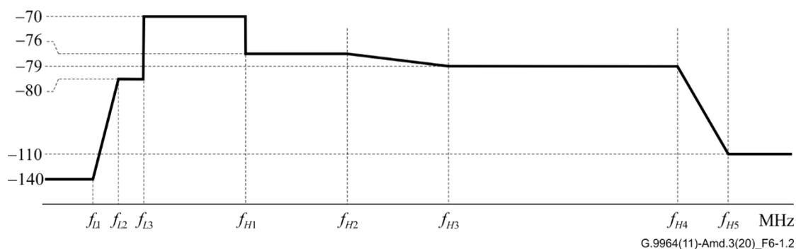
**Figure 6-1.2 – Limit PSD mask for transmission over telephone lines
