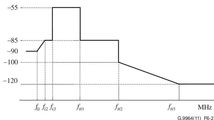
**Figure 6-2 – Limit PSD mask for baseband transmission over power lines for 25 MHz-PB, 50 MHz-PB and 100 MHz-PB bandplans-OFBs (amateur radio-band notches are not shown)**
