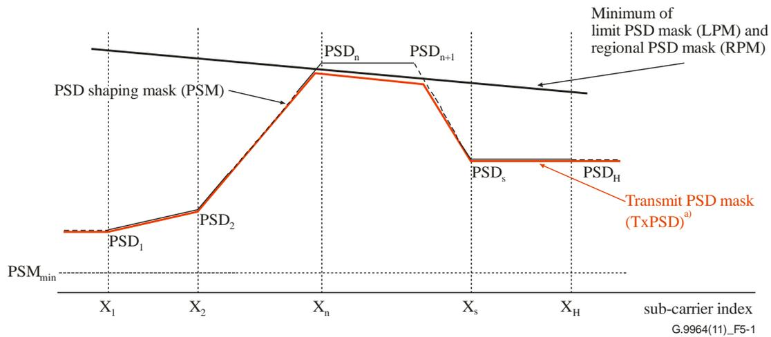
**Figure 5-1 – Construction of transmit PSD mask**
