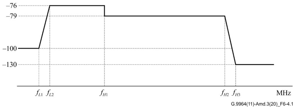
**Figure 6-4.1 – Limit PSD mask of coax (Profile 2 OFBs)**
