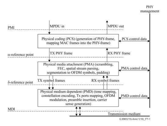
Figure 7-1 – PHY functional model of the MIMO transceiver
