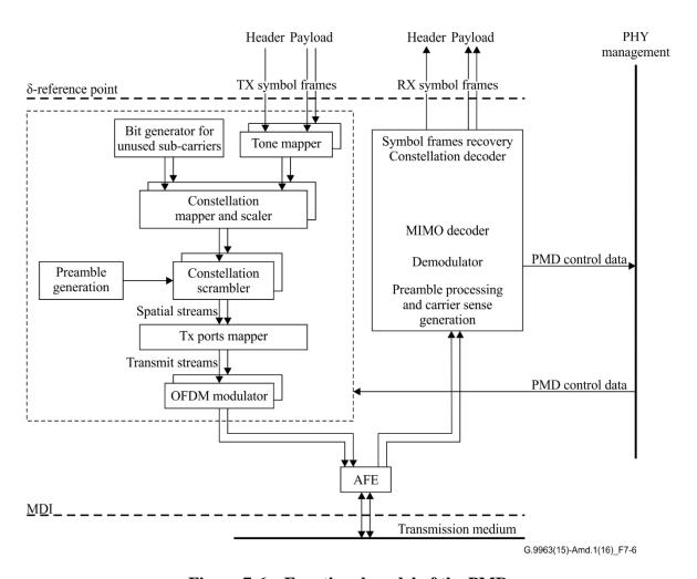
Figure 7-6 – Functional model of the PMD
