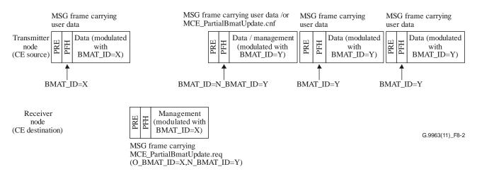
Figure 8-2 – Example of partial BMAT update using management message
