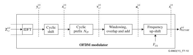
Figure 7-10 – Functional model of the OFDM modulator
