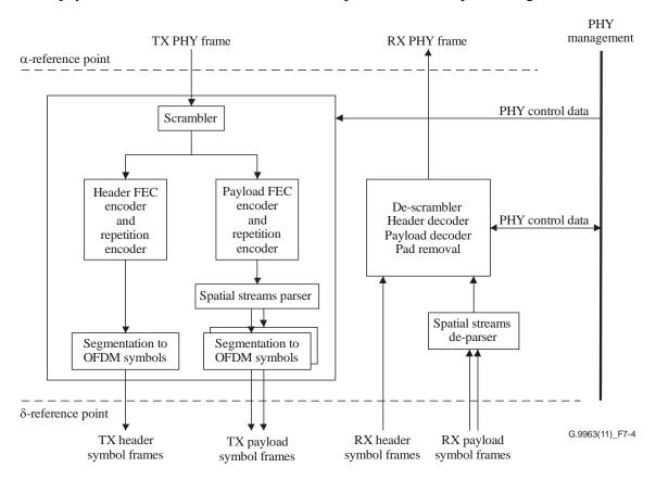
Figure 7-4 – Functional model of PMA
