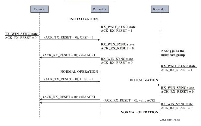
Figure 8-53 – Initialization of the acknowledgement protocol for multicast transmission
