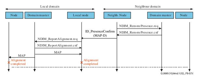
Figure 8-57.6 – Protocol diagram for local MAC cycle alignment
