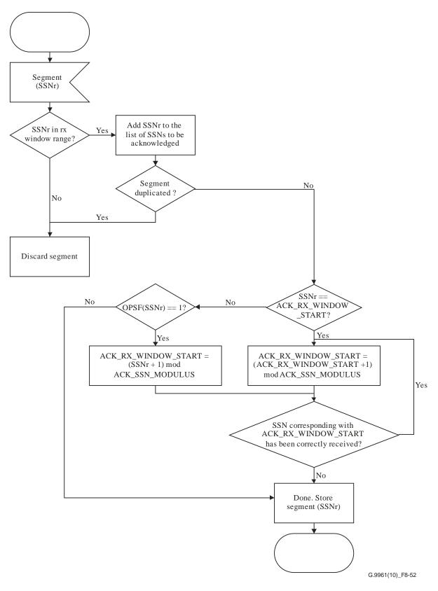
Figure 8-52 – Receiver SSN processing
