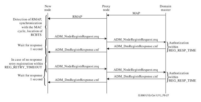
Figure 8-27 – Protocol diagram describing node registration via proxy
