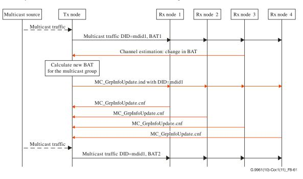
Figure 8-61 – Example of maintenance of PHY multicast binding information
