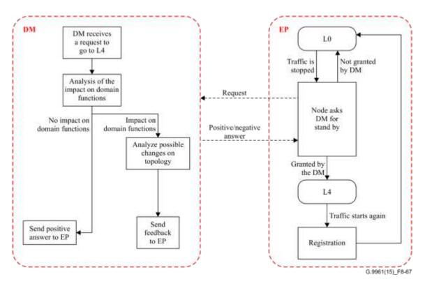
Figure 8-67 – Operation in L4 power saving mode
