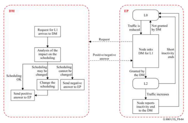
Figure 8-64 – Operation in L1 power saving mode
