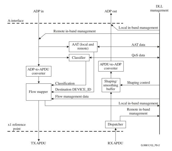
Figure 8-2 – Functional model of APC
