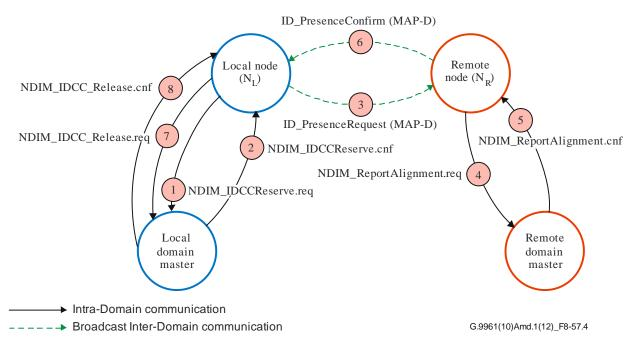
Figure 8-57.4 – Remote MAC cycle alignment procedure
