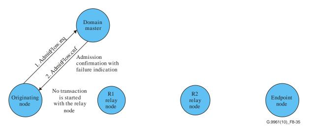
Figure 8-35 – Example of a tunnel establishment failure scenario due to the domain master rejecting the admission request
