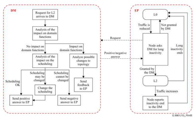
Figure 8-65 – Operation in L2 power saving mode
