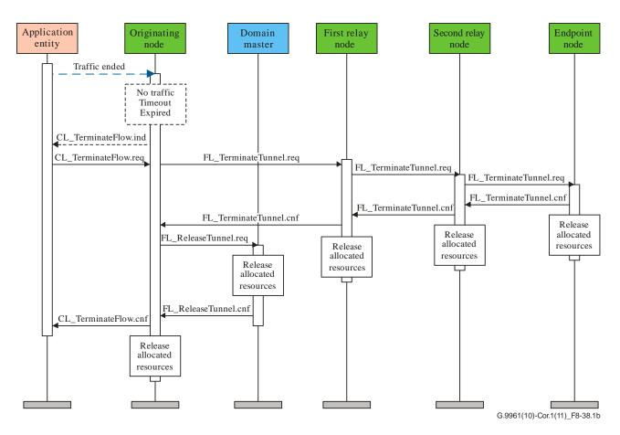
Figure 8-38.1b – MSC of normal termination of a tunnel
