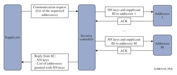
Figure 9-6 – Procedure for NN key generation for unicast (M=1) and multicast (M > 1)
