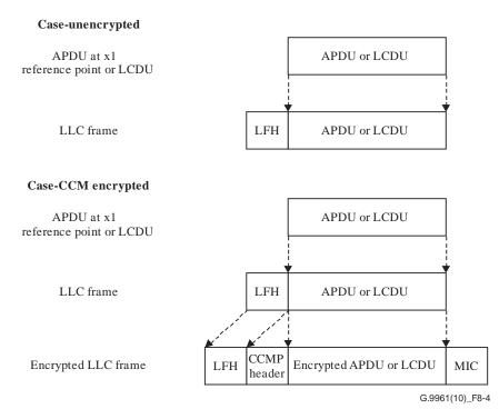
Figure 8-4 – LLC frame format (unencrypted and encrypted)
