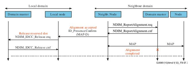
Figure 8-57.7 – Protocol diagram for remote MAC cycle alignment
