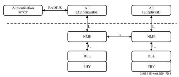
Figure D.1 – IEEE 802.1x port-based network access control over a domain
