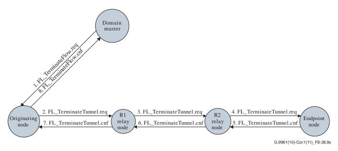
Figure 8-38.9a – Domain master triggers tunnel termination
