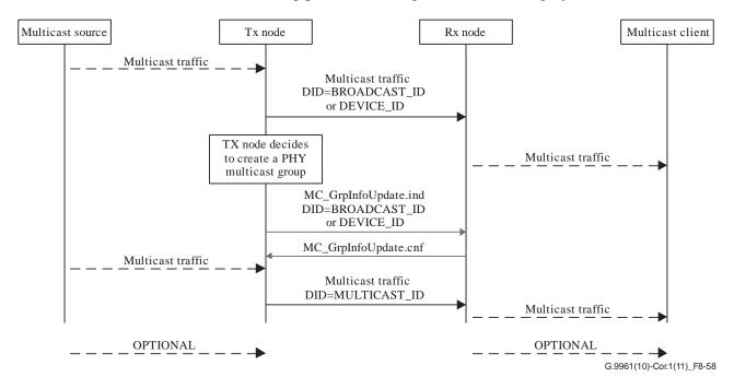
Figure 8-58 – Example of initializing a PHY multicast group
