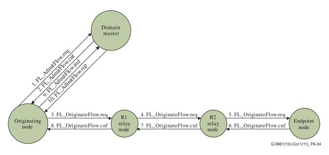
Figure 8-34 - Example of a successful tunnel establishment via two relay nodes
