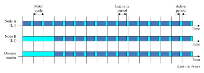
Figure 8-63.1 – Example of domain with nodes in L1 power saving mode
