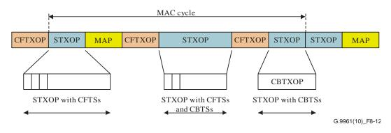
Figure 8-12 – Example of a MAC cycle structure
