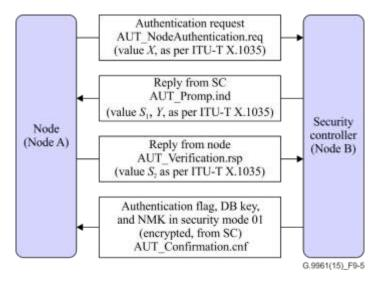
Figure 9-5 – PAK handshake procedure
