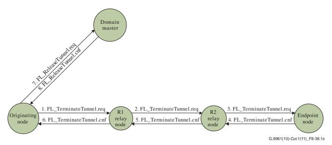
Figure 8-38.1a – Normal tunnel termination
