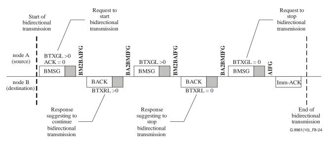
Figure 8-24 – Example of bidirectional transmission (invited by the originating node)
