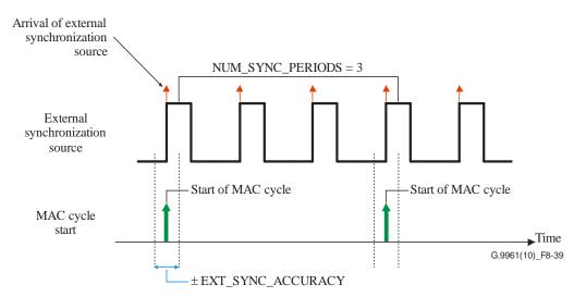
Figure 8-39 – Example of synchronization of MAC cycle to a periodic external source
