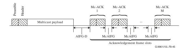
Figure 8-45 – Multicast acknowledgment without NACK signalling
