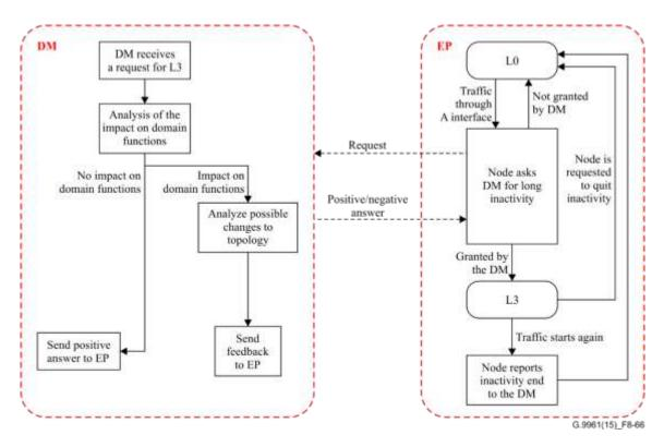
Figure 8-66 – Operation in L3 power saving mode
