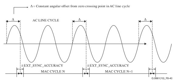
Figure 8-40 – Relationship between the AC line cycle and the MAC cycle when the duration of the MAC cycle is 2 AC cycles
