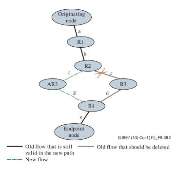
Figure 8-38.3 – Tunnel renewal due to a broken link
