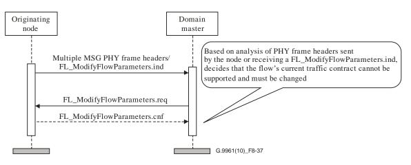
**Figure 8-37 – Flow parameters modification example**
