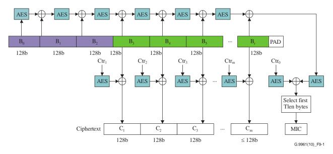
Figure 9-1 – Functional diagram of CCM encryption and message-authentication
