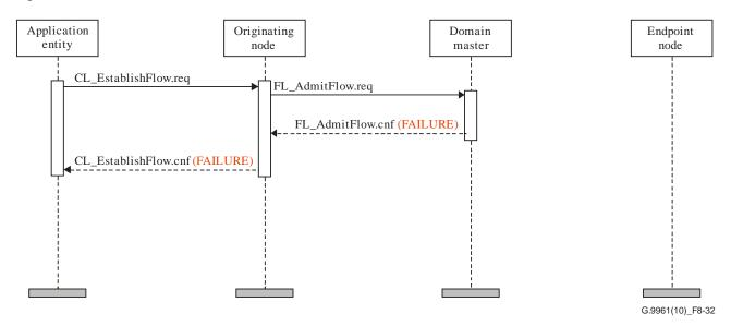
Figure 8-32 – Failure in flow establishment due to rejection by the domain master
