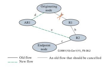
Figure 8-38.2 – Tunnel renewal due to a broken link: case 1
