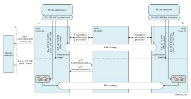
Figure B.2 – External authentication procedure via proxy for smart grid
