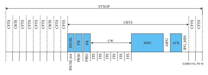
Figure 8-16 – An example of transmission in a CBTS
