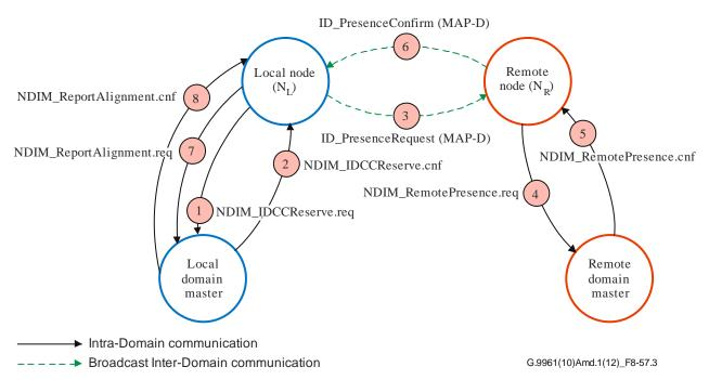
Figure 8-57.3 – Local MAC cycle alignment procedure
