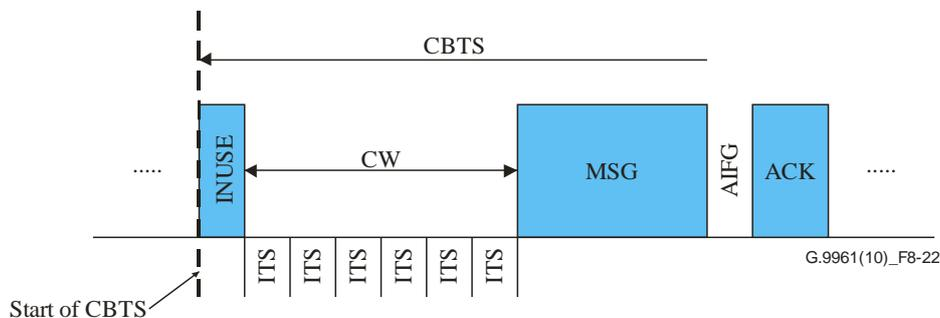
**Figure 8-22 – Example of transmission in a CBTS with no PR signals (INUSE signal is used, RTS/CTS is not used)**
