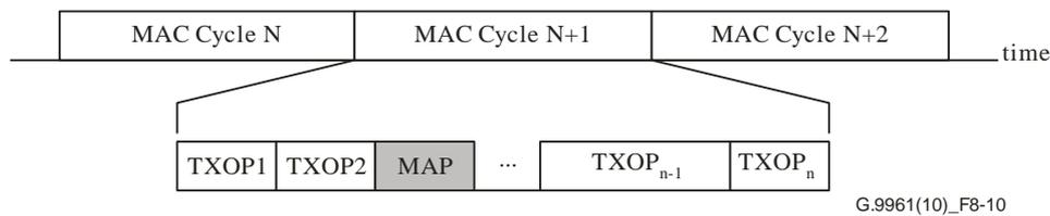
**Figure 8-10 – Illustration of MAP controlled medium access**
