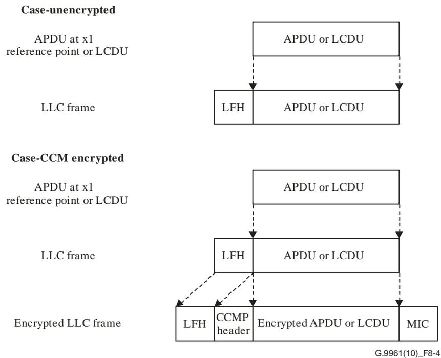
**Figure 8-4 – LLC frame format (unencrypted and encrypted)**
