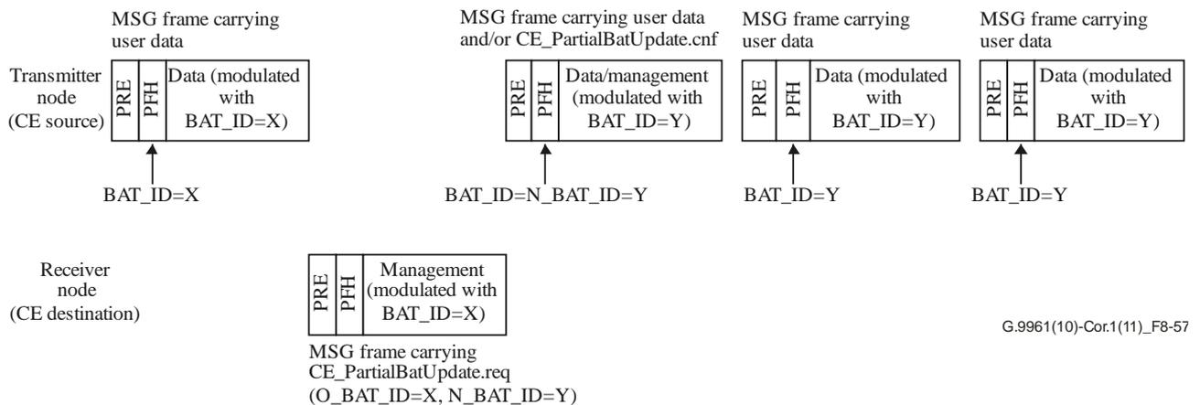
**Figure 8-57 – Example of partial BAT update using management message**
