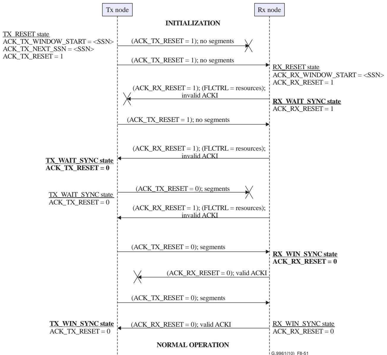
**Figure 8-51 – Detailed initialization of the Acknowledgement protocol**
