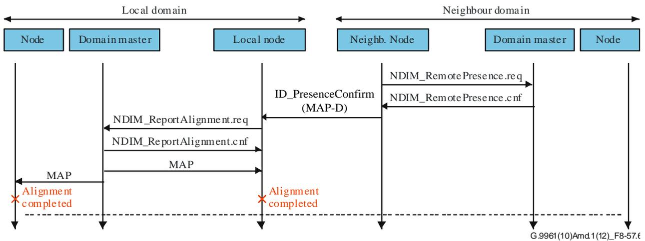
**Figure 8-57.6 – Protocol diagram for local MAC cycle alignment**
