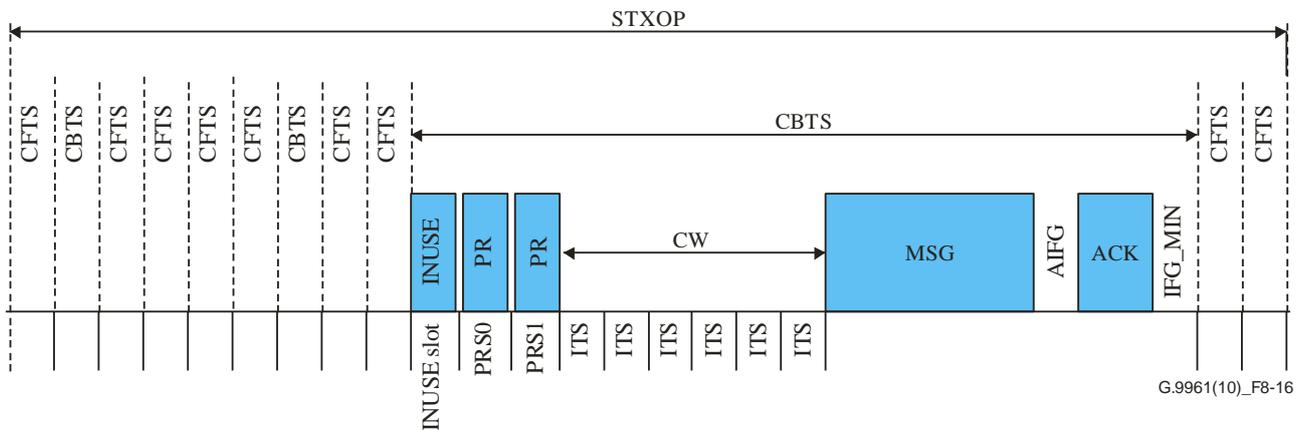
**Figure 8-16 – An example of transmission in a CBTS**
