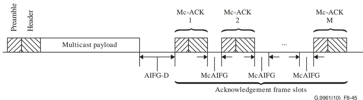
**Figure 8-45 – Multicast acknowledgment without NACK signalling**
