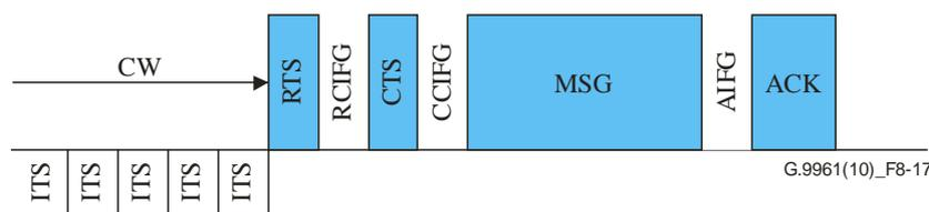
**Figure 8-17 – Use of RTS/CTS signalling in a CBTS**
