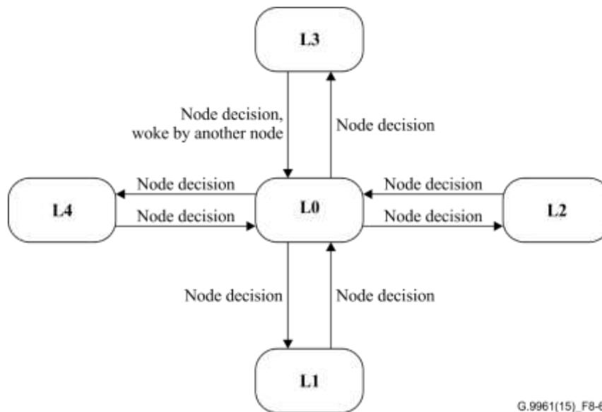
**Figure 8-63 – Allowed transitions for node power saving modes**
