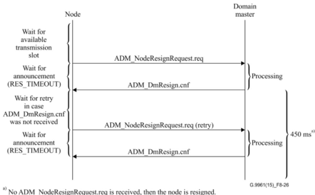
**Figure 8-26 – Protocol diagram describing node resignation**
