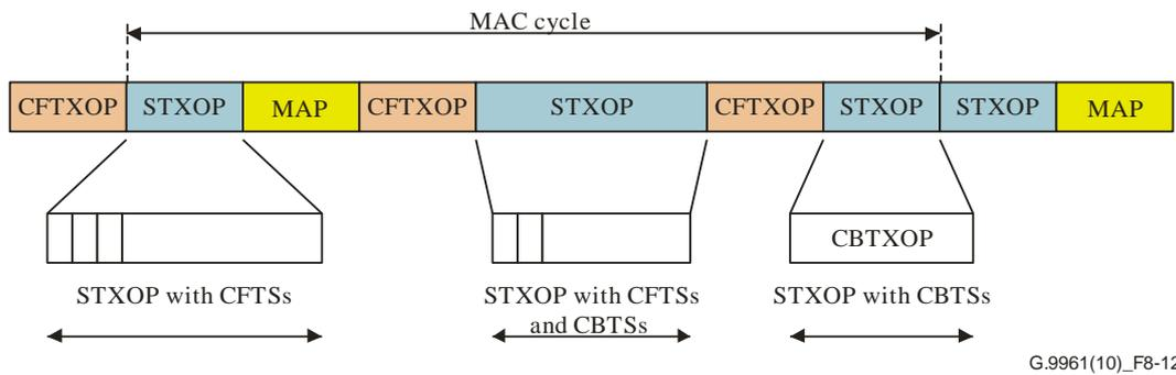
**Figure 8-12 – Example of a MAC cycle structure**
