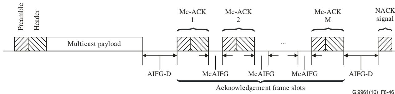
**Figure 8-46 – Multicast acknowledgment with NACK signalling**
