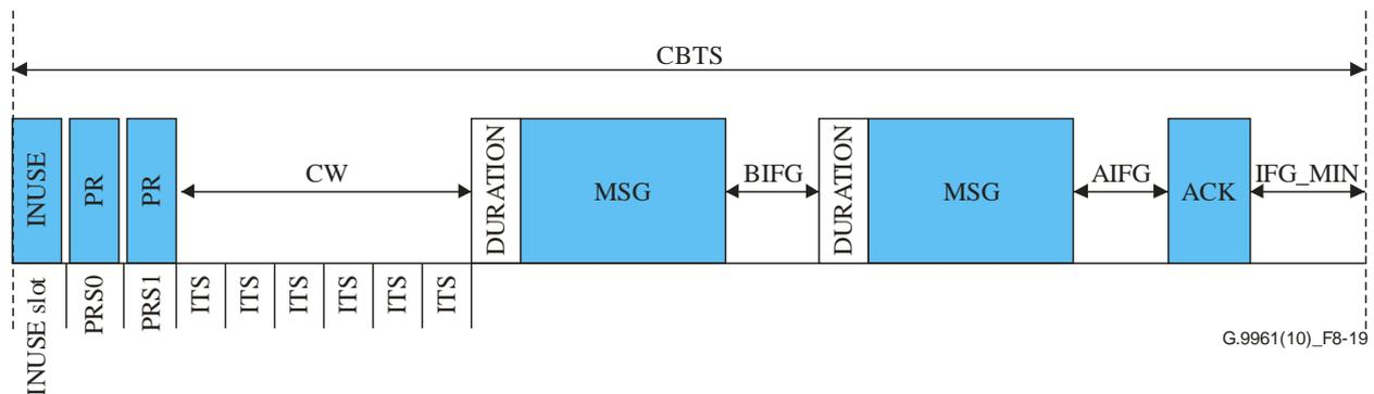
**Figure 8-19 – Example of duration-based CBTS closure**
