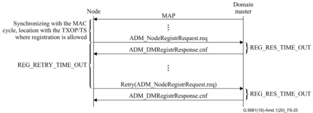
**Figure 8-25 – Protocol diagram describing node registration**
