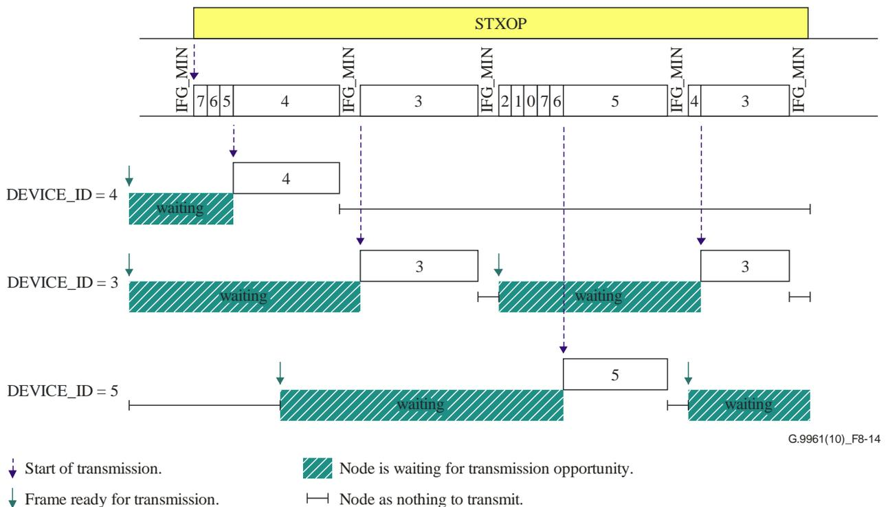
**Figure 8-14 – Sequential TS assignment rule example**
