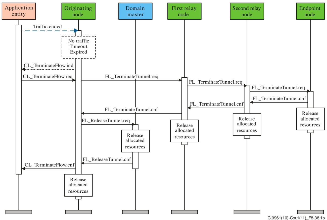
**Figure 8-38.1b – MSC of normal termination of a tunnel**
