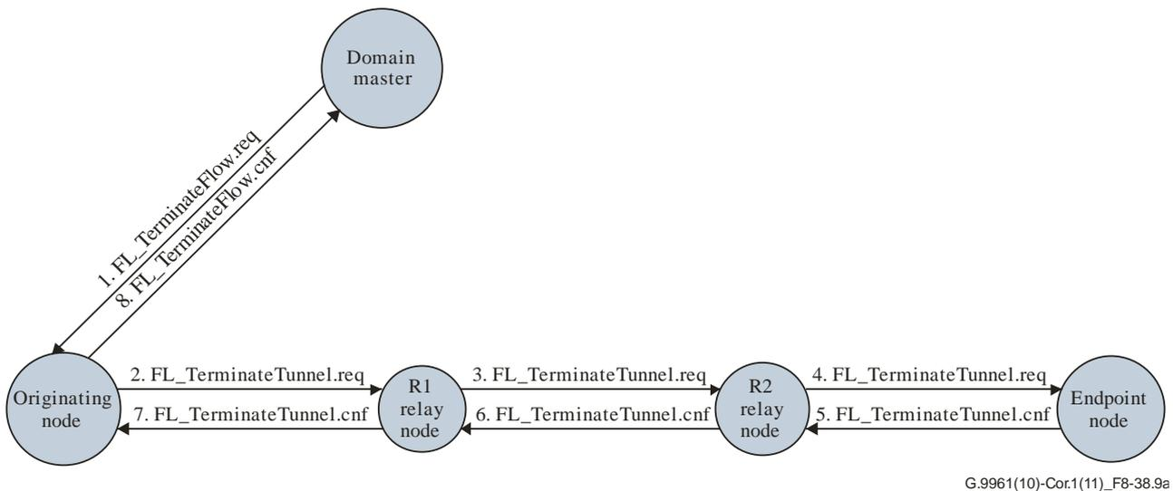
**Figure 8-38.9a – Domain master triggers tunnel termination**
