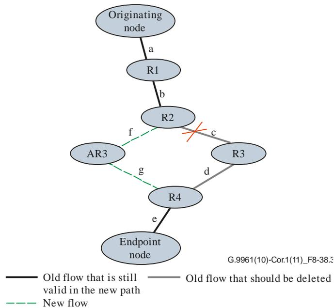
**Figure 8-38.3 – Tunnel renewal due to a broken link**
