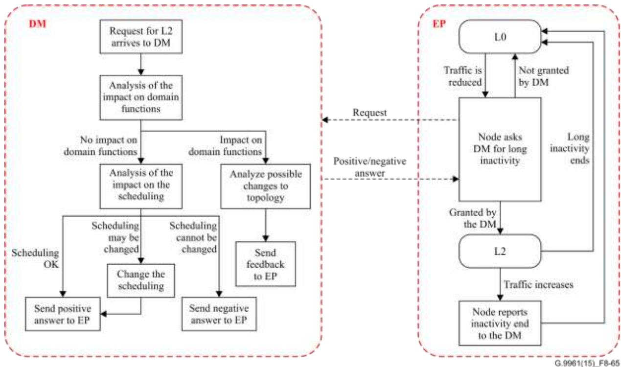
**Figure 8-65 – Operation in L2 power saving mode**
