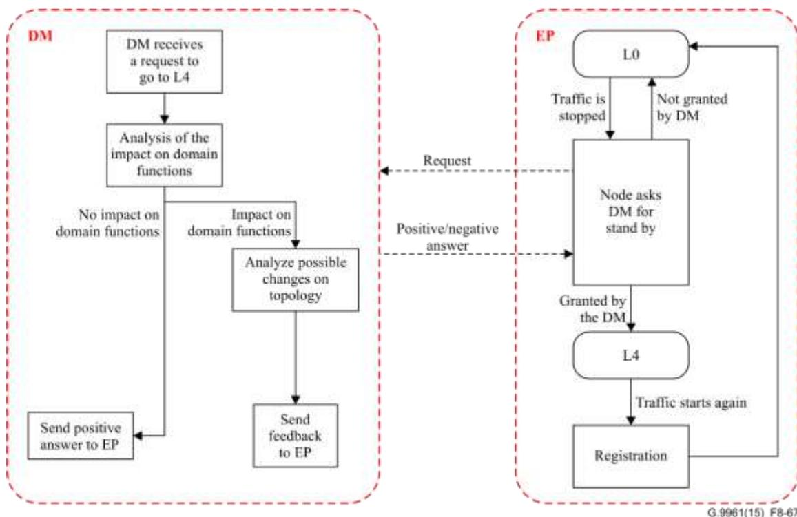
**Figure 8-67 – Operation in L4 power saving mode**
