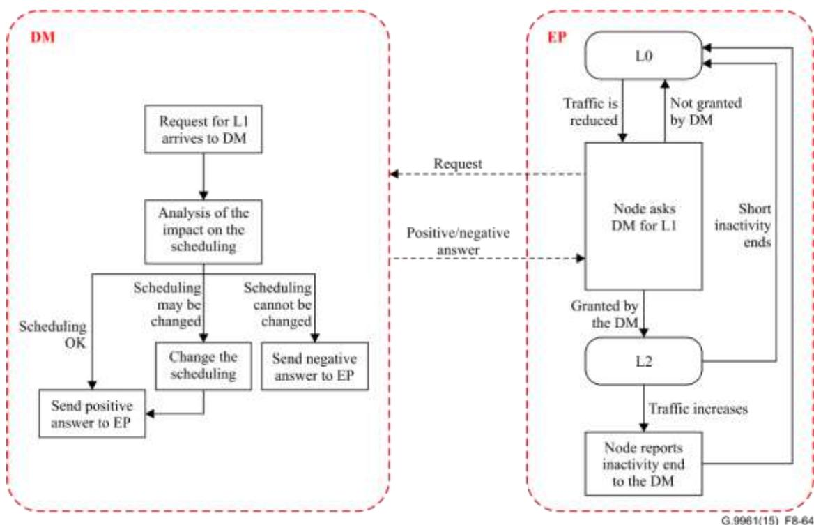
**Figure 8-64 – Operation in L1 power saving mode**
