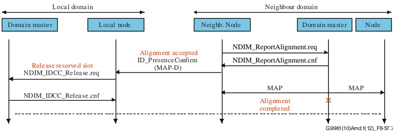
**Figure 8-57.7 – Protocol diagram for remote MAC cycle alignment**
