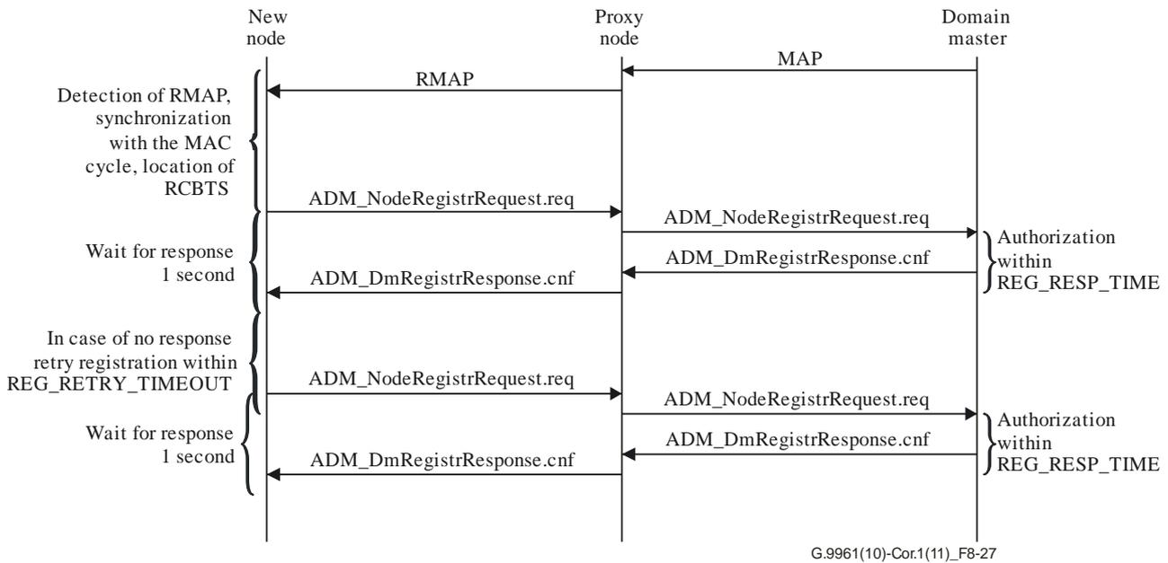
**Figure 8-27 – Protocol diagram describing node registration via proxy**
