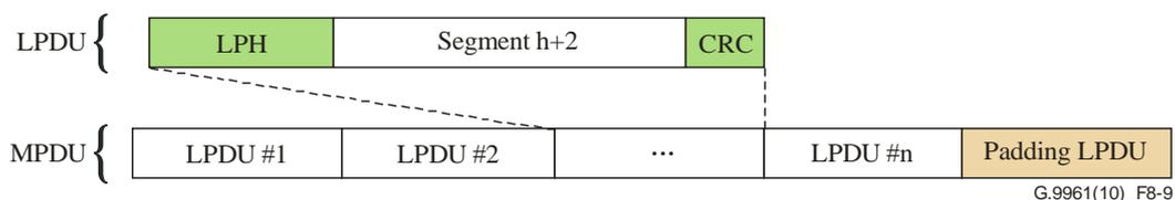
**Figure 8-9 – Assembling of an MPDU from LPDUs**
