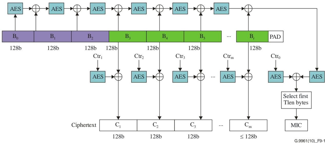
**Figure 9-1 – Functional diagram of CCM encryption and message-authentication**
