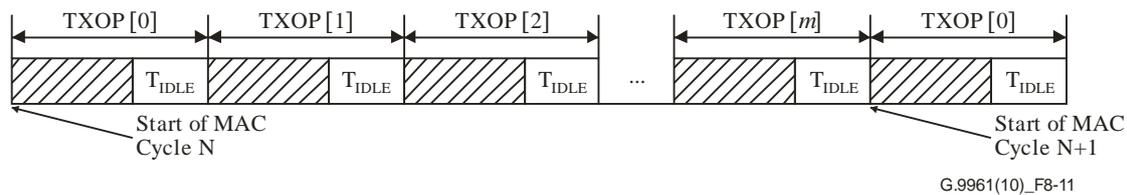
**Figure 8-11 – IFG placement in the MAC cycle**
