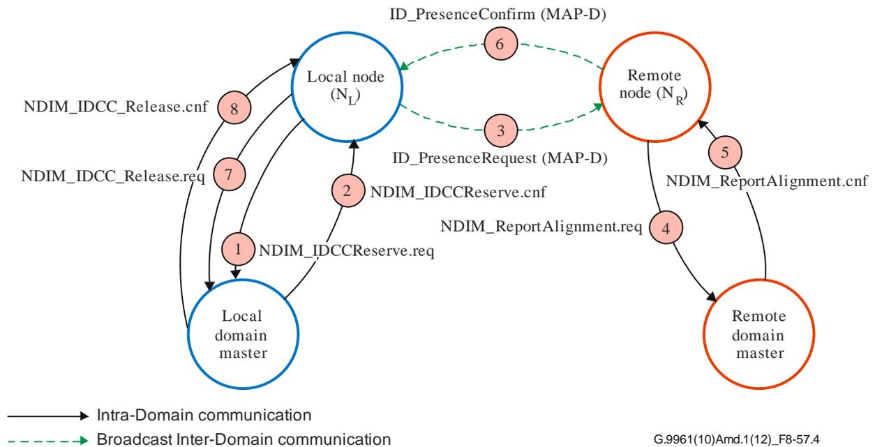
**Figure 8-57.4 – Remote MAC cycle alignment procedure**
