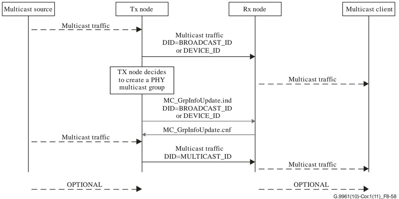
**Figure 8-58 – Example of initializing a PHY multicast group**
