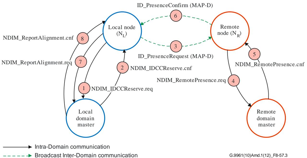
**Figure 8-57.3 – Local MAC cycle alignment procedure**
