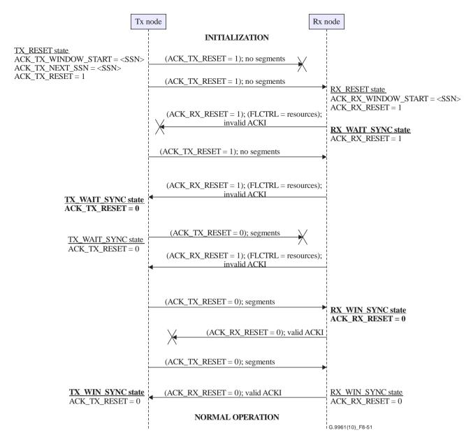
Figure 8-51 – Detailed initialization of the Acknowledgement protocol
