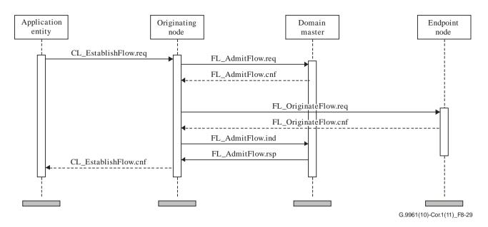
Figure 8-29 – Successful flow establishment
