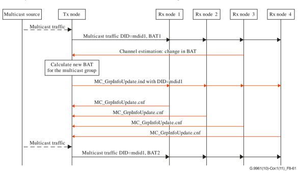
Figure 8-61 – Example of maintenance of PHY multicast binding information
