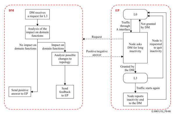
Figure 8-66 – Operation in L3 power saving mode
