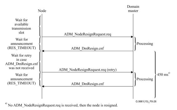
Figure 8-26 – Protocol diagram describing node resignation
