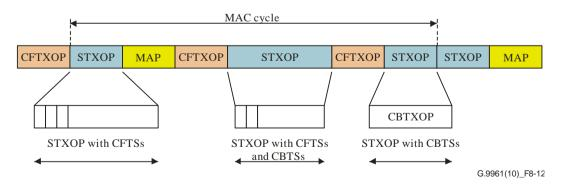
Figure 8-12 – Example of a MAC cycle structure
