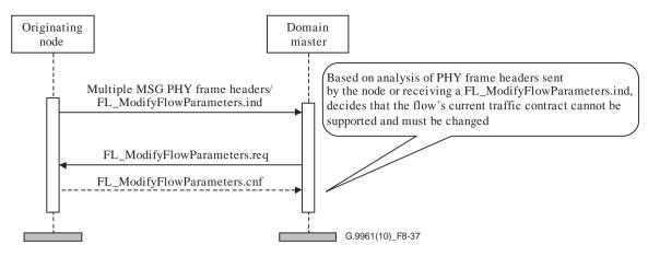
**Figure 8-37 – Flow parameters modification example**
