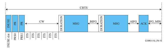
Figure 8-19 – Example of duration-based CBTS closure
