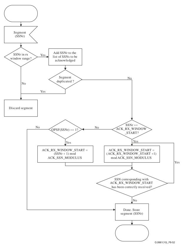
Figure 8-52 – Receiver SSN processing
