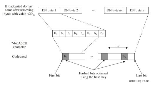
Figure 8-42 – Generation of a DNI from the domain name
