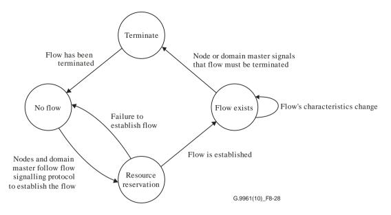
Figure 8-28 - Lifecycle of a flow
