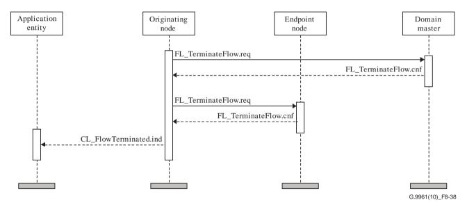
Figure 8-38 – MSC showing an example of how a flow can be terminated
