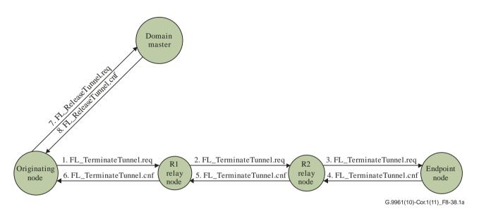
Figure 8-38.1a – Normal tunnel termination
