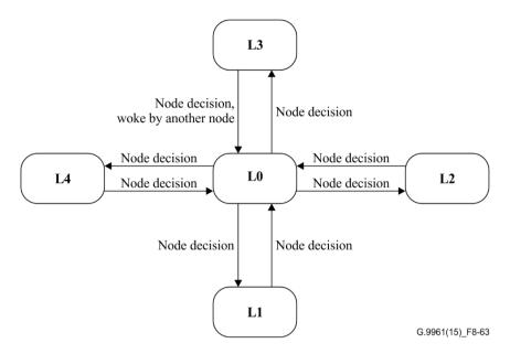
Figure 8-63 – Allowed transitions for node power saving modes
