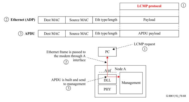
Figure 8-68 – Example of encapsulation of LCMP messages into ITU-T G.hn in-band management messages
