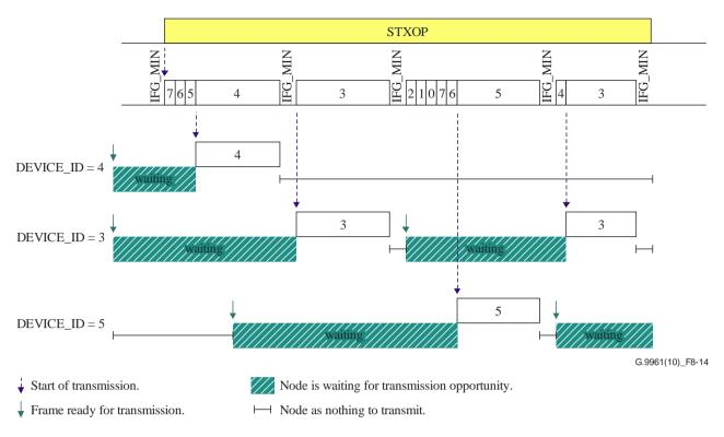
Figure 8-14 – Sequential TS assignment rule example
