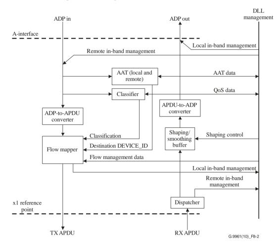
Figure 8-2 – Functional model of APC
