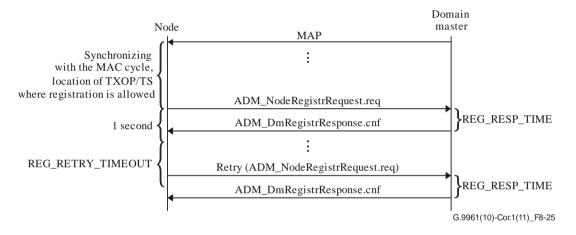
Figure 8-25 – Protocol diagram describing node registration
