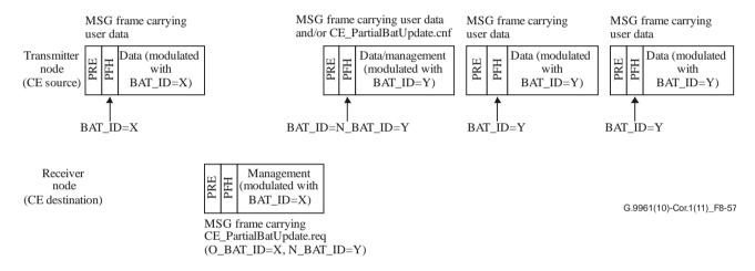
Figure 8-57 – Example of partial BAT update using management message
