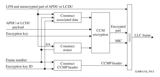
Figure 9-2 – Functional diagram of CCMP encryption
