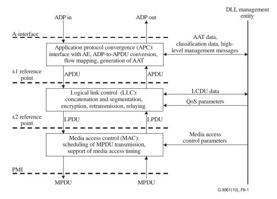
Figure 8-1 – Functional model of the DLL
