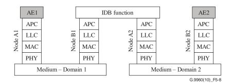
Figure 5-8 – Protocol stack of inter-domain communication
