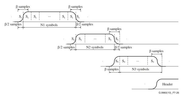
Figure 7-26 – Preamble time-domain generation
