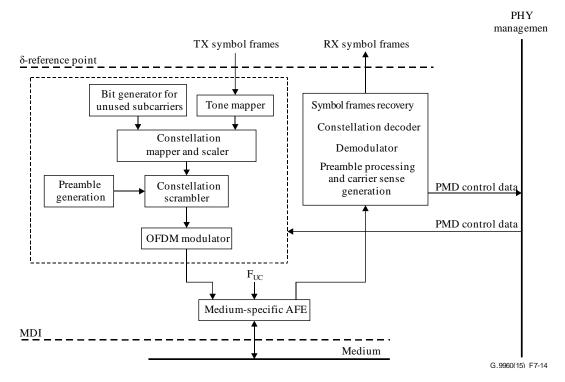
Figure 7-14 – Functional model of the PMD
