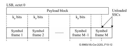
Figure 10-12 – Payload segmentation
