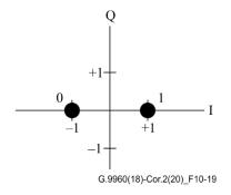
Figure 10-19 – Constellation shape and mapping for *b* = 1
