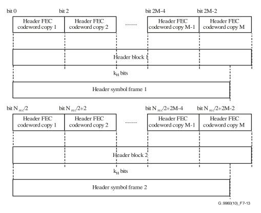
**Figure 7-13 – Header segmentation**
