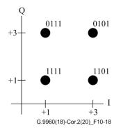
Figure 10-18 – Constellation and mapping for b = 4 (first quadrant)
