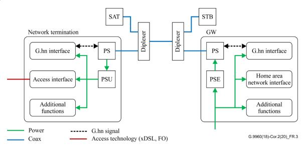
Figure R.3 – Reference architecture – G.hn service coexistence with satellite
