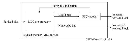
Figure 10-8.1 – Functional diagram of the MLC Payload Encoder
