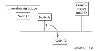
Figure 5-2 – Domain operating in peer-to-peer mode (PM)
