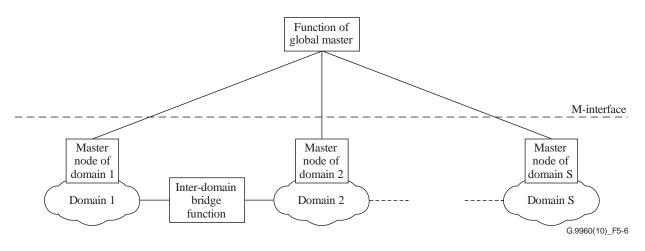
Figure 5-6 – Functional model of GM
