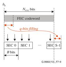
Figure 7-9 – Mapping of an FEC codeword on to sections
