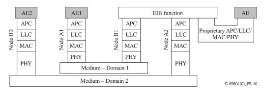
Figure 5-10 – Protocol stack of inter-domain communication
