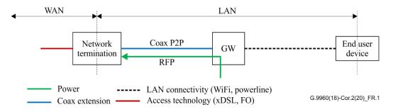
Figure R.1 – Reference model for a RPF installation
