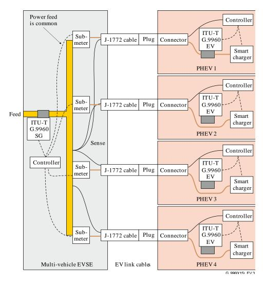
Figure V.3 – EVSE attached to four EVs
