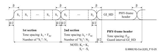
**Figure 10-25 – Preamble waveform**
