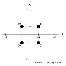
Figure 10-17 – Constellation and mapping for b = 2
