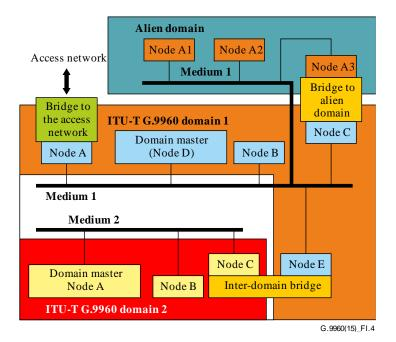
Figure I.4 – Example of an ITU-T G.9960 domain sharing a medium with an alien domain
