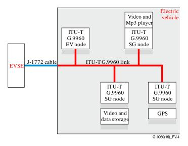
Figure V.4 – Example of multiple nodes within an EV
