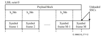
Figure 7-12 – Payload segmentation
