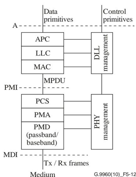
**Figure 5-12 – Functional model of a home network transceiver**
