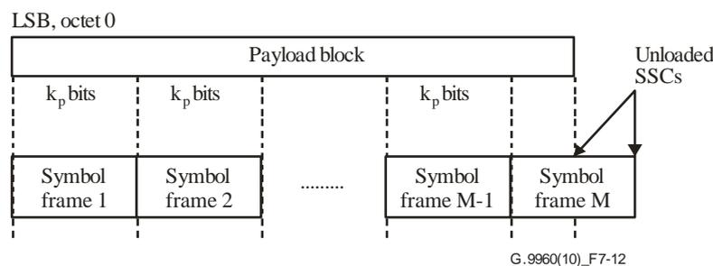
**Figure 7-12 – Payload segmentation**
