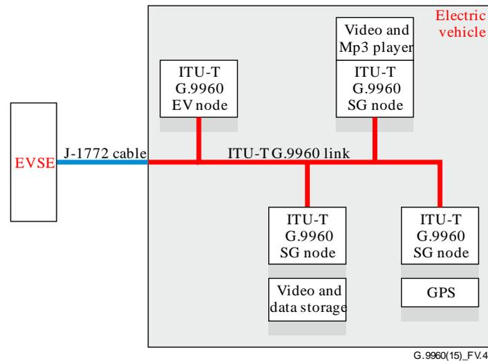
**Figure V.4 – Example of multiple nodes within an EV**
