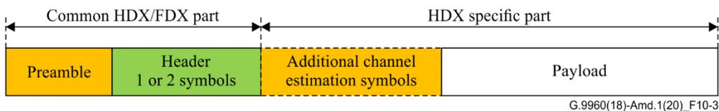
**Figure 10-3 – Format of an HDX PHY frame**
