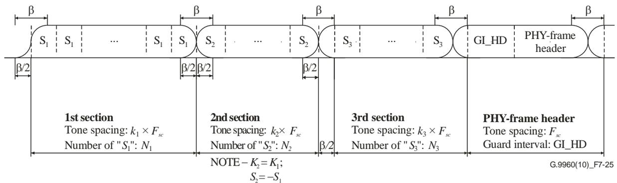
**Figure 7-25 – Preamble waveform**
