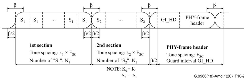
**Figure 10-25 – Preamble waveform**
