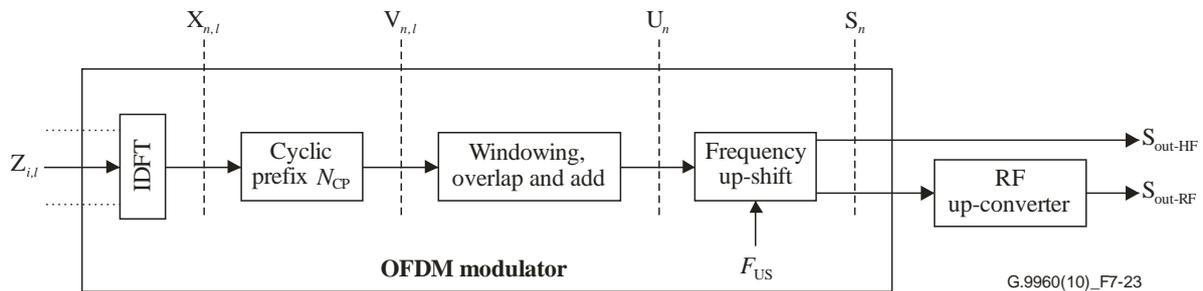
**Figure 7-23 – Functional model of the OFDM modulator**
