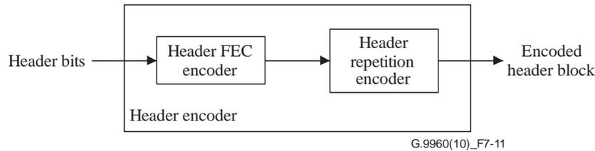
**Figure 7-11 – Functional diagram of the header encoder**
