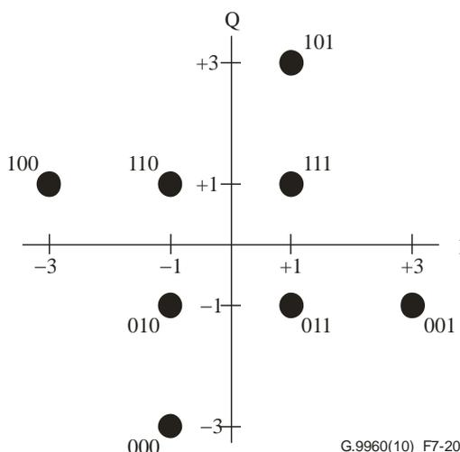
**Figure 7-20 – Constellation and mapping for  $b = 3$**
