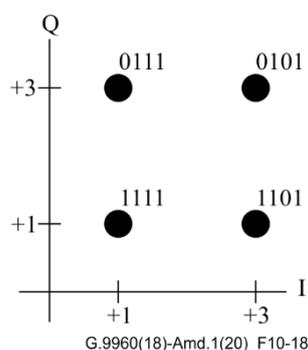
**Figure 10-18 – Constellation and mapping for  $b = 4$  (first quadrant)**
