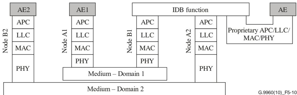
**Figure 5-10 – Protocol stack of inter-domain communication**
