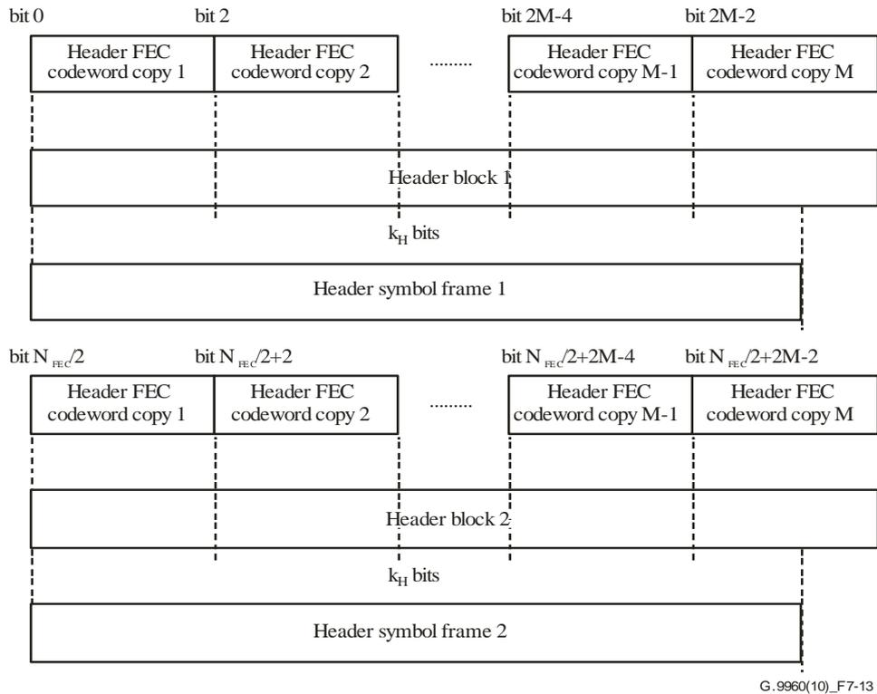
**Figure 7-13 – Header segmentation**
