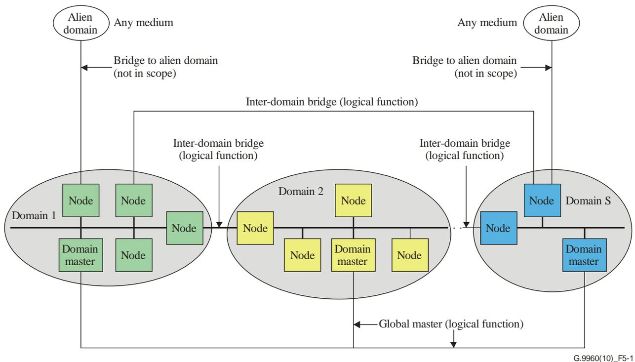
**Figure 5-1 – Home network architecture reference model**
