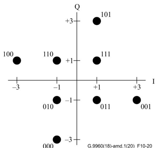
**Figure 10-20 – Constellation and mapping for  $b = 3$**
