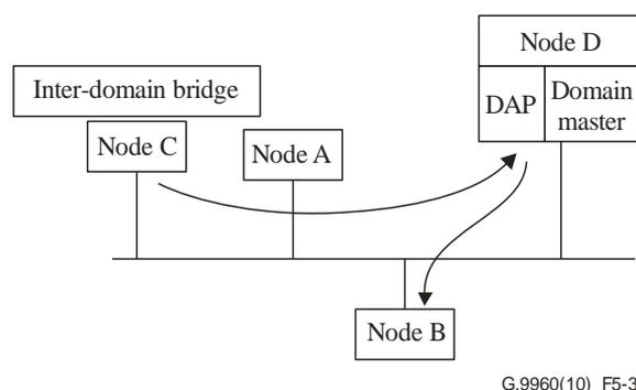
**Figure 5-3 – Domain operating in centralized mode (CM)**
