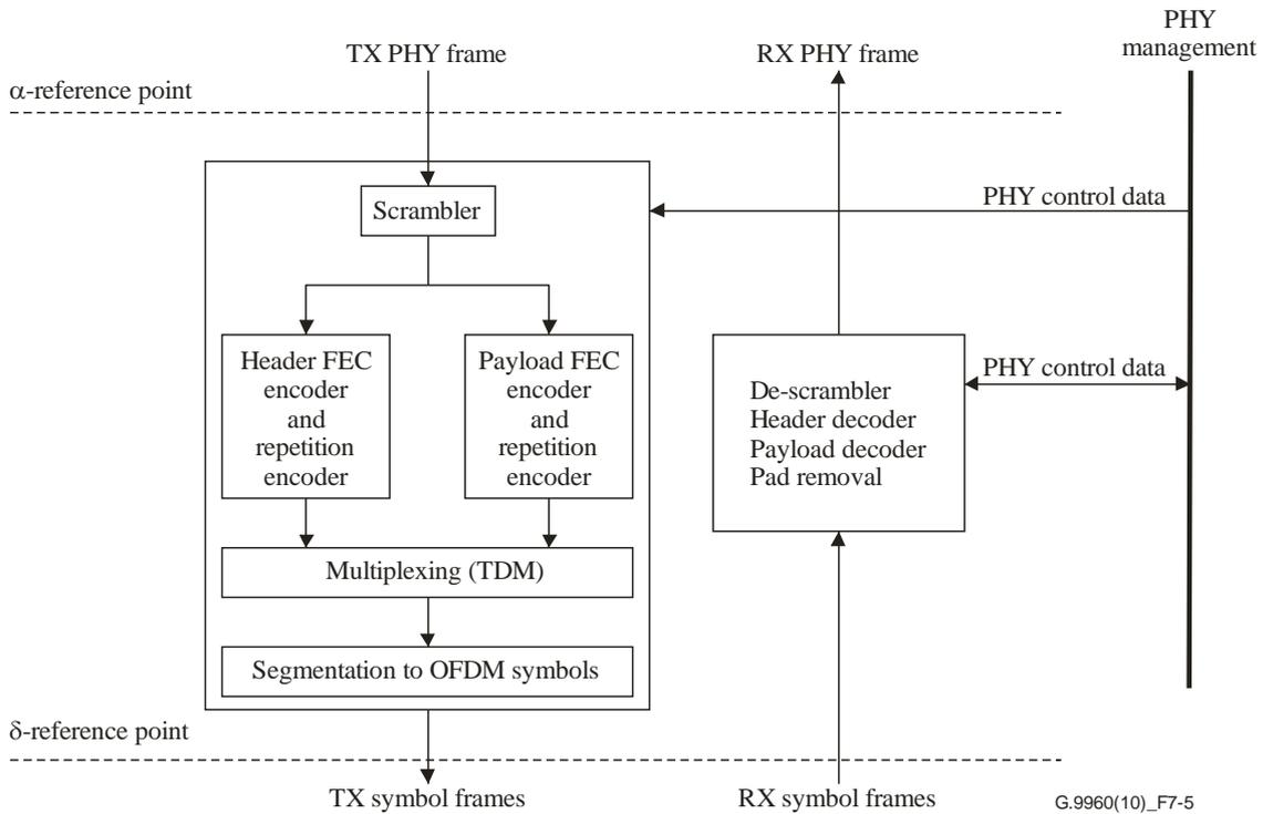
**Figure 7-5 – Functional model of PMA sublayer**
