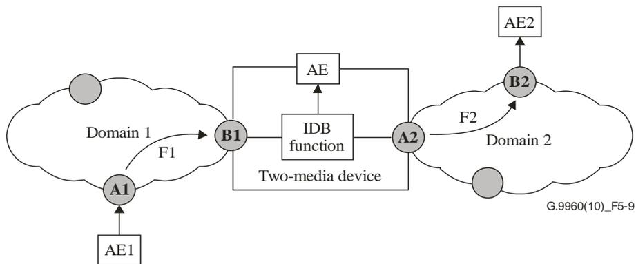
**Figure 5-9 – Example of communication with a two-media (domain) device**
