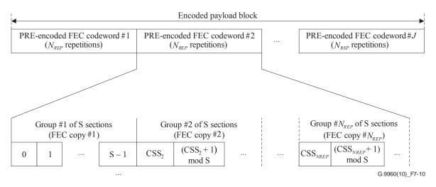
Figure 7-10 – The format of the encoded payload block (payload consists of *J* FEC codewords)
