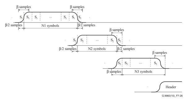
Figure 7-26 – Preamble time-domain generation
