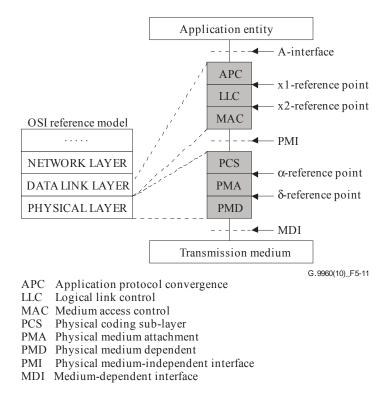
Figure 5-11 – Protocol reference model of a home network transceiver
