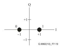
Figure 7-19 – Constellation shape and mapping for b = 1
