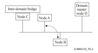
Figure 5-2 – Domain operating in peer-to-peer mode (PM)
