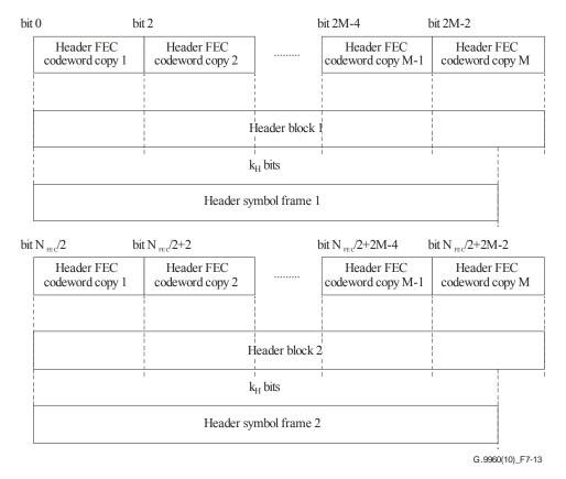
Figure 7-13 – Header segmentation
