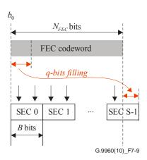
Figure 7-9 – Mapping of a FEC codeword onto sections
