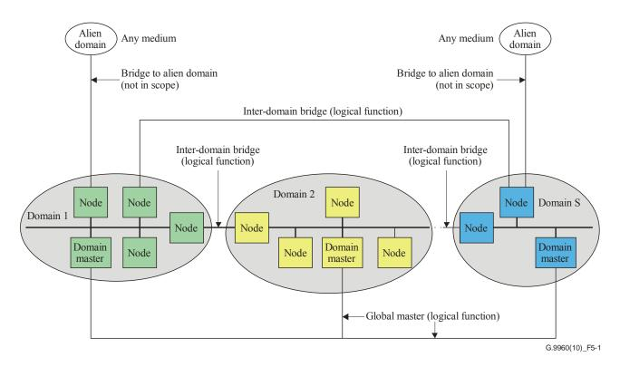
Figure 5-1 – Home network architecture reference model
