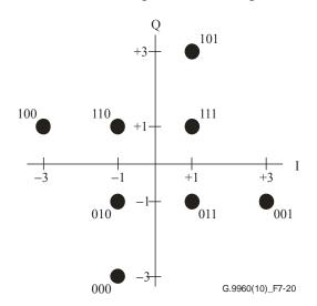
Figure 7-20 – Constellation and mapping for b = 3
