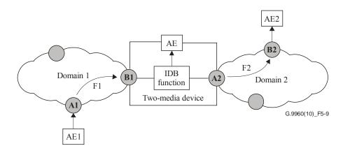
Figure 5-9 – Example of communication with a two-media (domain) device
