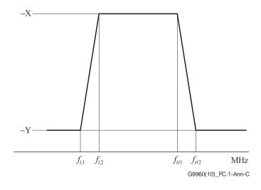
Figure C.1 – Limit PSD mask over RF coax for transceivers used between 770 MHz and 1032 MHz
