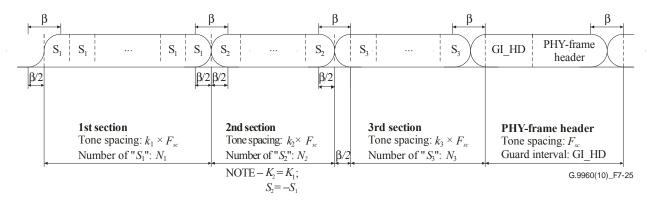
Figure 7-25 – Preamble waveform
