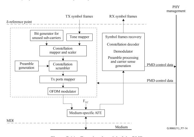
Figure 7-14 – Functional model of the PMD
