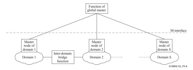
Figure 5-6 – Functional model of GM
