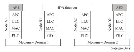
Figure 5-8 – Protocol stack of inter-domain communication
