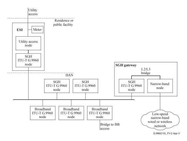
Figure IV.2 – Interconnection between ITU-T G.9960 SGH and a SG narrow-band network
