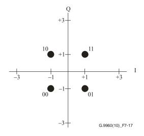
Figure 7-17 – Constellation and mapping for b = 2
