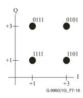
Figure 7-18 – Constellation and mapping for b = 4 (first quadrant)
