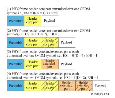
Figure 7-4 – Possible cases of PHY-frame header transmissions
