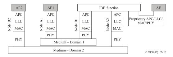
Figure 5-10 – Protocol stack of inter-domain communication
