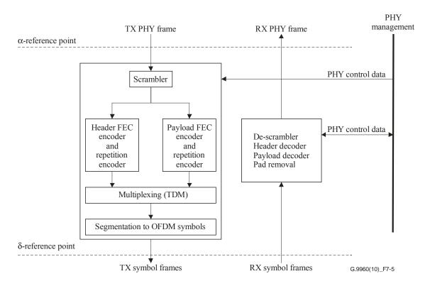
Figure 7-5 – Functional model of PMA sub-layer
