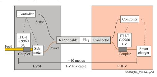
Figure V.2 – Simple EVSE to EV link using a J-1772 cable
