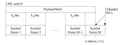
Figure 7-12 – Payload segmentation
