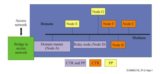
Figure I.2 – Example of a home network containing a single domain operating in UM (using a combination of P2P and REL)
