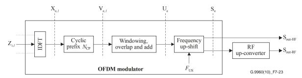
Figure 7-23 – Functional model of the OFDM modulator
