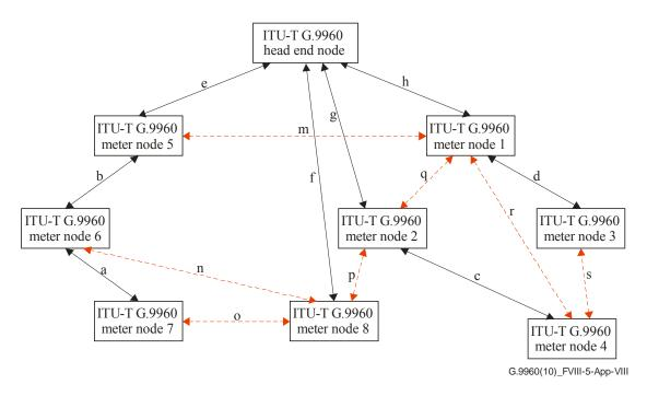
Figure VI.5 – ITU-T G.9960 mesh network ability
