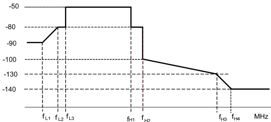
**Figure 7-27/G.9960 – Limit PSD mask for baseband transmission over power lines for 50 MHz-PB bandplan (Amateur radio-band notches are not shown)**
