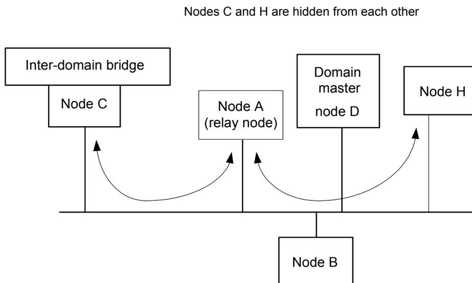
**Figure 5-4/G.9960 – A domain operating in unified mode (UM) containing hidden nodes**
