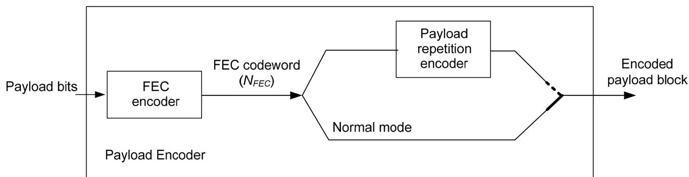
**Figure 7-7/G.9960 – Functional diagram of the Payload Encoder (set to Normal mode)**
