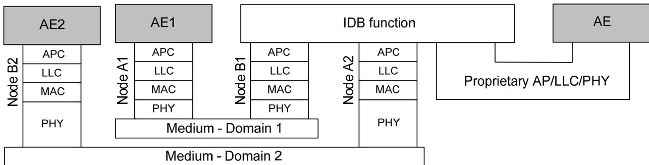
**Figure 5-10/G.9960 – Protocol stack of inter-domain communication**
