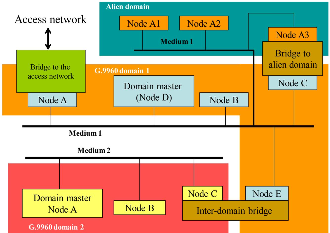
**Figure I-4/G.9960 – Example of a G.9960 sharing a medium with an alien domain**
