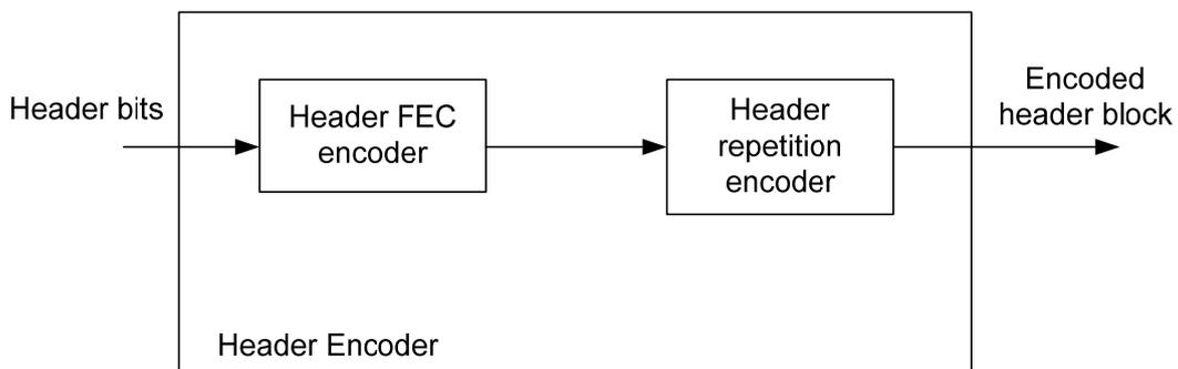
**Figure 7-10/G.9960 – Functional diagram of the Header Encoder**
