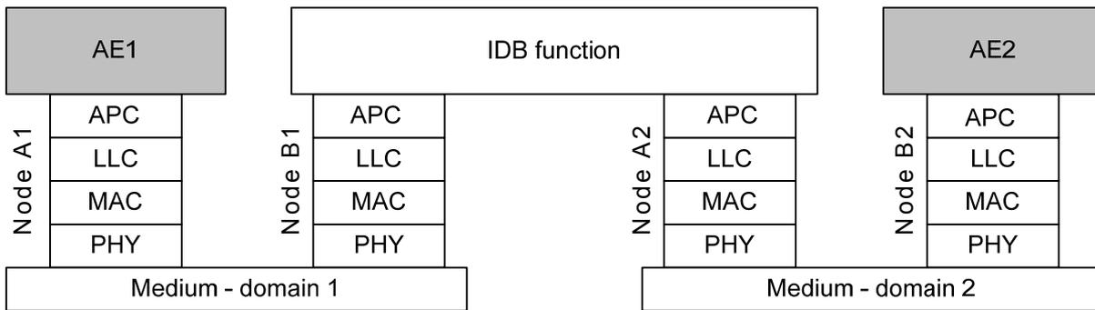
**Figure 5-8/G.9960 – Protocol stack of inter-domain communication**
