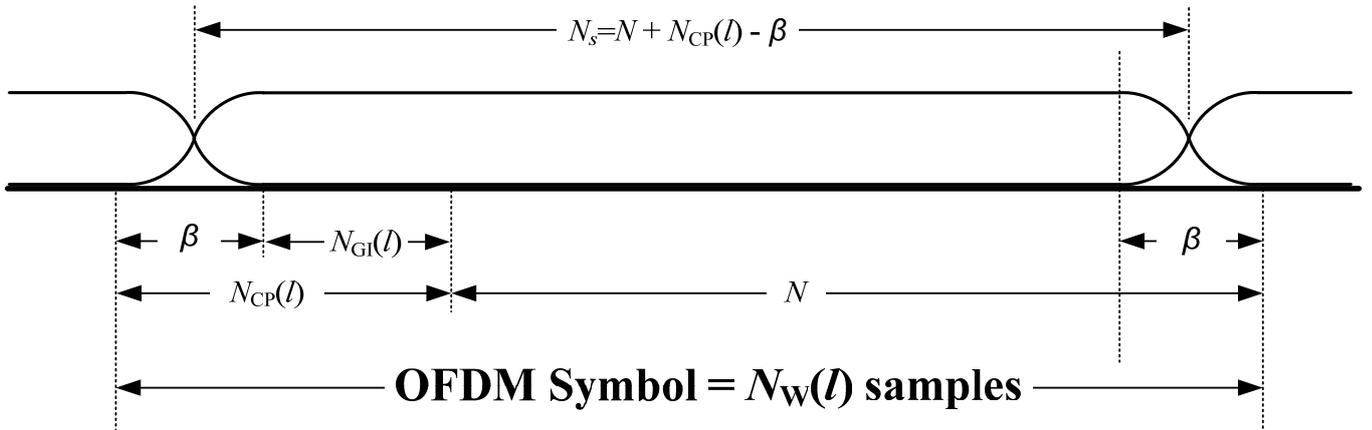
**Figure 7-22/G.9960 – Structure of an OFDM symbol with cyclic extension and overlapped windowing**
