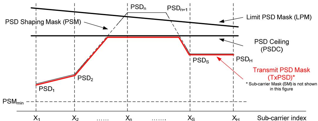
**Figure 7-25/G.9960 – Construction of PSM**
