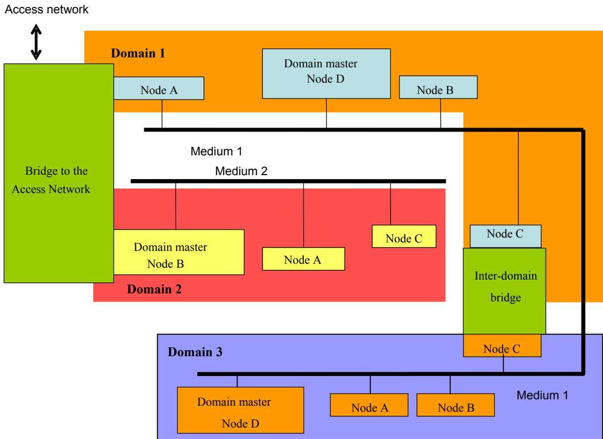
**Figure I-3/G.9960 – Example of a home network comprising three domains**
