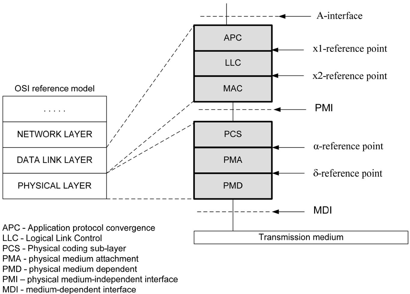
**Figure 5-11/G.9960 – Protocol reference model of a home network transceiver**
