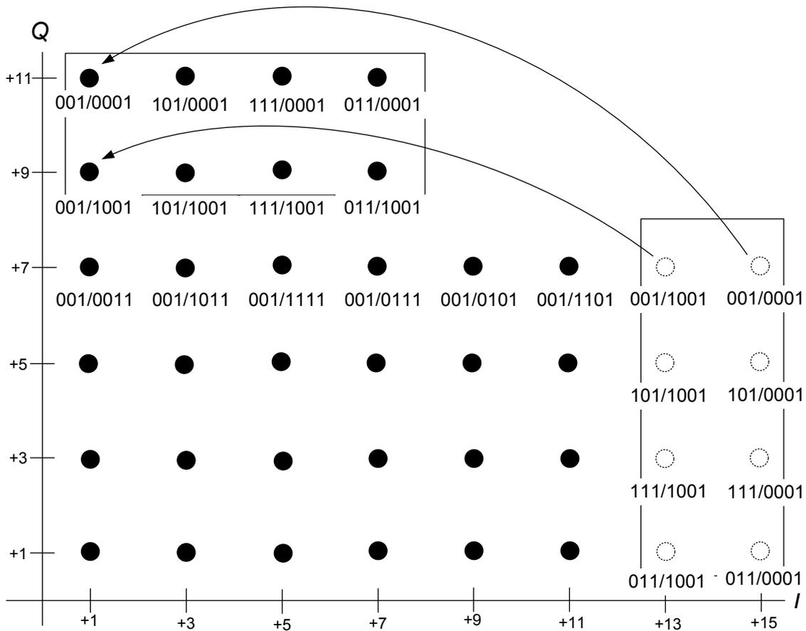
**Figure 7-19/G.9960 - Transformation of rectangular constellation into cross-shaped constellation for  $b = 7$  (first quadrant)**
