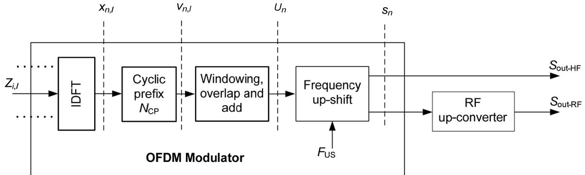
**Figure 7-21/G.9960 – Functional model of the OFDM modulator**
