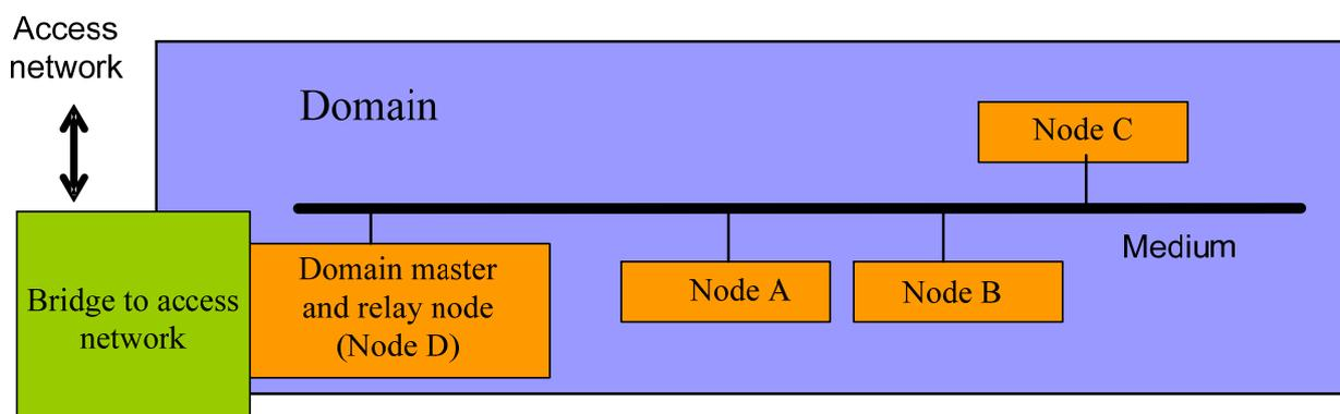
**Figure I-1/G.9960 – Example of a home network containing a single domain**
