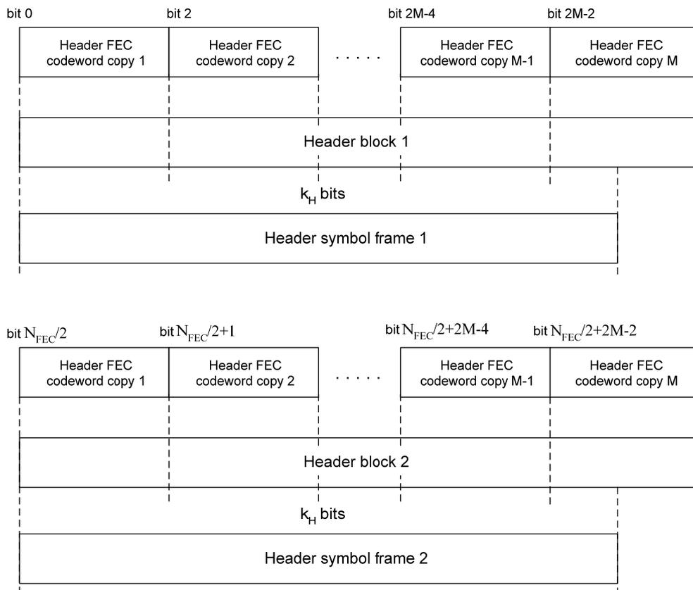
**Figure 7-12/G.9960 – Header segmentation**
