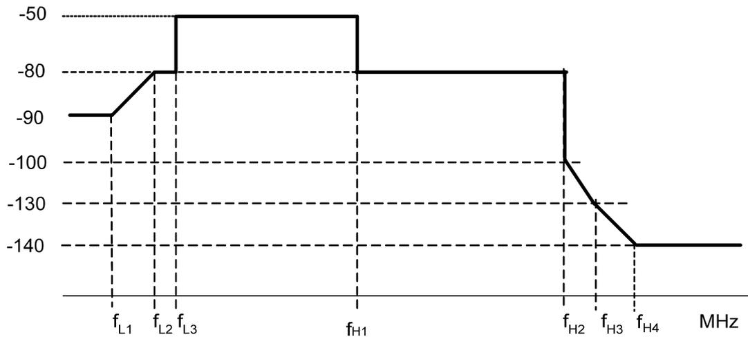
**Figure 7-28/G.9960 – Limit PSD mask for baseband transmission over power lines for 100 MHz-PB bandplan (Amateur radio-band notches are not shown)**
