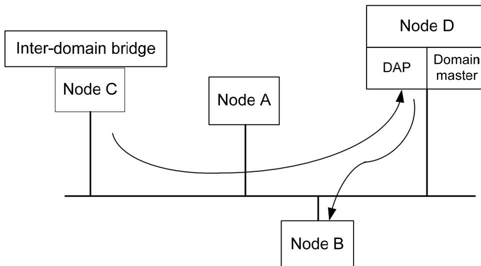
**Figure 5-3/G.9960 – Domain operating in centralized mode (CM)**
