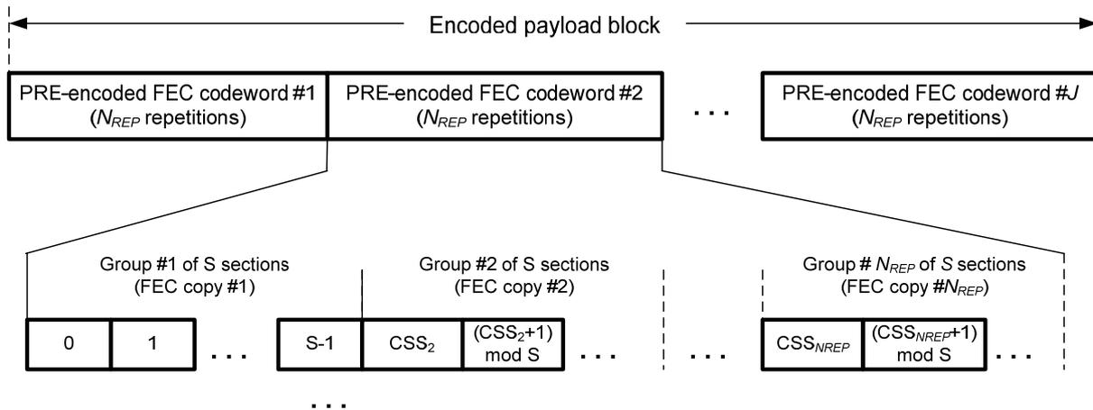
**Figure 7-9/G.9960 – The format of the encoded payload block (payload consists of  $J$  FEC codewords)**
