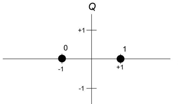
**Figure 7-17/G.9960 - Constellation shape and mapping for  $b = 1$**
