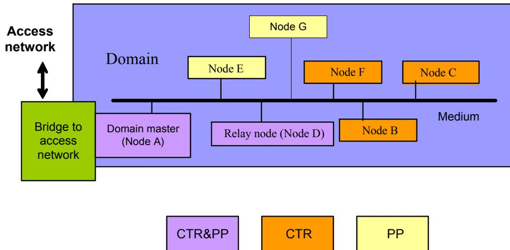
**Figure I-2/G.9960 – Example of a home network containing a single domain operating in UM (using a combination of P2P& REL)**
