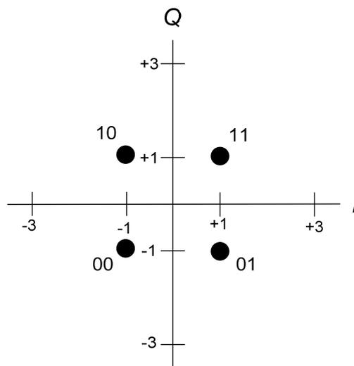
Figure 7-15/G.9960 - Constellation and mapping for  $b = 2$
