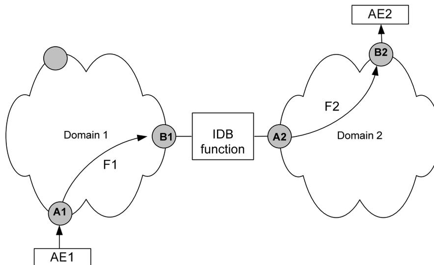
**Figure 5-7/G.9960 – Communication path between nodes of two different domains**
