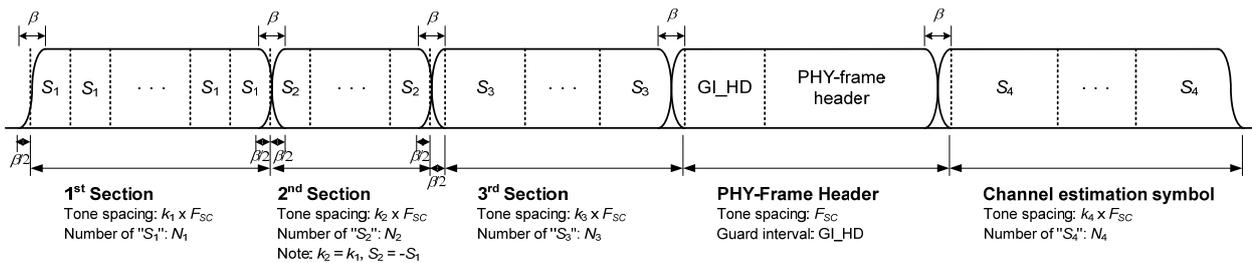
**Figure 7-23/G.9960 – Preamble waveform**
