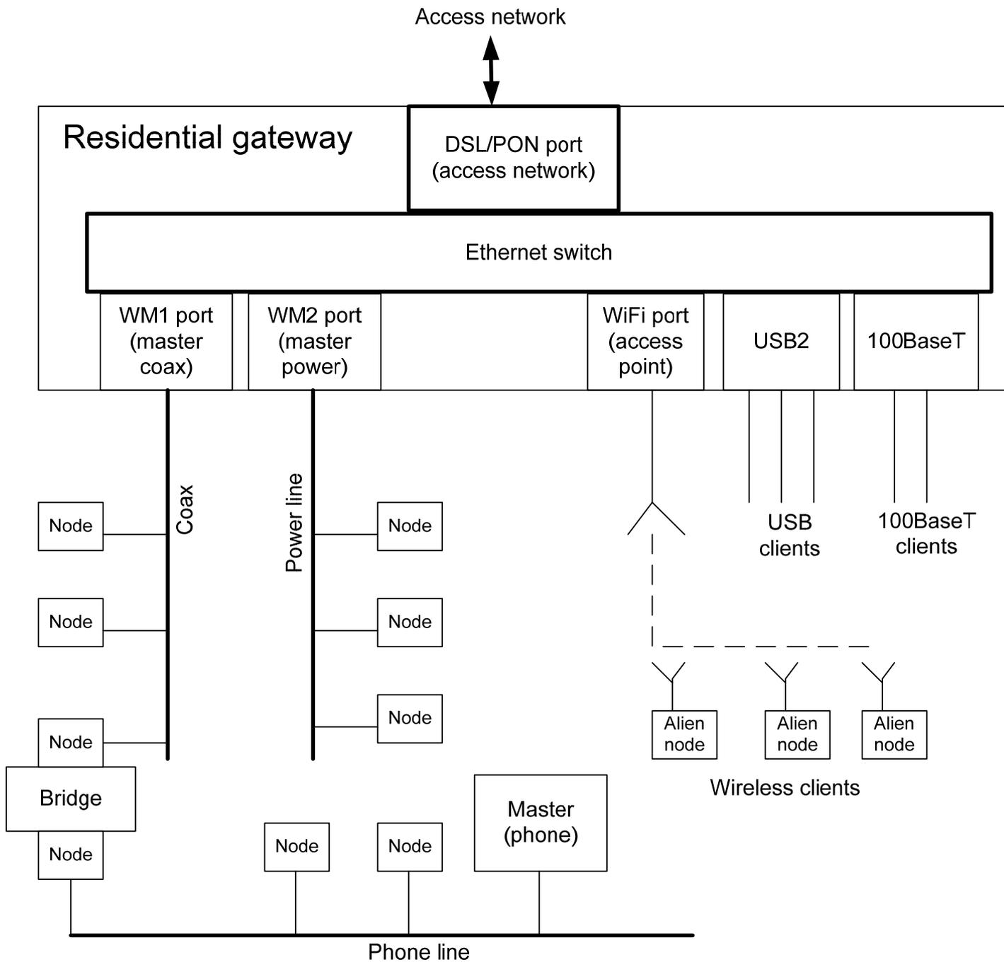
**Figure I-5/G.9960 – Example of a home network supporting residential broadband access**
