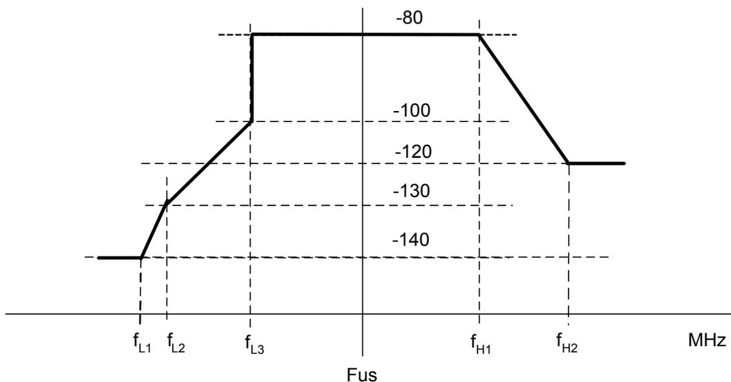
**Figure 7-29/G.9960 – Limit PSD mask for passband transmission over power lines**
