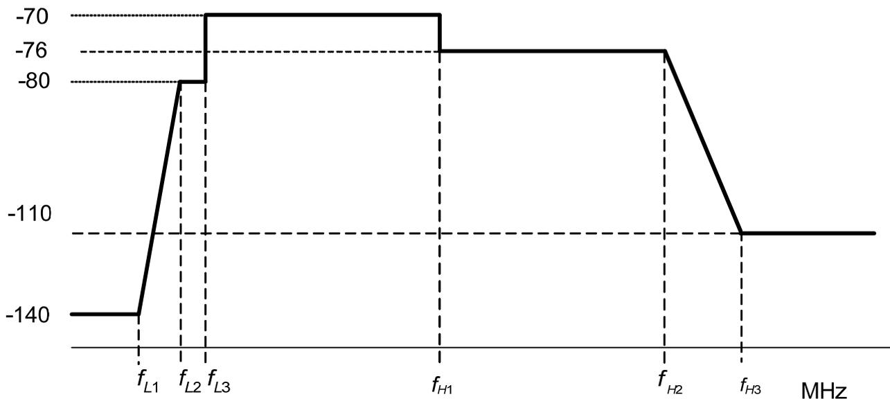
**Figure 7-26/G.9960 – Limit PSD mask for transmission over phone lines
