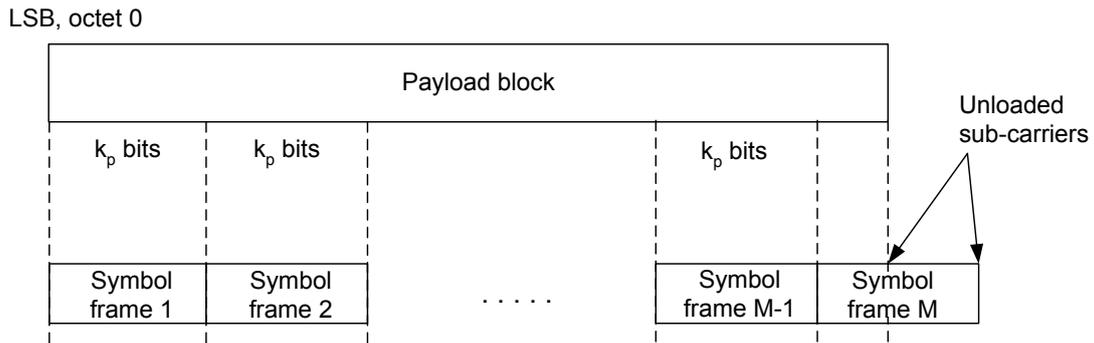
**Figure 7-11/G.9960 – Payload segmentation**
