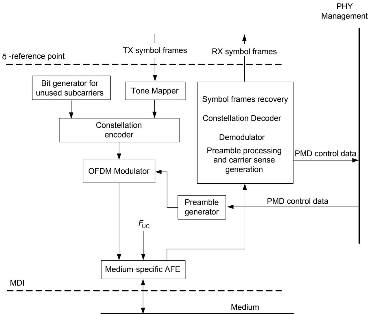
**Figure 7-13/G.9960 – Functional model of the PMD**
