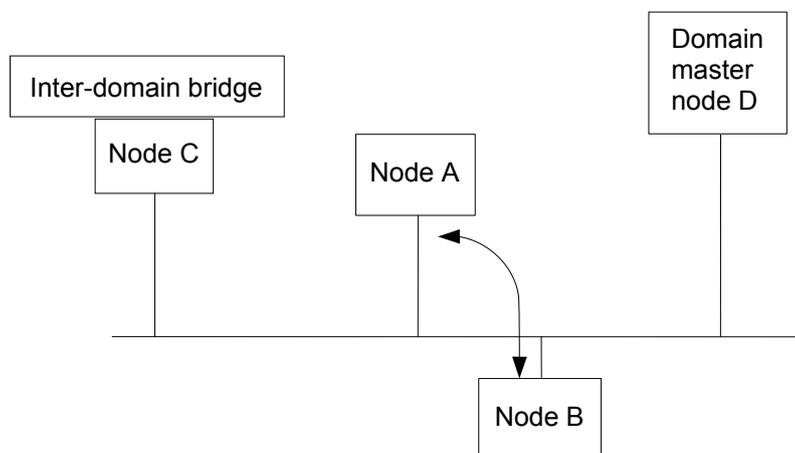
**Figure 5-2/G.9960 – Domain operating in peer-to-peer mode (PM)**
