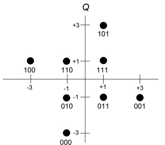
**Figure 7-18/G.9960 - Constellation and mapping for  $b = 3$**
