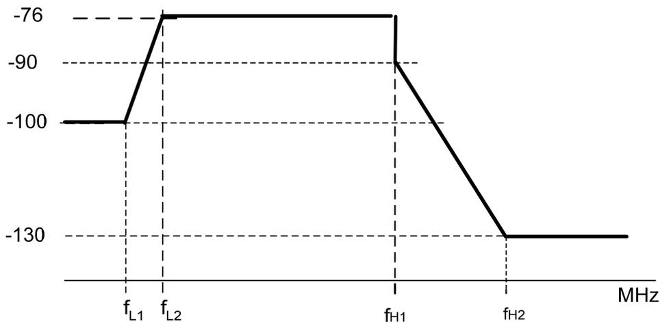
**Figure 7-31/G.9960 - Limit PSD mask of baseband coax**
