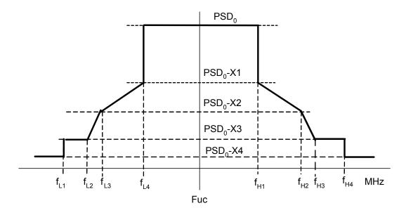
Figure 7-30/G.9960 - Limit PSD mask of a single channel for RF transmission over coax
