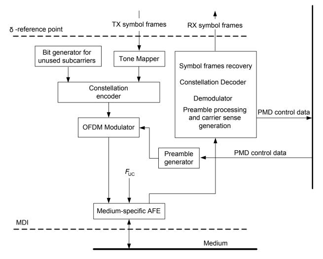
Figure 7-13/G.9960 – Functional model of the PMD
