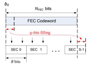
Figure 7-8/G.9960 – Mapping of a FEC codeword onto sections
