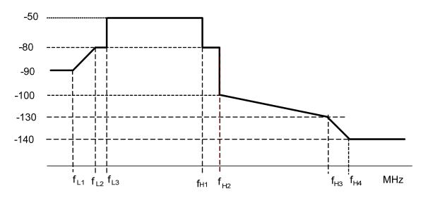
Figure 7-27/G.9960 – Limit PSD mask for baseband transmission over power lines for 50 MHz-PB bandplan (Amateur radio-band notches are not shown)
