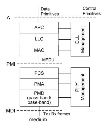
Figure 5-12/G.9960 - Functional model of a home network transceiver
