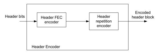
Figure 7-10/G.9960 – Functional diagram of the Header Encoder
