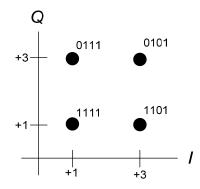
Figure 7-16/G.9960 – Constellation and mapping for b = 4 (first quadrant)
