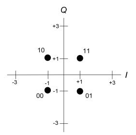
Figure 7-15/G.9960 - Constellation and mapping for b = 2
