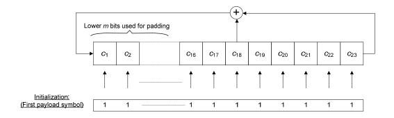
Figure 7-14/G.9960 – LFSR for modulation of unloaded and partially loaded sub-carriers
