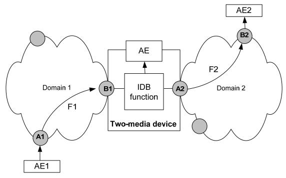
Figure 5-9/G.9960 – Example of communication with a two-media (domain) device
