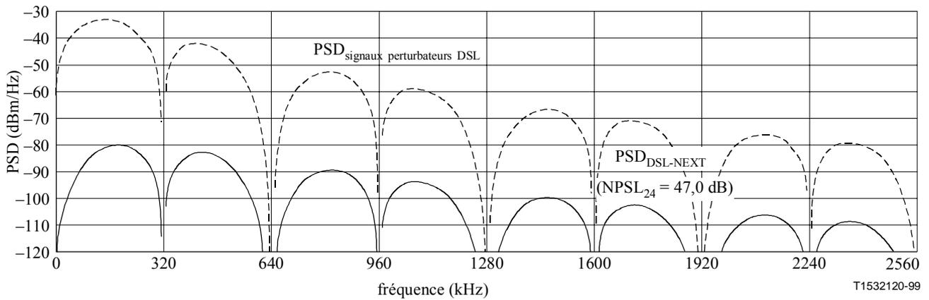
Figure 29/G.996.1 – Paradiaphonie DSL RNIS-TCM due to 24 interfering signals
