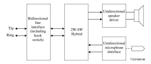
Figure 7/G.996.1 – Typical telephone signal flow
