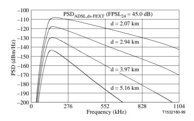
Figure 35/G.996.1 – 24-disturber G.992.1 (FDM) downstream FEXT
