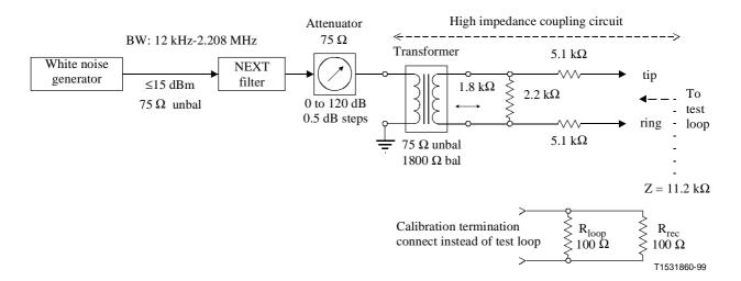
Figure 3/G.996.1 – High impedance crosstalk injection circuit
