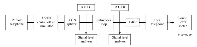
Figure 8/G.996.1 – Test configuration
