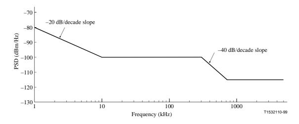
Figure 28/G.996.1 – Single-sided noise power spectral density into 100  $\Omega$  for ETSI B
