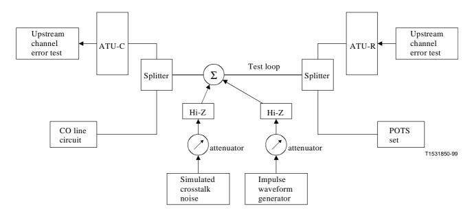
Figure 2/G.996.1 – Laboratory test set-up for measuring performance margins for the upsteam channel with splitters
