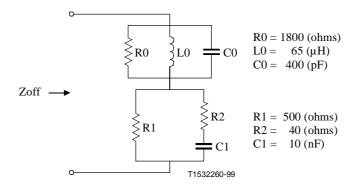
Figure 43/G.996.1 – Off-hook impedance for off-hook phone model #1
