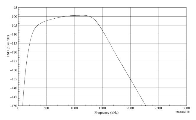
Figure 22/G.996.1 – 10-disturber upstream G.992.1 NEXT into the downstream
