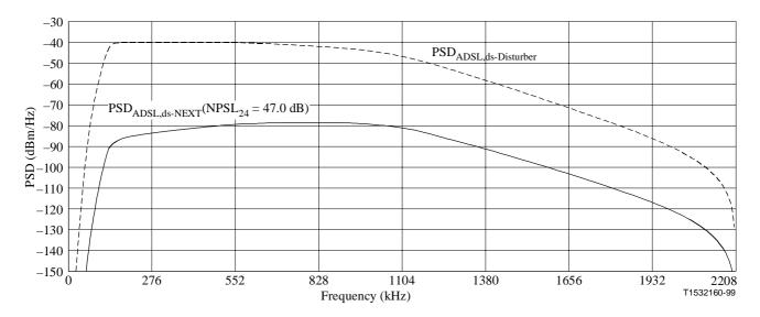
Figure 33/G.996.1 – 24-disturber G.992.1 (FDM) downstream NEXT
