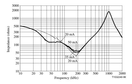
Figure 41/G.996.1 – Measured off-hook impedance for off-hook phone #1
