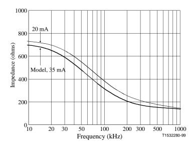
Figure 45/G.996.1 – Off-hook impedance of measured telephone compared with model
