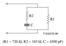
Figure 44/G.996.1 – Simple model of an off-hook telephone
