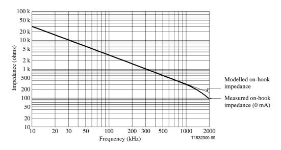
Figure 47/G.996.1 – Measured and modelled on-hook impedance
