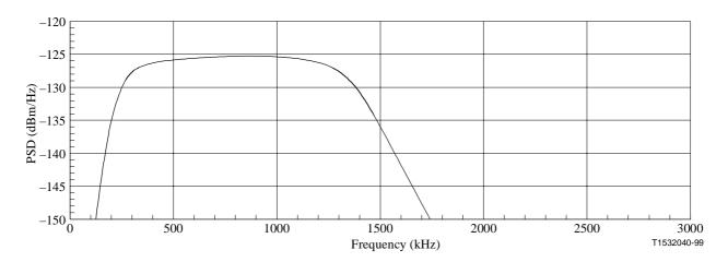
Figure 21/G.996.1 – Theoretical 10-disturber upstream G.992.1 FEXT on C loop #6
