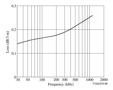
Figure 48/G.996.1 – Insertion loss characteristics of 3 m connecting cord
