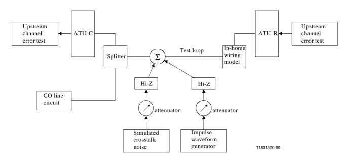
Figure 6/G.996.1 – Laboratory test set-up for measuring performance margins for the upstream channel without a splitter at the ATU-R
