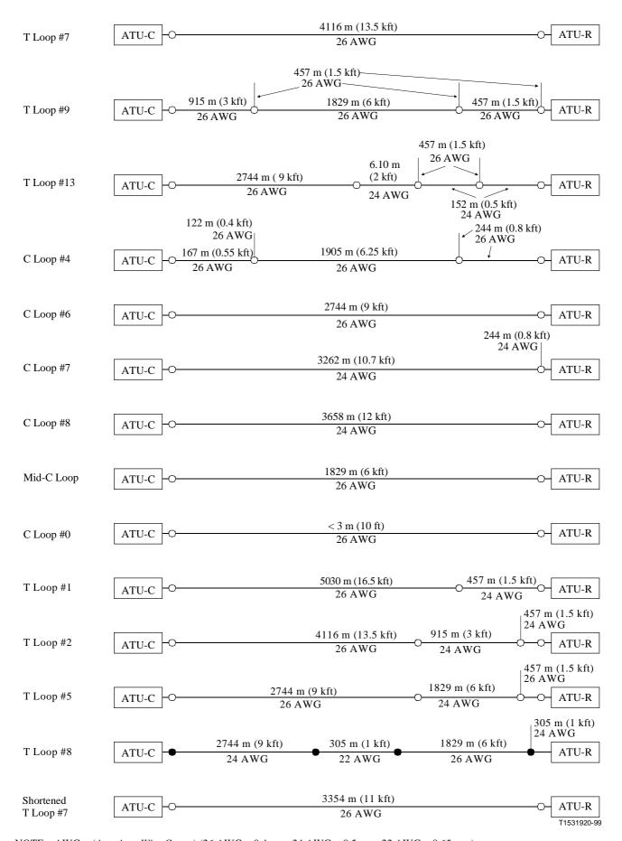
$NOTE-AWG=(\textit{American Wire Gauge}) \ (26 \ AWG=0.4 \ mm, 24 \ AWG=0.5 \ mm, 22 \ AWG=0.65 \ mm).$
