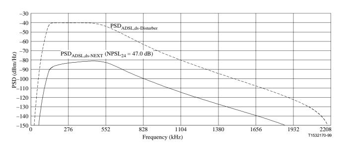
Figure 34/G.996.1 – 24-disturber G.992.2 (FDM) downstream NEXT
