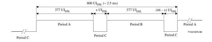
Period A: DSL NEXT noise injection Period B: DSL FEXT noise injection Period C: DSL XT noise non-injection  $6 \le x \le 40$ NOTE -1 UI<sub>DSL</sub> =  $3.125 \mu s$
