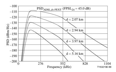
Figure 36/G.996.1 – 24-disturber G.992.2 (FDM) downstream FEXT
