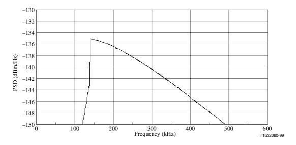
Figure 23/G.996.1 – 49-disturber downstream G.992.2 FEXT on T loop #7
