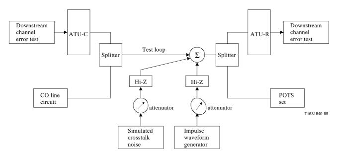
Figure 1/G.996.1 – Laboratory test set-up for measuring performance margins for the downstream channel with splitters
