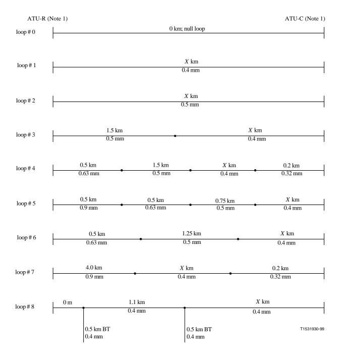
NOTE 1 – These test loops are shown with the ATU-Rs on the left; this is the European convention, which is in contrast to Figure 9, where the ATU-Rs are on the right.
