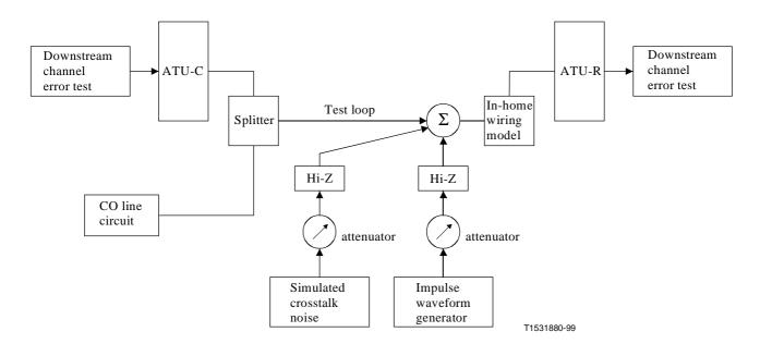
Figure 5/G.996.1 – Laboratory test set-up for measuring performance margins for the downstream channel without a splitter at the ATU-R
