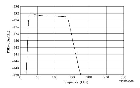
Figure 25/G.996.1 – Theoretical 49-disturber upstream G.992.2 FEXT on T loop #7
