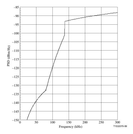
Figure 24/G.996.1 – 49-disturber downstream G.992.2 NEXT into the upstream
